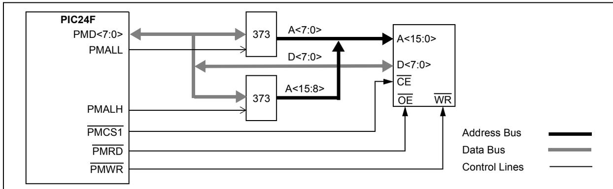
**FIGURE 19-8: EXAMPLE OF A PARTIALLY MULTIPLEXED ADDRESSING APPLICATION**
