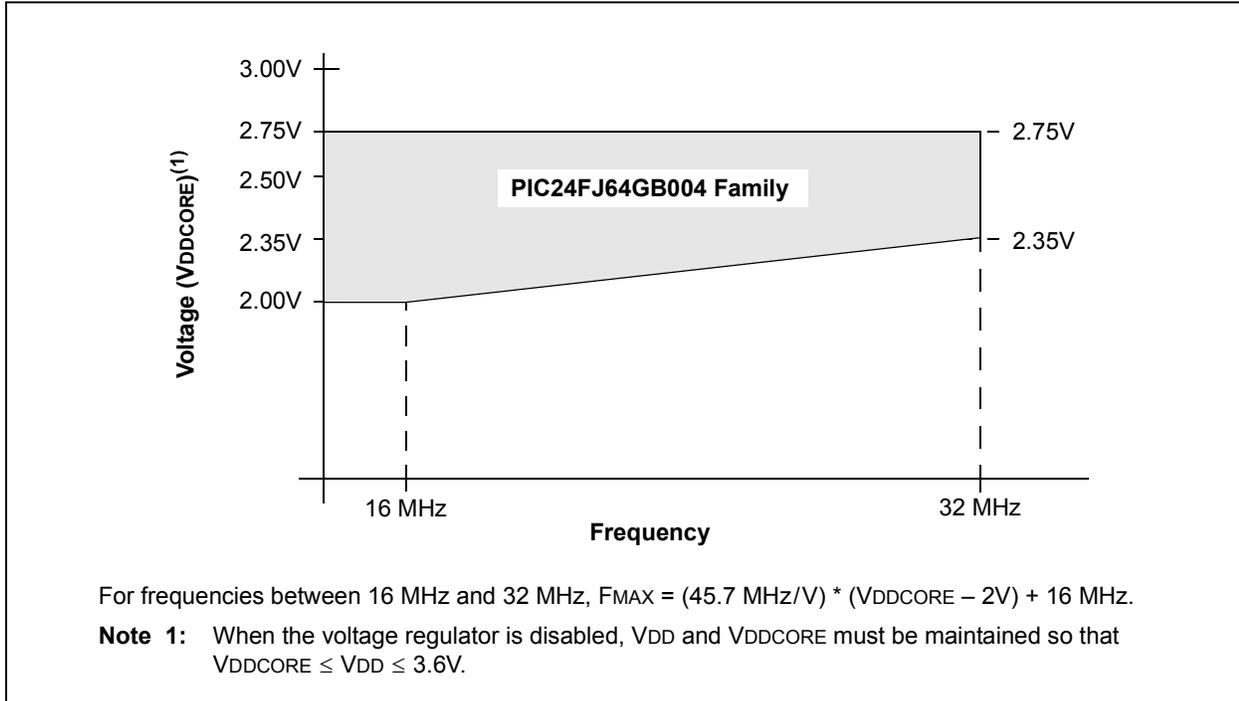
FIGURE 29-2: PIC24FJ64GB004 FAMILY VOLTAGE-FREQUENCY GRAPH (EXTENDED TEMPERATURE)
