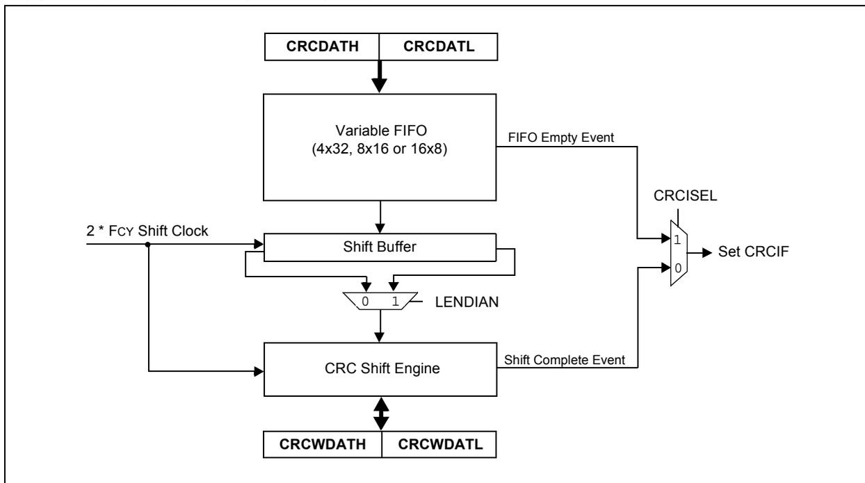
**FIGURE 21-2: CRC SHIFT ENGINE DETAIL**
