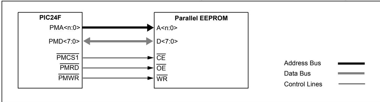
**FIGURE 19-11: PARALLEL EEPROM EXAMPLE (UP TO 11-BIT ADDRESS, 16-BIT DATA)**
