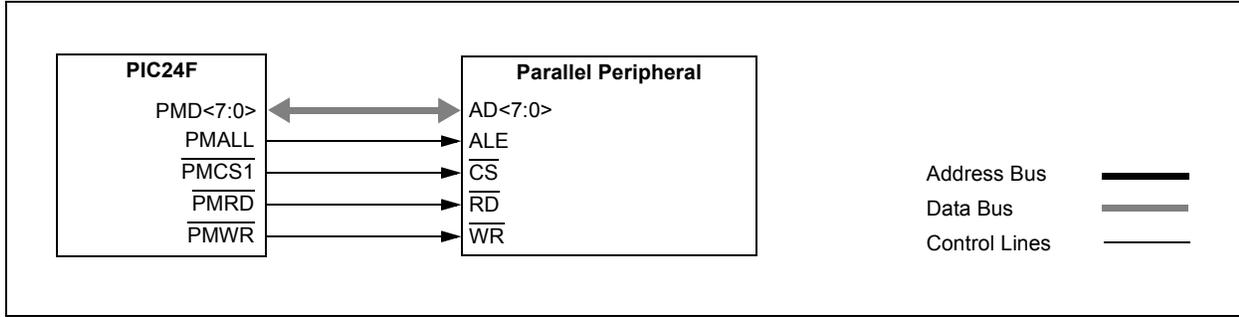
**FIGURE 19-10: PARALLEL EEPROM EXAMPLE (UP TO 11-BIT ADDRESS, 8-BIT DATA)**
