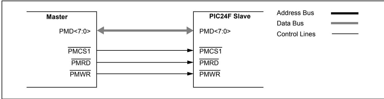
**FIGURE 19-3: ADDRESSABLE PARALLEL SLAVE PORT EXAMPLE**
