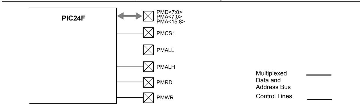
**FIGURE 19-7: EXAMPLE OF A MULTIPLEXED ADDRESSING APPLICATION**
