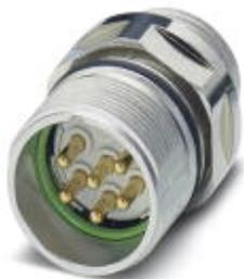
Device connector for front wall, straight, shielded: yes, SPEEDCON locking, M23, No. of pos.: 7, type of contact: Pin, Crimp connection, Axial seal, Central fastening M20 x 1.5, can be positioned via a locking nut
