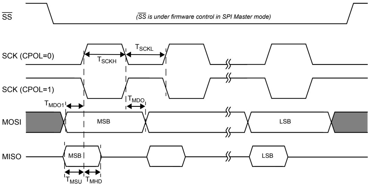
Figure 21-6. SPI Slave Timing, CPHA = 0
