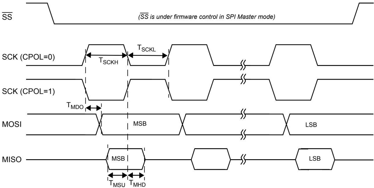
Figure 21-4. SPI Slave Timing, CPHA = 1
