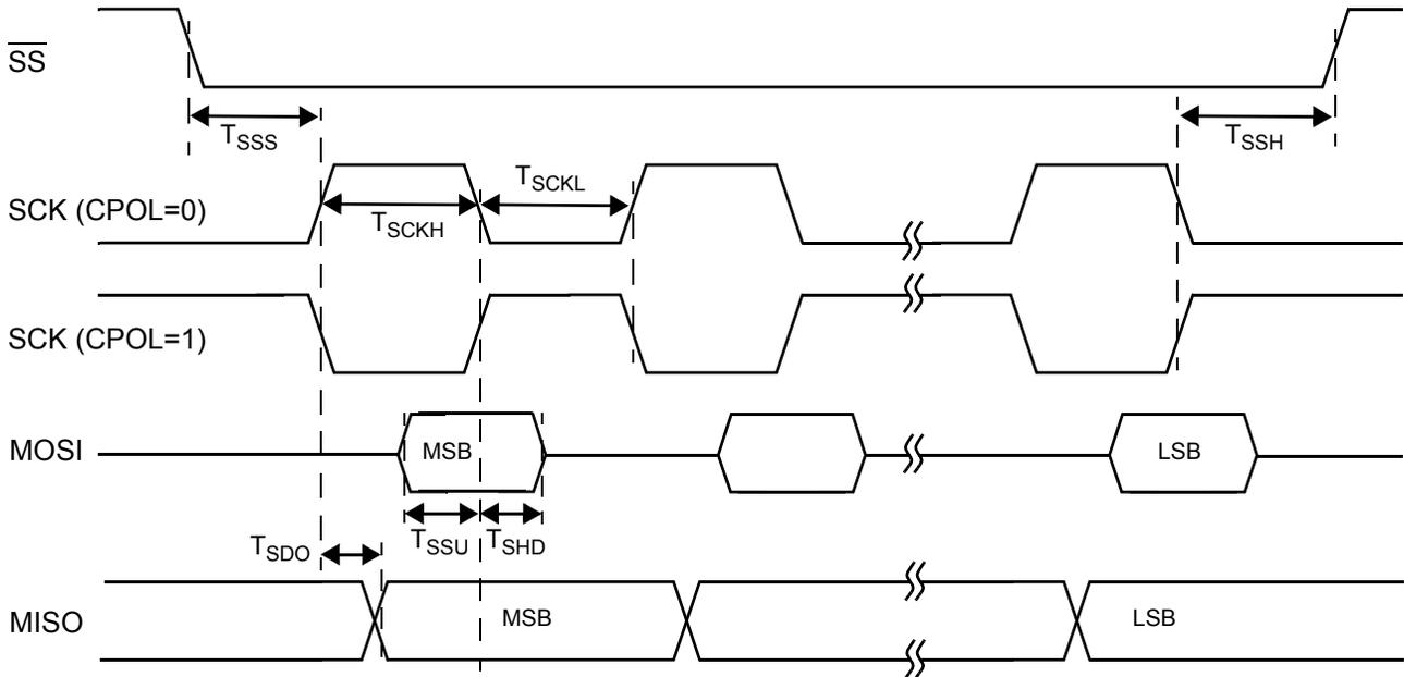
Figure 21-5. SPI Master Timing, CPHA = 0
