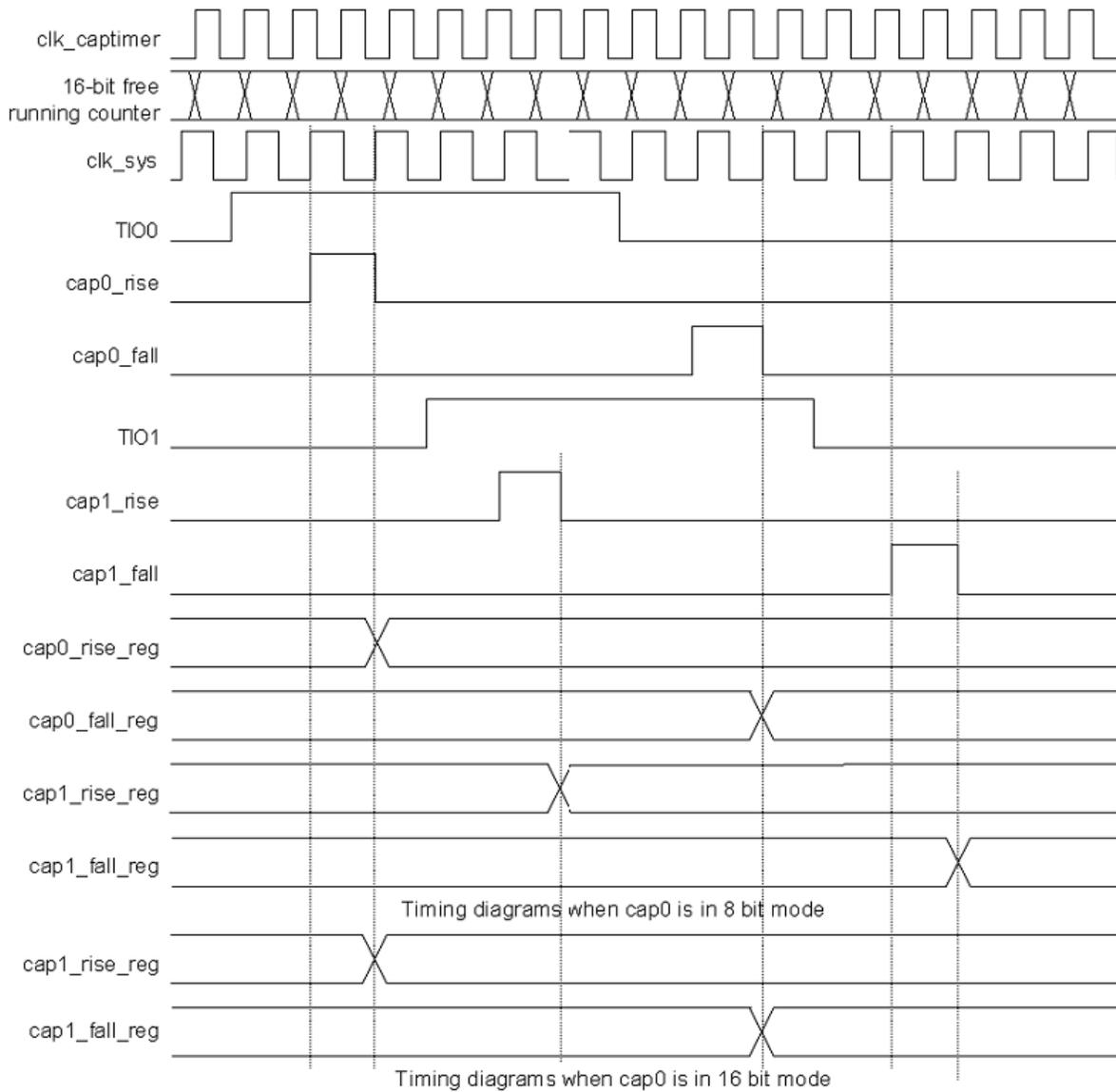
**Figure 19-4. 16-Bit Free-Running Counter Loading Timing Diagram**
