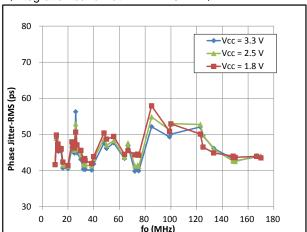
Phase Jitter RMS (Integration bandwidth 1.8 M-20 MHz)
