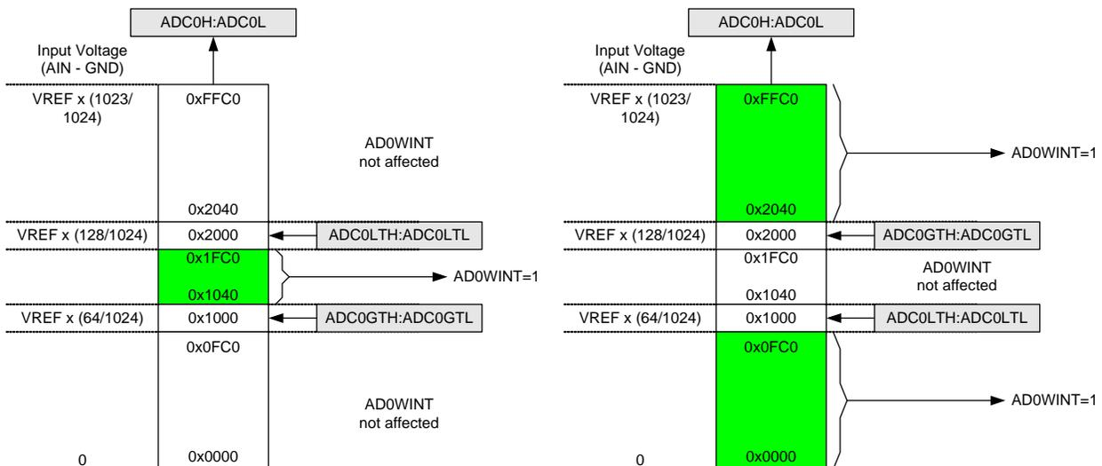
Figure 10.5. ADC Window Compare Example: Left-Justified Data
