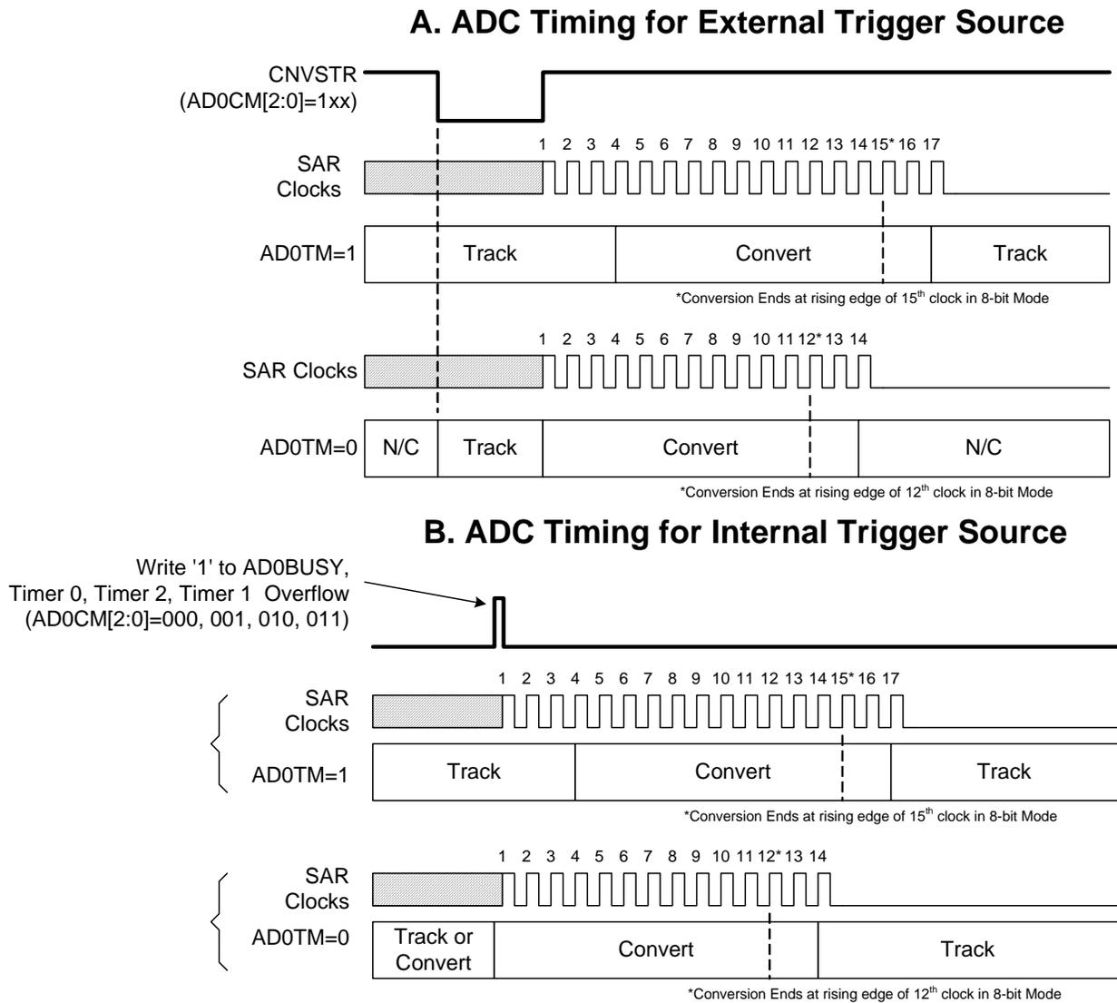
**Figure 10.2. 10-Bit ADC Track and Conversion Example Timing**
