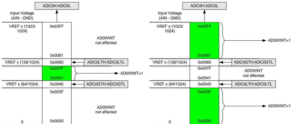
Figure 10.4. ADC Window Compare Example: Right-Justified Data
