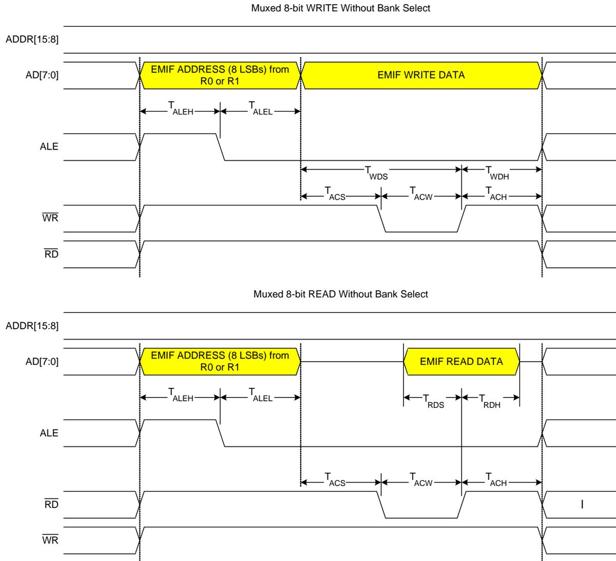
**Figure 18.8. Multiplexed 8-Bit MOVX without Bank Select Timing**
