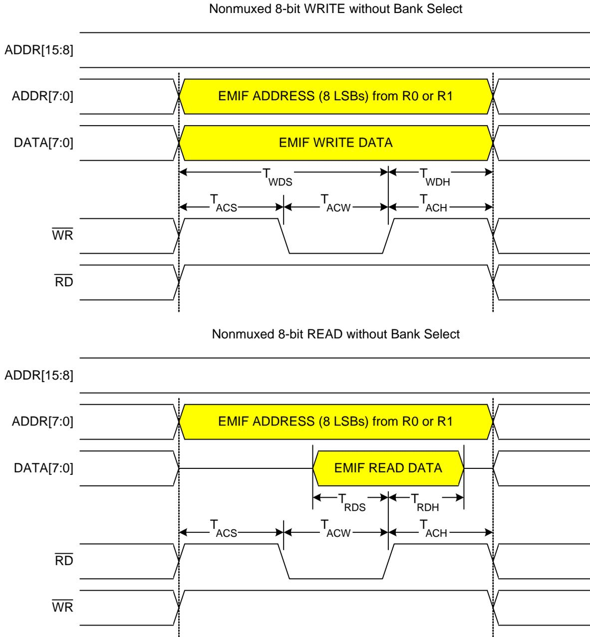
**Figure 18.5. Non-multiplexed 8-bit MOVX without Bank Select Timing**
