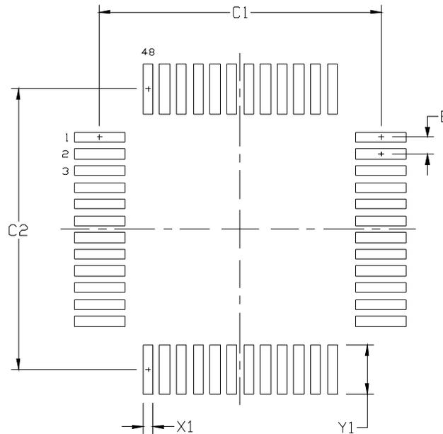
**Figure 5.2. TQFP-48 PCB Land Pattern**
