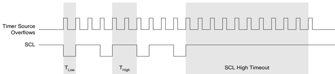
**Figure 30.4. Typical SMBus SCL Generation**
