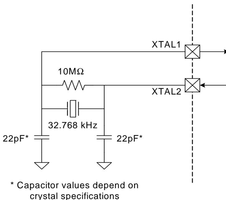
**Figure 27.2. External 32.768 kHz Quartz Crystal Oscillator Connection Diagram**
