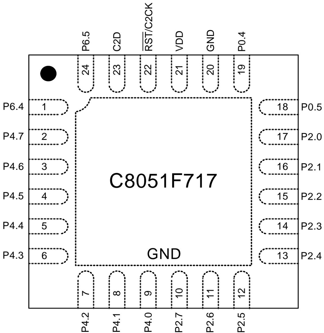
Figure 3.5. C8051F717-GM QFN24 Pinout Diagram (Top View)
