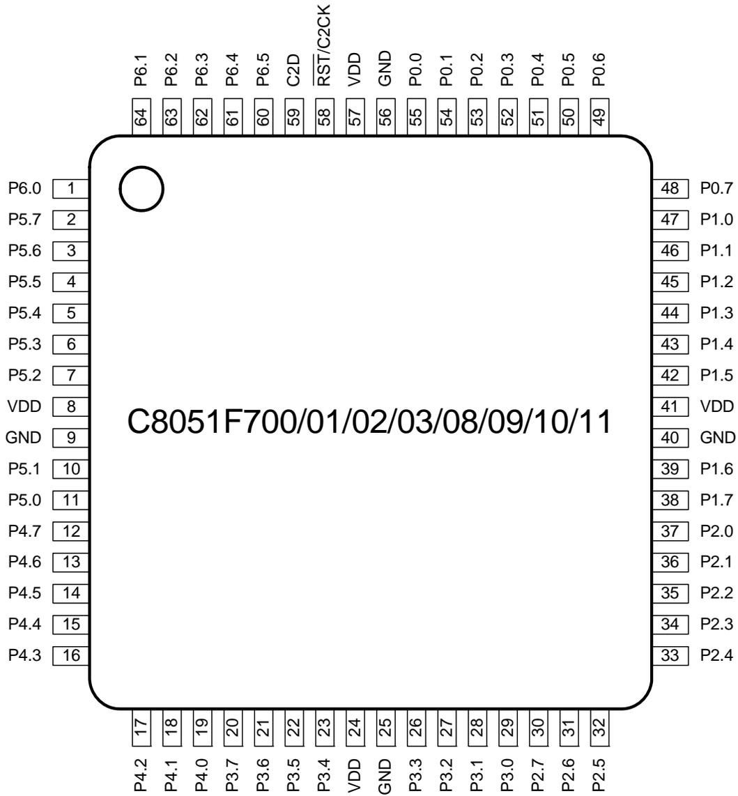
**Figure 3.1. C8051F7xx-GQ TQFP64 Pinout Diagram (Top View)**
