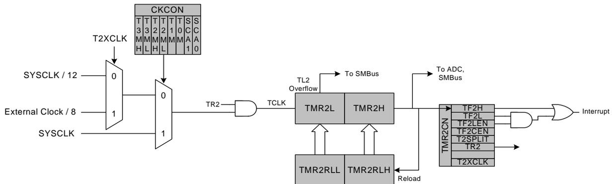
Figure 33.4. Timer 2 16-Bit Mode Block Diagram
