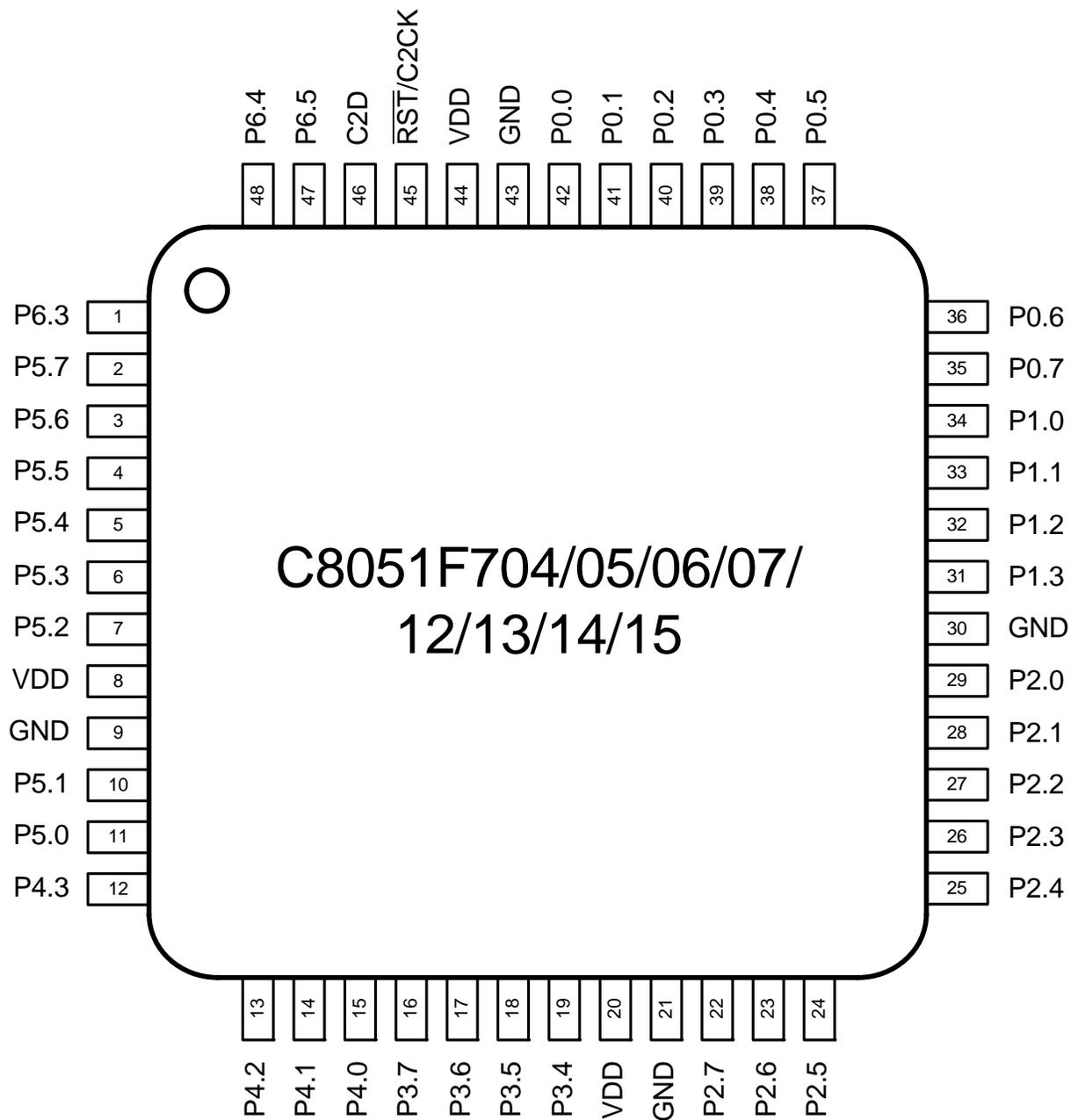
Figure 3.2. C8051F7xx-GQ QFP48 Pinout Diagram (Top View)
