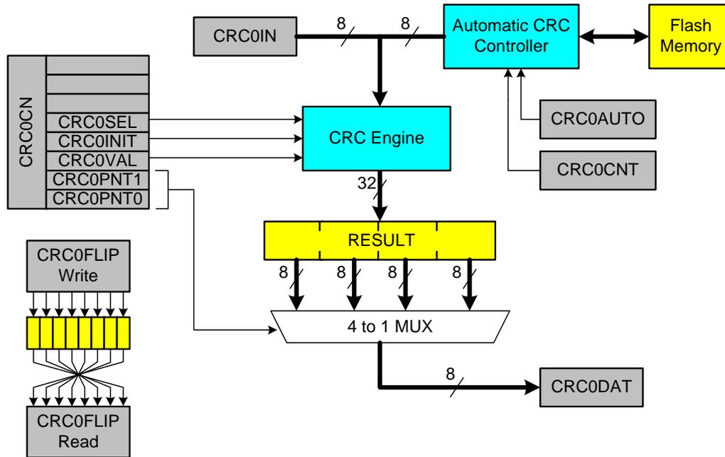
Figure 29.1. CRC0 Block Diagram
