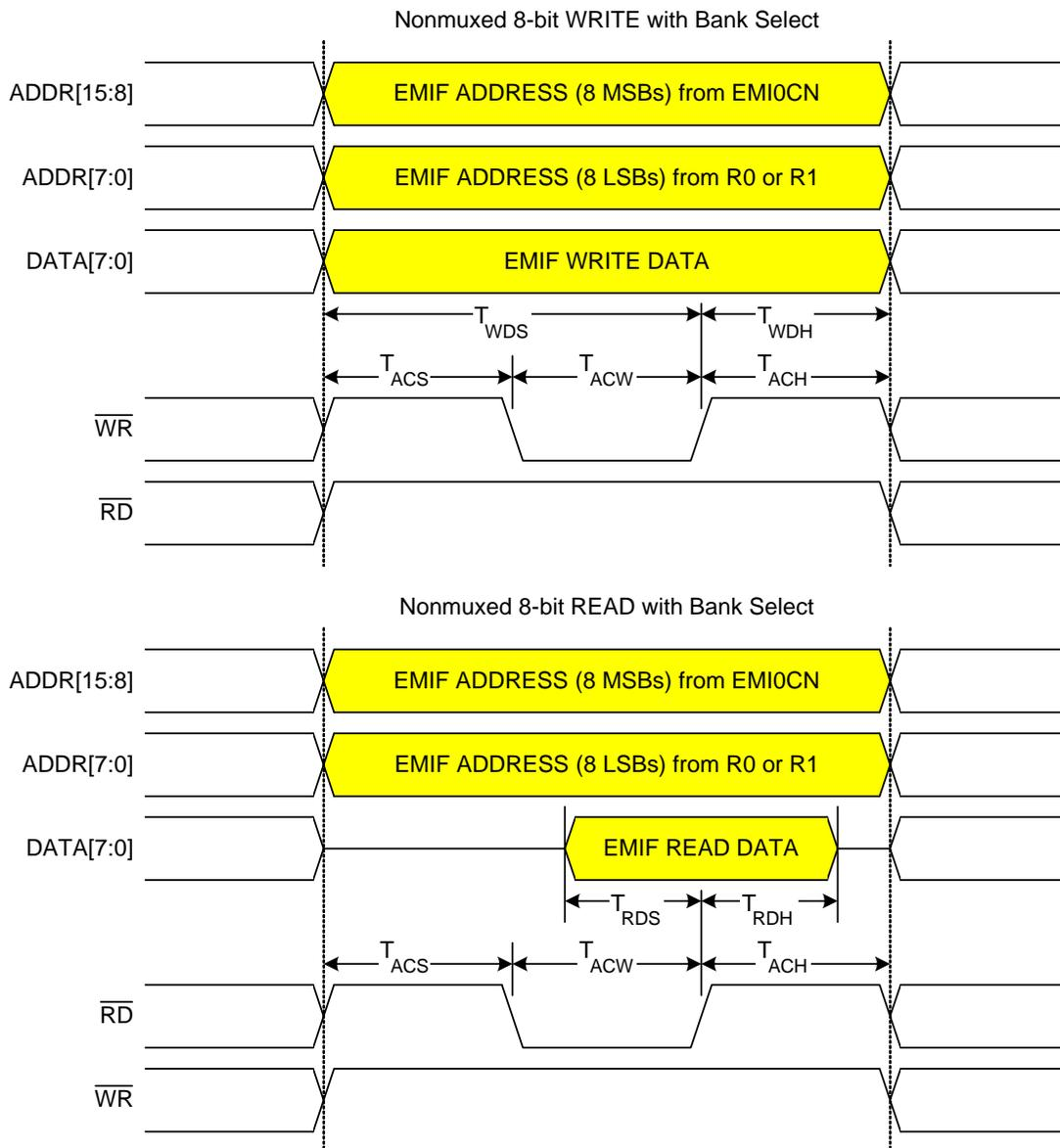
**Figure 18.6. Non-Multiplexed 8-Bit MOVX with Bank Select Timing**
