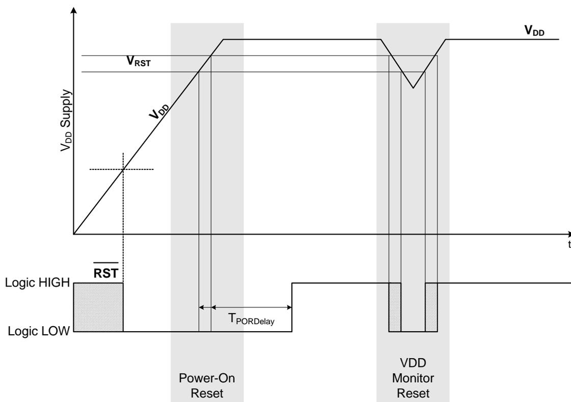
Figure 25.2. Power-On and  $V_{\text{DD}}$  Monitor Reset Timing
