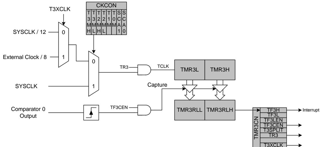
**Figure 33.9. Timer 3 Capture Mode Block Diagram**
