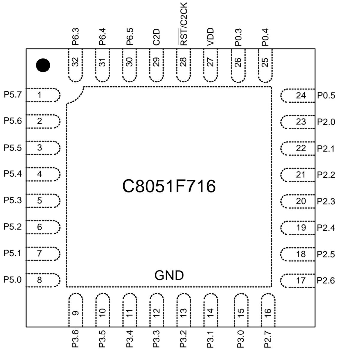
Figure 3.4. C8051F716-GM QFN32 Pinout Diagram (Top View)
