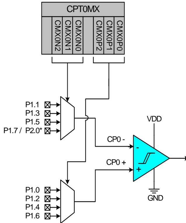
\*P1.7 on 64 and 48-pin devices, P2.0 on 32 and 24-pin devices
