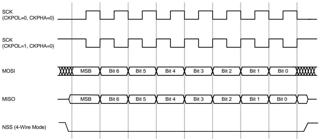
**Figure 31.6. Slave Mode Data/Clock Timing (CKPHA = 0)**
