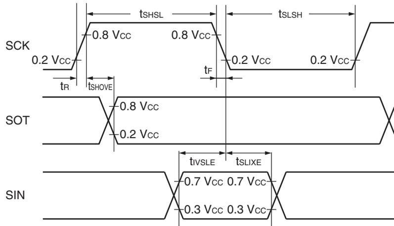
Sampling is executed at the rising edge of the sampling clock\*<sup>1</sup>, and serial clock delay is enabled\*<sup>2</sup>.
