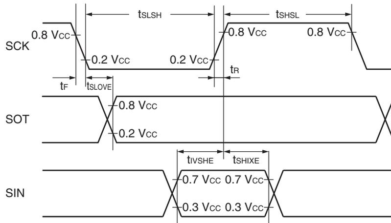
Sampling is executed at the falling edge of the sampling clock\*1, and serial clock delay is disabled\*2.
