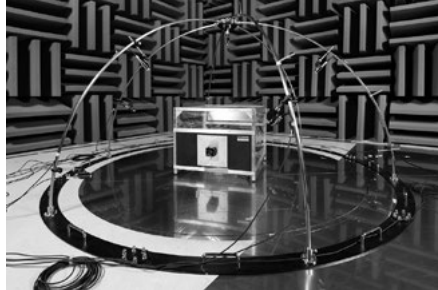
Noise characteristic measurement equipment
