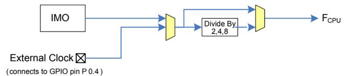
The  $F_{CPU}$  signal can be divided down to generate synchronous clocks for the analog and digital peripherals. There are four clock dividers for the PSoC 4000, each with 16-bit divide capability. The 16-bit capability allows flexible generation of fine-grained frequency values and is fully supported in PSoC Creator.
