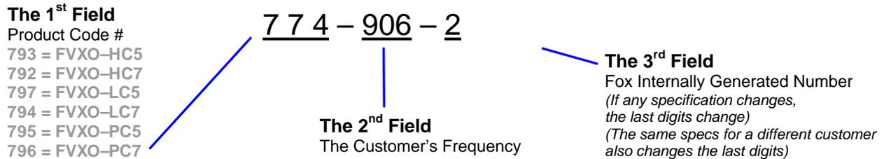
**This example, FXO-PC726R-906 = LVPECL Output, Ceramic, 7 x 5mm Package, 2.5V, ±25 PPM Stability, -40 to +85°C Temperature Range, at 906 MHz**
