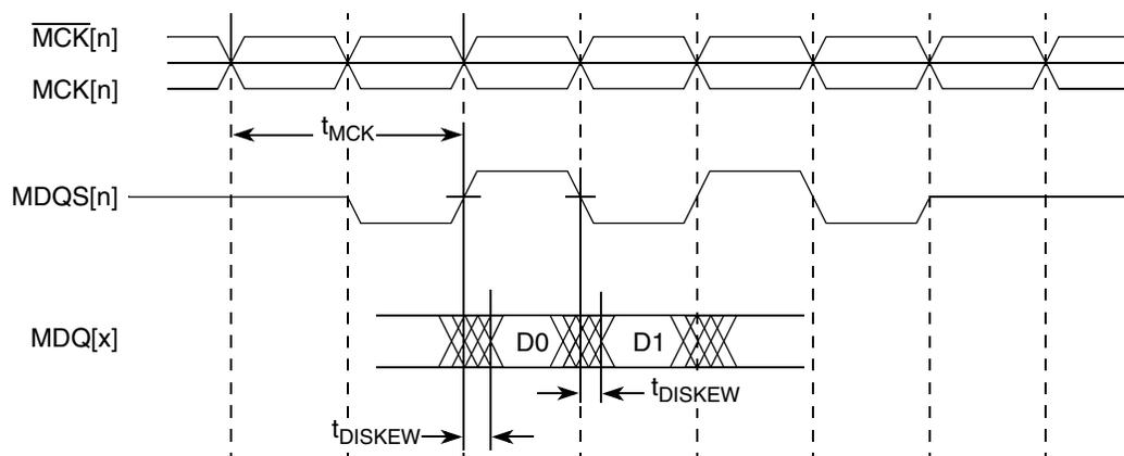
**Figure 3. DDR SDRAM Input Timing Diagram ( $t_{DISKEW}$ )**
