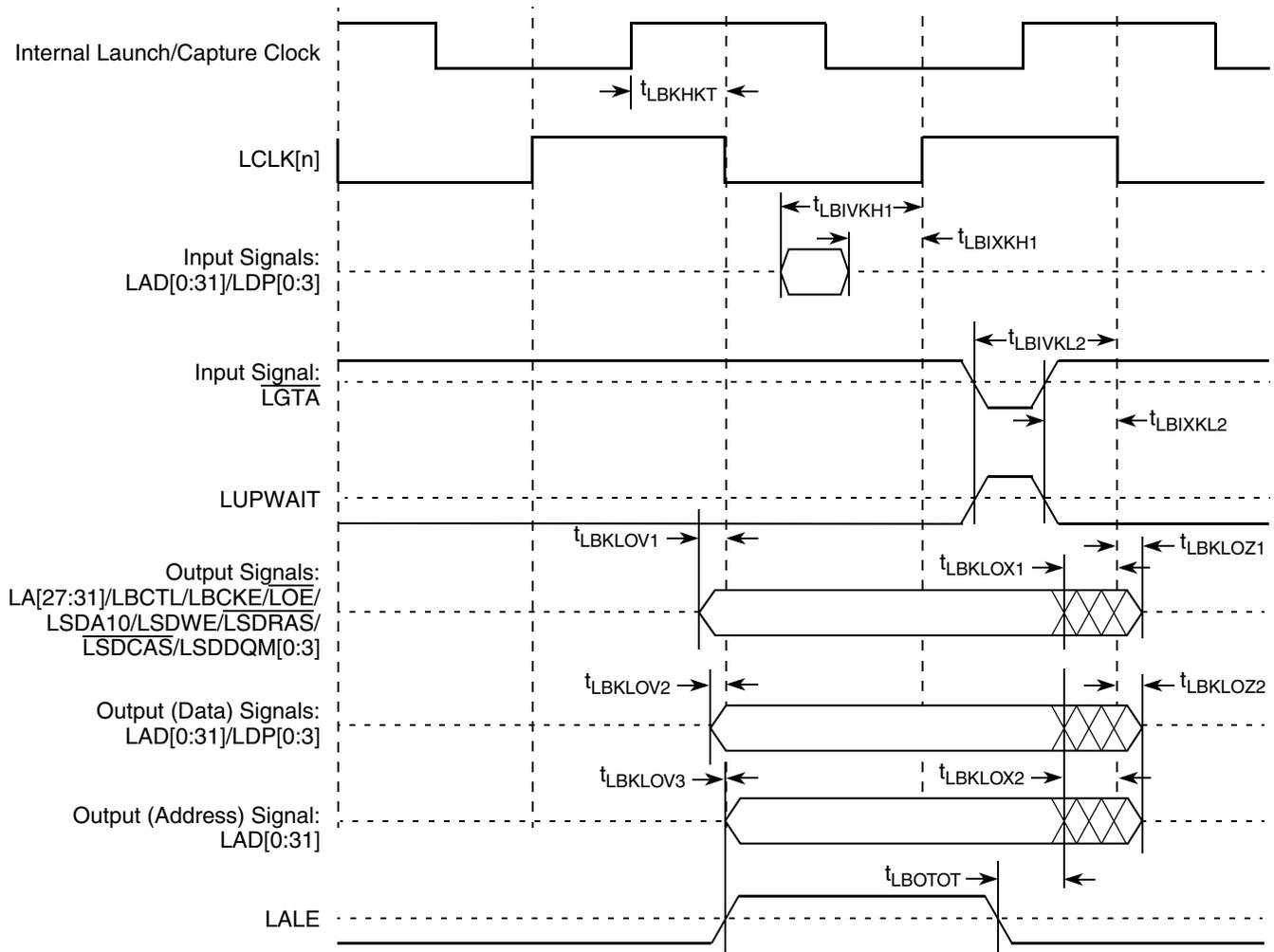
**Figure 29. Local Bus Signals (PLL Bypass Mode)**
