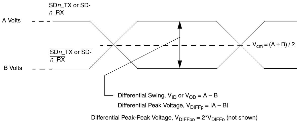
**Figure 44. Differential Voltage Definitions for Transmitter or Receiver**
