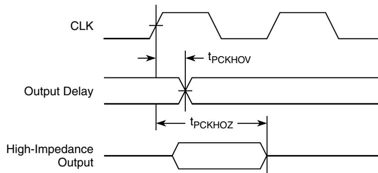
Figure 43. PCI Output AC Timing Measurement Condition
