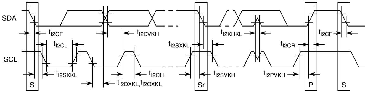
Figure 39. I<sup>2</sup>C Bus AC Timing Diagram
