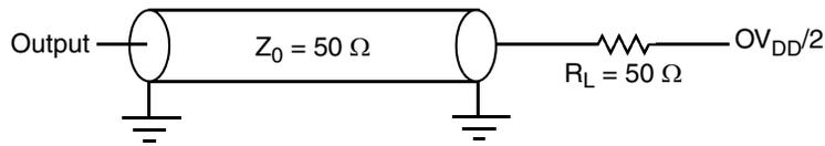
Figure 38. I<sup>2</sup>C AC Test Load
