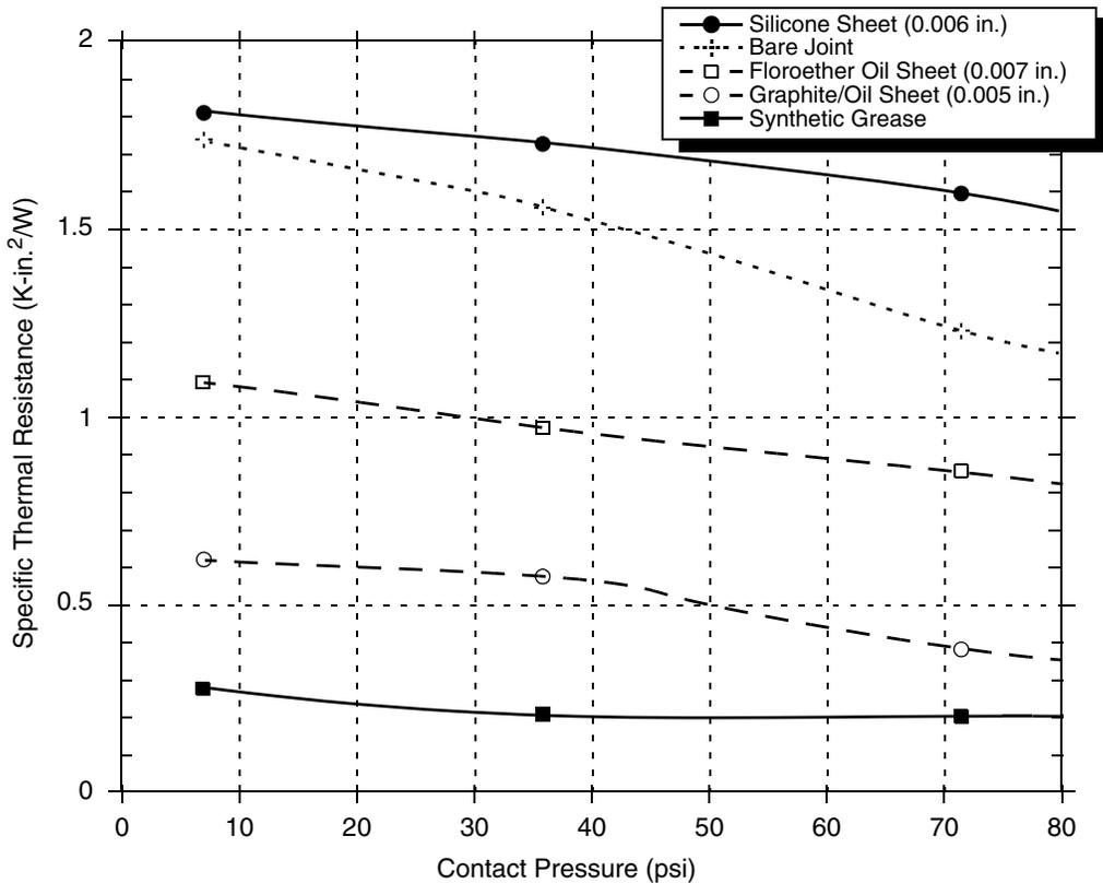
**Figure 63. Thermal Performance of Select Thermal Interface Materials**
