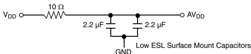
**Figure 65. MPC8544E PLL Power Supply Filter Circuit**
