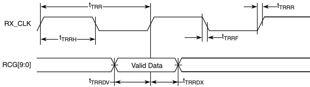
**Figure 21. TBI Single-Clock Mode Receive AC Timing Diagram**
