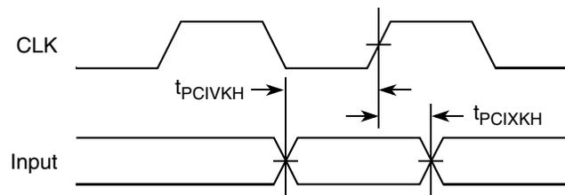
Figure 42. PCI Input AC Timing Measurement Conditions
