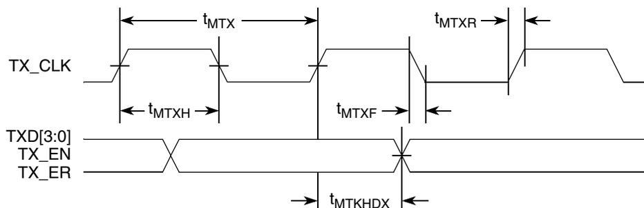
**Figure 16. MII Transmit AC Timing Diagram**
