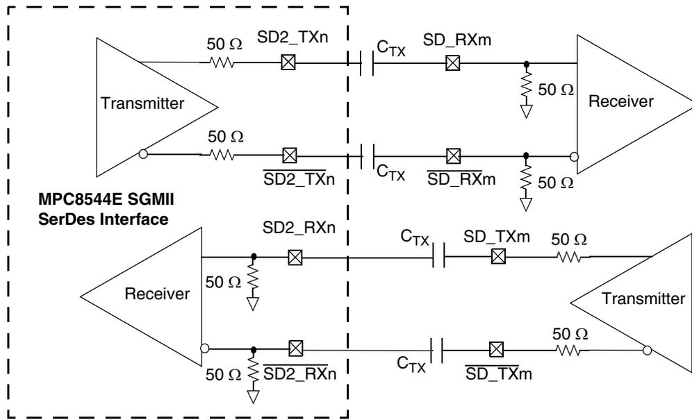
Figure 7. 4-Wire AC-Coupled SGMII Serial Link Connection Example
