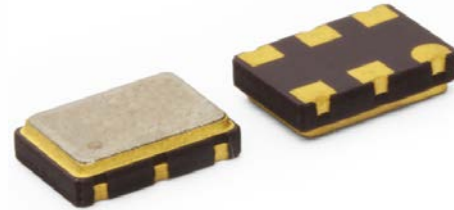
Part Dimensions: 7.0 × 5.0 × 2.0mm • 178.462mg
