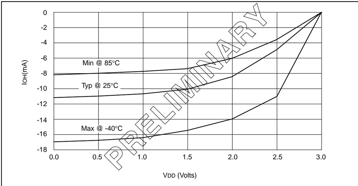
**FIGURE 20-15:  $I_{OH}$  vs.  $V_{OH}$ ,  $V_{DD} = 5V$**
