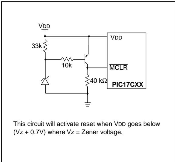
**FIGURE 4-8: PIC17C42 EXTERNAL POWER-ON RESET CIRCUIT (FOR SLOW VDD POWER-UP)**
