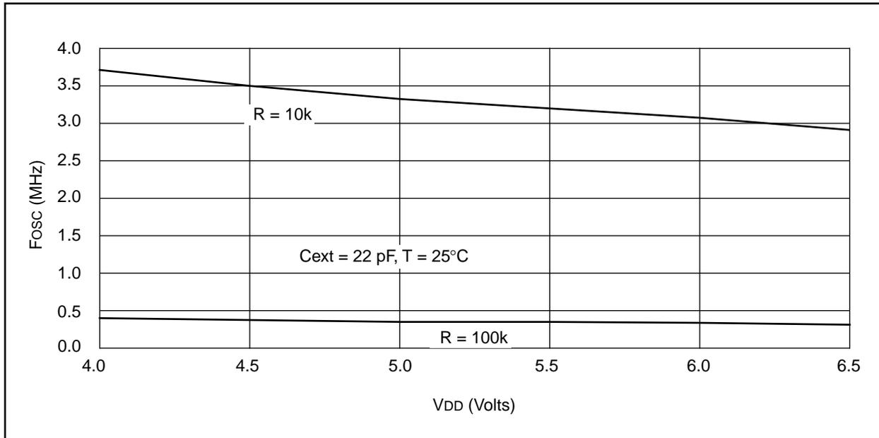
FIGURE 18-3: TYPICAL RC OSCILLATOR FREQUENCY vs. VDD
