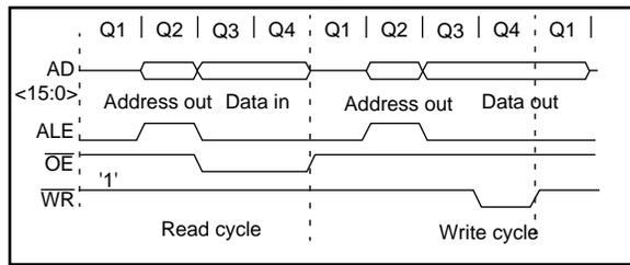
The system bus requires that there is no bus conflict (minimal leakage), so the output value (address) will be capacitively held at the desired value.
