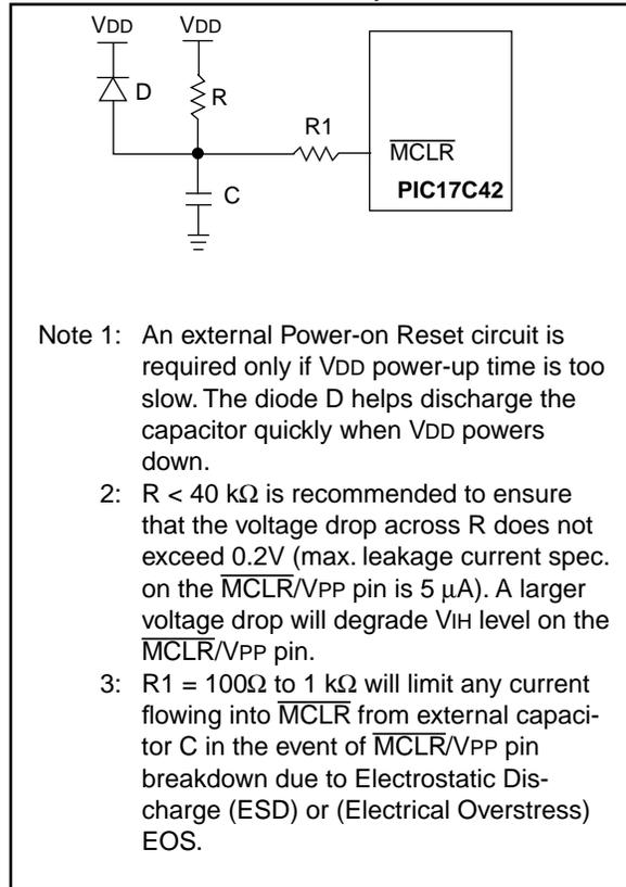
**FIGURE 4-9: BROWN-OUT PROTECTION CIRCUIT 2**
