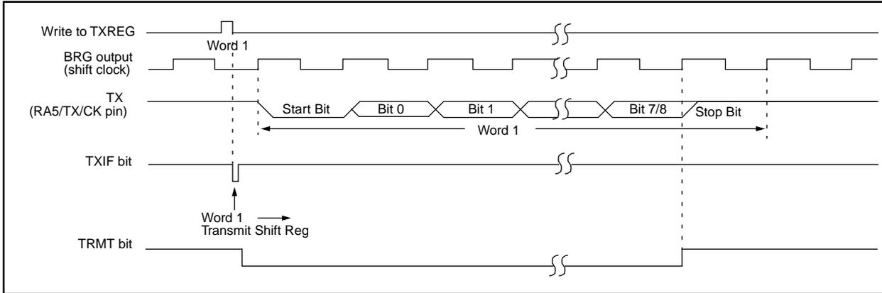
**FIGURE 13-6: ASYNCHRONOUS MASTER TRANSMISSION (BACK TO BACK)**
