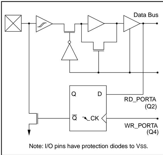
**FIGURE 9-3: RA4 AND RA5 BLOCK DIAGRAM**
