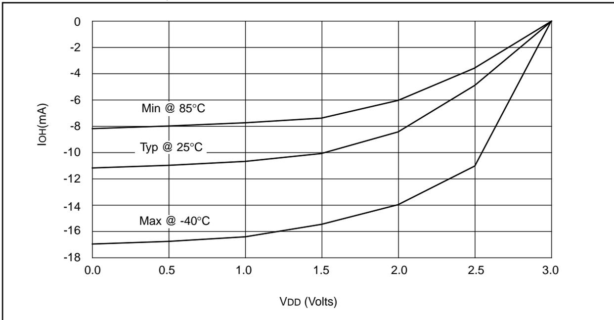
**FIGURE 18-15:  $I_{OH}$  vs.  $V_{OH}$ ,  $V_{DD} = 5V$**
