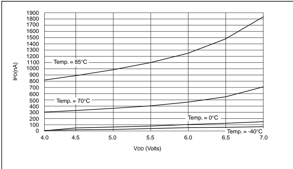
**FIGURE 18-11: TYPICAL  $I_{PD}$  vs.  $V_{DD}$  WATCHDOG ENABLED 25°C**
