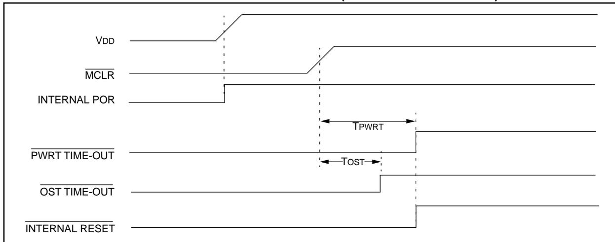
**FIGURE 4-4: SLOW RISE TIME ( $\overline{\text{MCLR}}$  TIED TO  $V_{\text{DD}}$ )**
