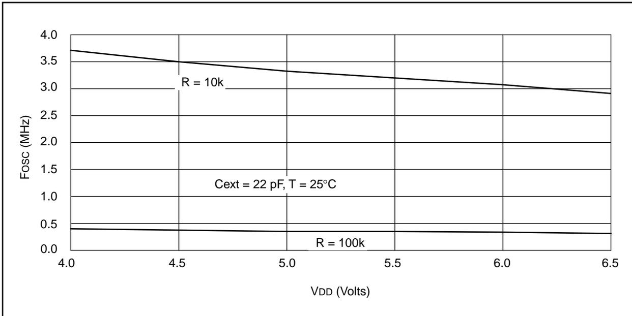
FIGURE 20-3: TYPICAL RC OSCILLATOR FREQUENCY vs. VDD
