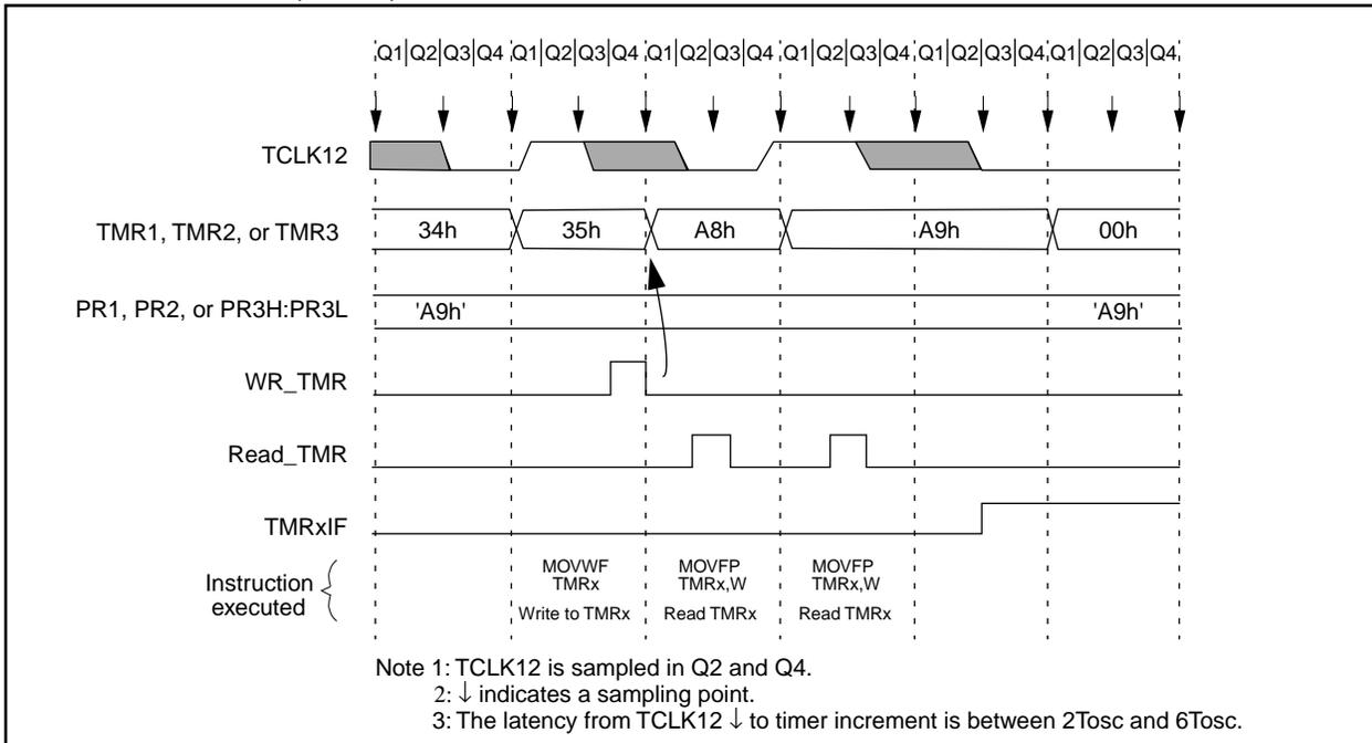
**FIGURE 12-10: TMR1, TMR2, AND TMR3 OPERATION IN TIMER MODE**
