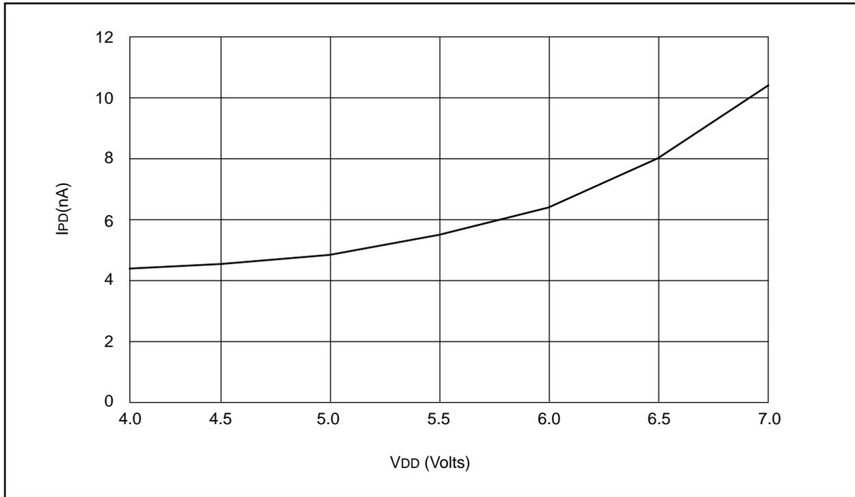
FIGURE 18-10: MAXIMUM  $I_{PD}$  vs.  $V_{DD}$  WATCHDOG DISABLED
