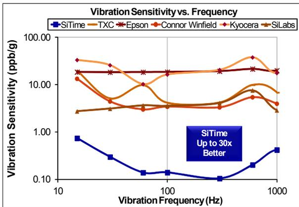
Figure 5. Vibration Robustness<sup>[5]</sup>
