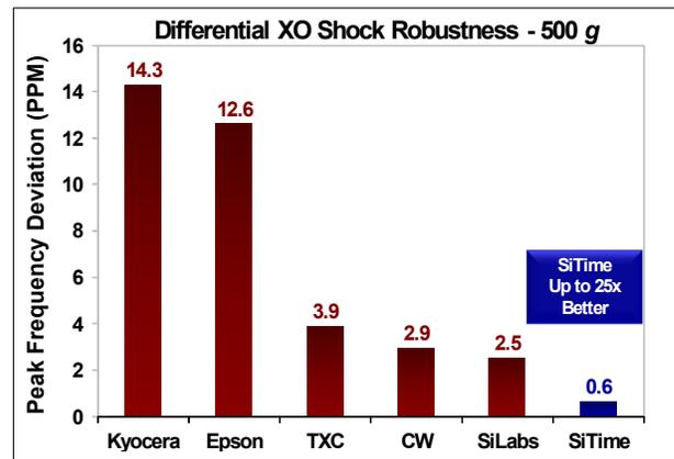
Figure 6. Shock Robustness<sup>[6]</sup>
