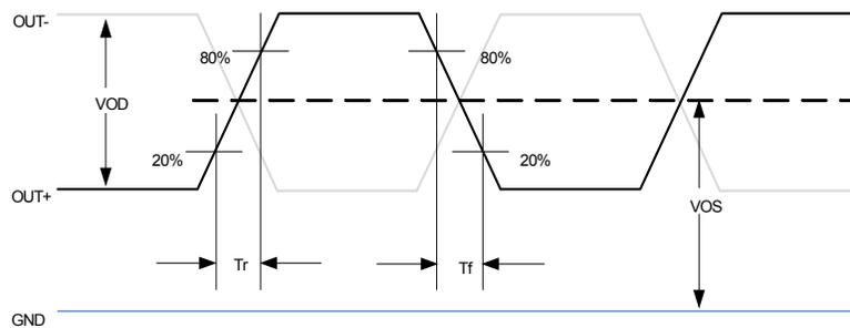
**Figure 2. LVDS Voltage Levels per Differential Pin (OUT+/OUT-)**
