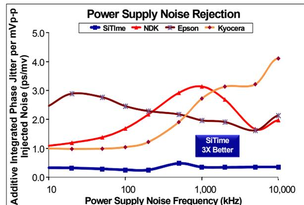
Figure 4. Power Supply Noise Rejection<sup>[4]</sup>
