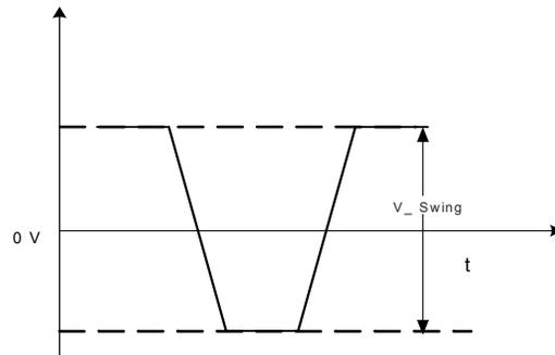
**Figure 1(b). LVPECL Voltage Levels Across Differential Pair**
