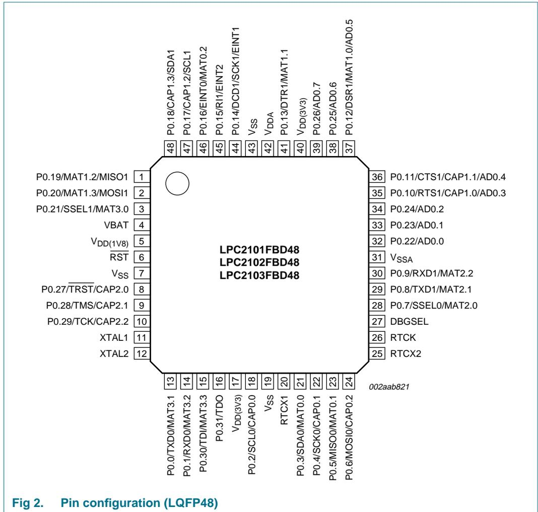
Fig 2. Pin configuration (LQFP48)
