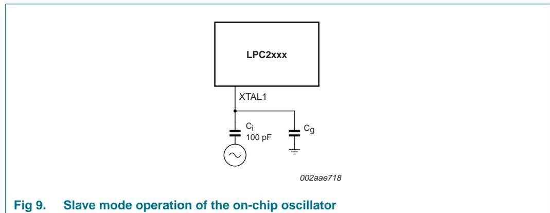
**Fig 9. Slave mode operation of the on-chip oscillator**
