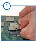
Place FC around two corners of the component. FC will bend slightly at the "horseshoe" tab. Note the direction of air flow when placing your HS.
