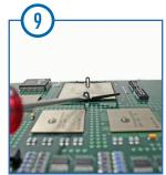
Remove the FC by placing a small screwdriver within the "horseshoe" tab and gently twisting in either direction to pull the frame clip away from the component.
