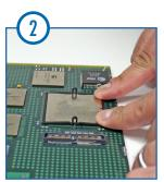
Press opposite end of the FC down until it is secure around the component's edges.
