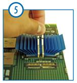
Place spring clip within the HS' fin field as shown. The ends of the SC will fit over the "horseshoe" tabs.
