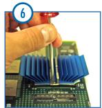
Push opposite end of the SC down over the FC with a small screwdriver until it fits securely on the assembly.
