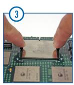
To ensure a secure fit, push spread apart FC slightly at the "horseshoe" tabs while pressing down.
