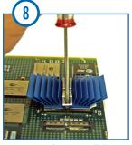
To remove, place a small flathead screwdriver between the spring clip and the frame clip and pry the spring clip away from the frame.
