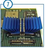
Shown above the is the HS, FC and SC assembly properly seated over the component.
