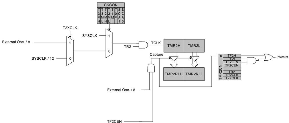
Figure 18.6. Timer 2 Capture Mode Block Diagram
