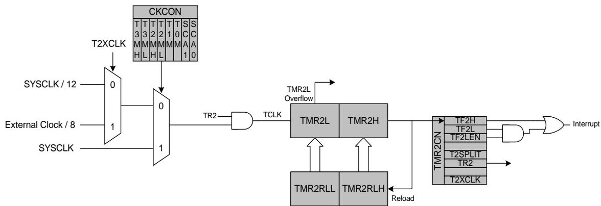
Figure 18.4. Timer 2 16-Bit Mode Block Diagram
