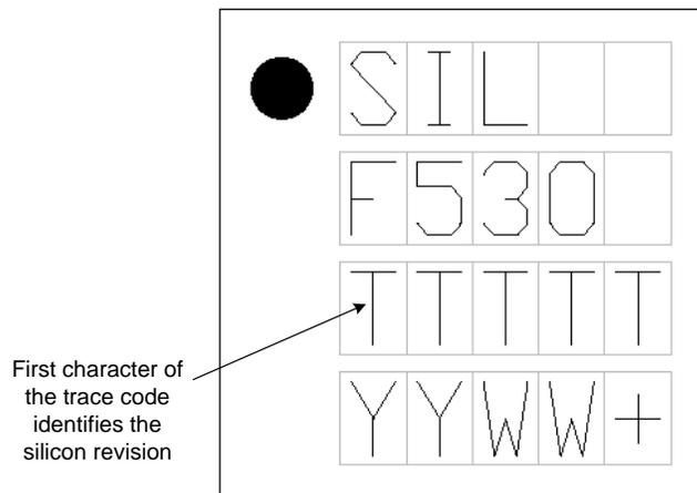
Figure 20.2. Device Package—QFN 20
