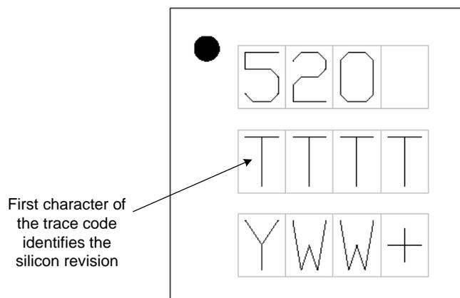
Figure 20.3. Device Package—DFN 10
