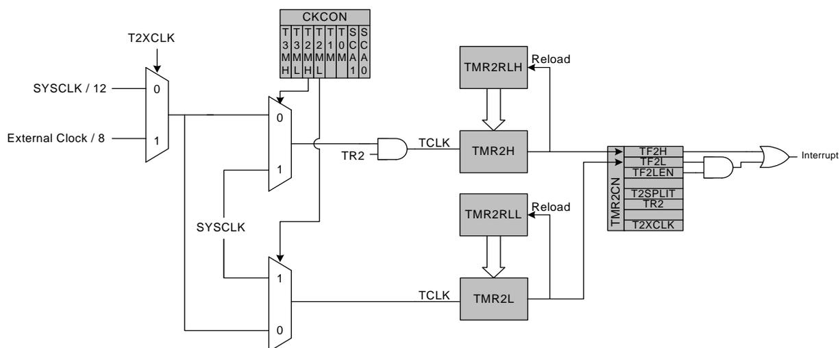
Figure 18.5. Timer 2 8-Bit Mode Block Diagram
