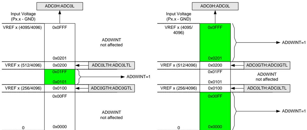
Figure 4.7. ADC Window Compare Example: Right-Justified Single-Ended Data
