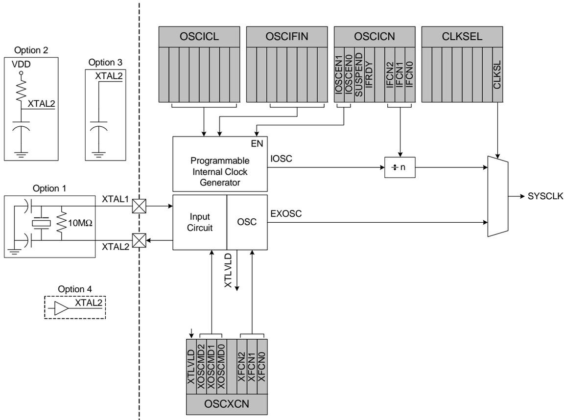
**Figure 14.1. Oscillator Diagram**
