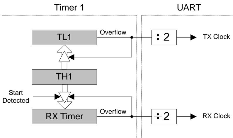
**Figure 15.2. UART0 Baud Rate Logic**
