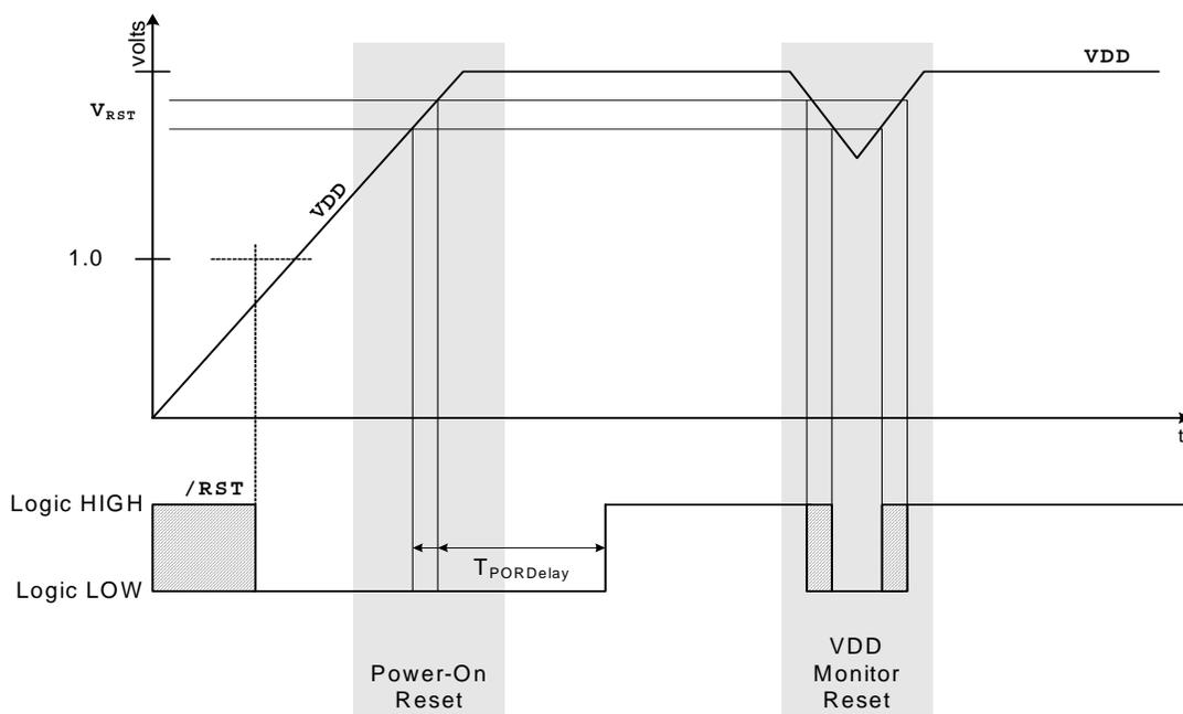
Figure 11.2. Power-On and  $V_{\text{DD}}$  Monitor Reset Timing
