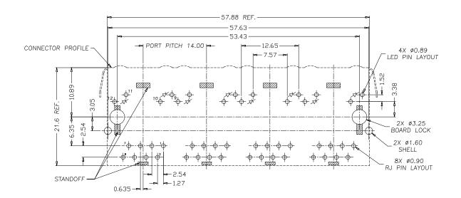
RECOMMENDED PCB LAYOUT  $\begin{array}{c} {\sf COMPONENT \ SIDE} \\ {\sf ALL \ DIMENSION \ TOLERANCE \ ARE \ \pm 0.05mm \ UNLESS \ OTHERWISE \ SPECIFIED} \end{array}$
