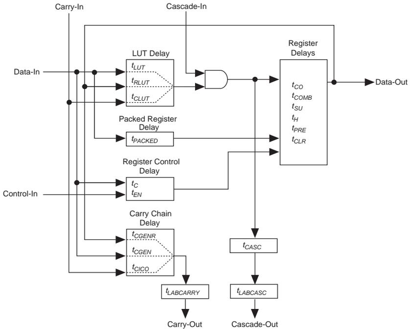
Figure 26. FLEX 10KE Device IOE Timing Model
