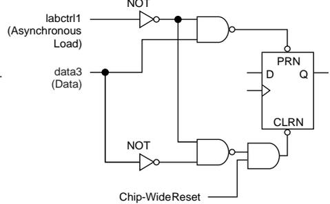
Asynchronous Load with Preset
