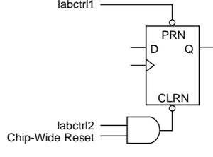
Asynchronous Load with Clear
