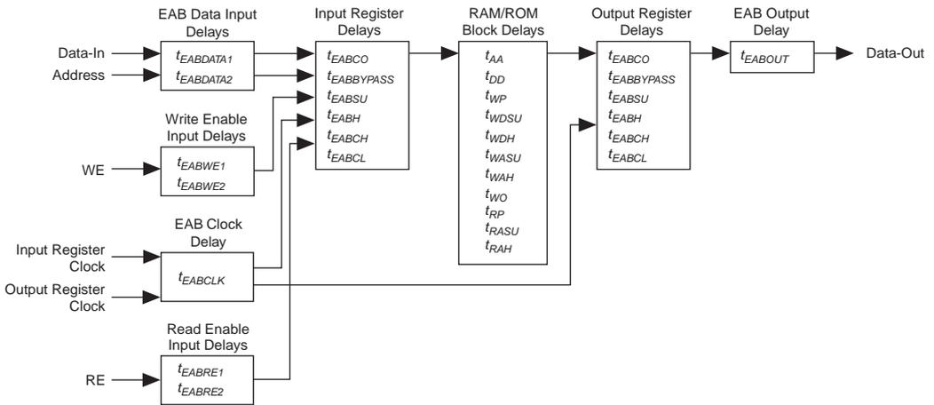
Figure 28. Synchronous Bidirectional Pin External Timing Model
