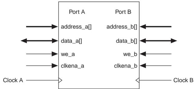
The FLEX 10KE EAB can be used in a single-port mode, which is useful for backward-compatibility with FLEX 10K designs (see [Figure 4](#)).
