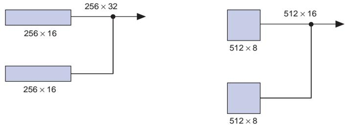
If necessary, all EABs in a device can be cascaded to form a single RAM block. EABs can be cascaded to form RAM blocks of up to 2,048 words without impacting timing. The Altera software automatically combines EABs to meet a designer's RAM specifications.
