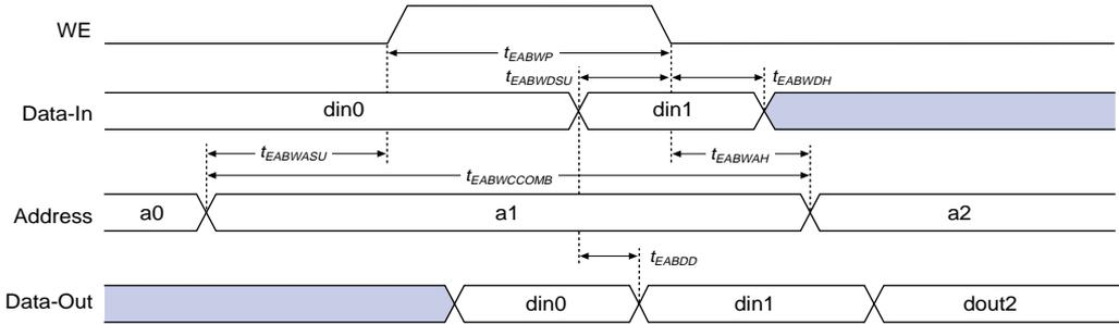
Figure 30. EAB Synchronous Timing Waveforms
