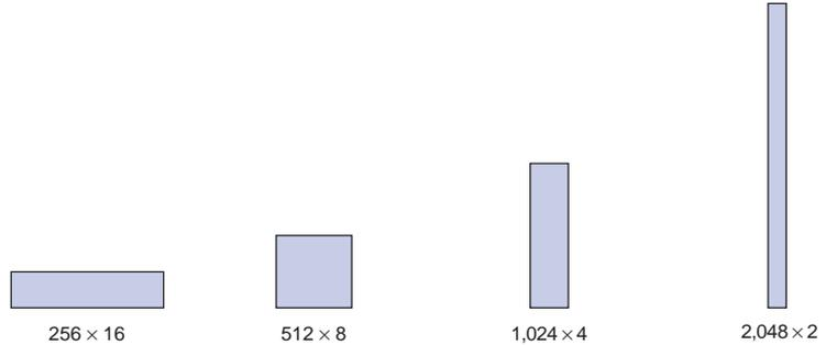
Larger blocks of RAM are created by combining multiple EABs. For example, two  $256 \times 16$  RAM blocks can be combined to form a  $256 \times 32$  block; two  $512 \times 8$  RAM blocks can be combined to form a  $512 \times 16$  block (see [Figure 6](#)).
