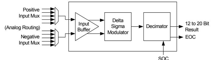
Resolution and sample rate are controlled by the Decimator. Data is pipelined in the decimator; the output is a function of the last four samples. When the input multiplexer is switched, the output data is not valid until after the fourth sample after the switch.
