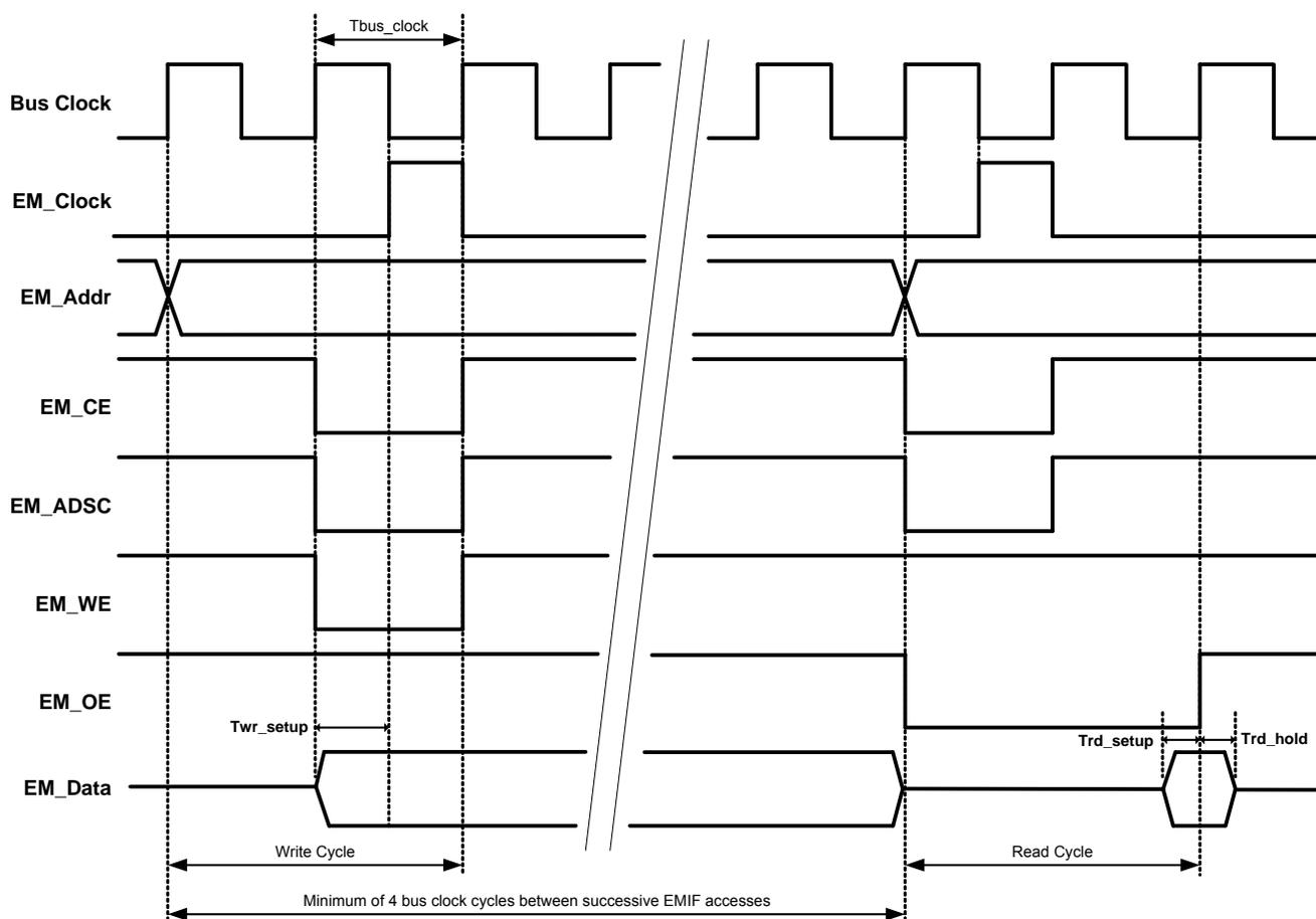
Table 11-54. Synchronous Write and Read Timing Specifications<sup>[59]</sup>
