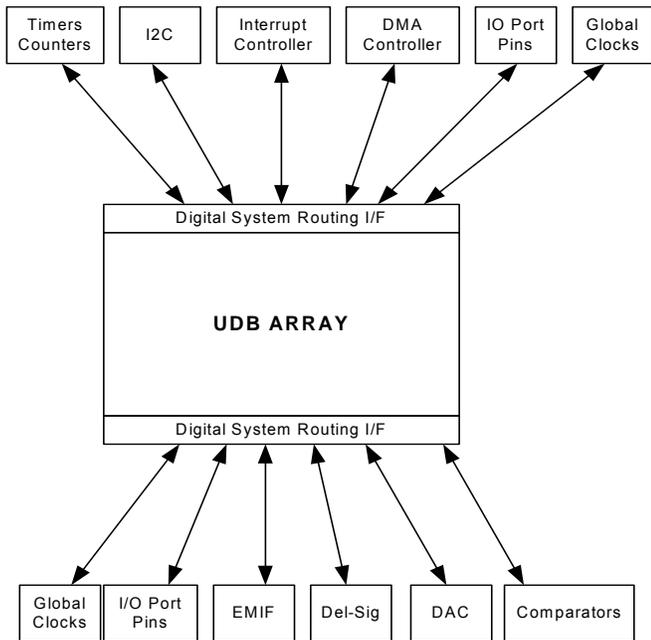
Interrupt and DMA routing is very flexible in the CY8C32 programmable architecture. In addition to the numerous fixed function peripherals that can generate interrupt requests, any data signal in the UDB array routing can also be used to generate a request. A single peripheral may generate multiple independent interrupt requests simplifying system and firmware design. Figure 7-10 shows the structure of the IDMUX (Interrupt/DMA Multiplexer).
