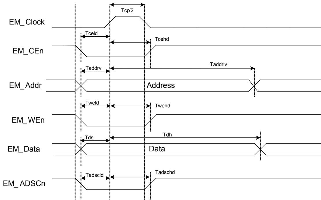
**Table 11-56. Synchronous Write Cycle Specifications**
