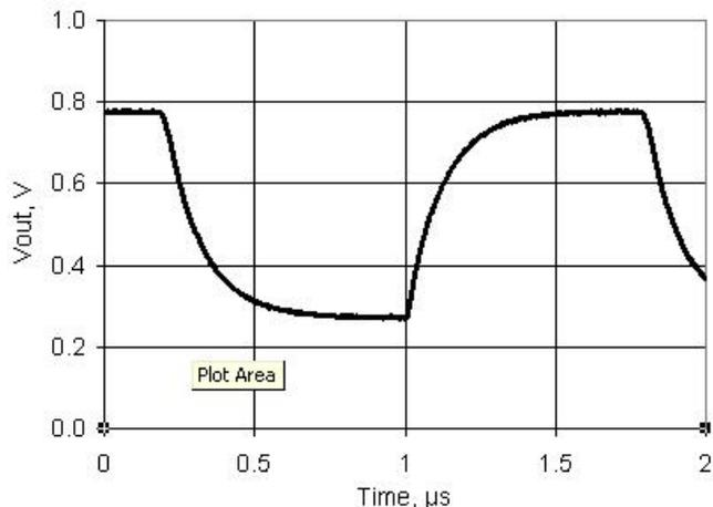
**Figure 11-49. VDAC Glitch Response, Codes 0x7F - 0x80, 1 V Mode, High speed mode, V<sub>DDA</sub> = 5 V**
