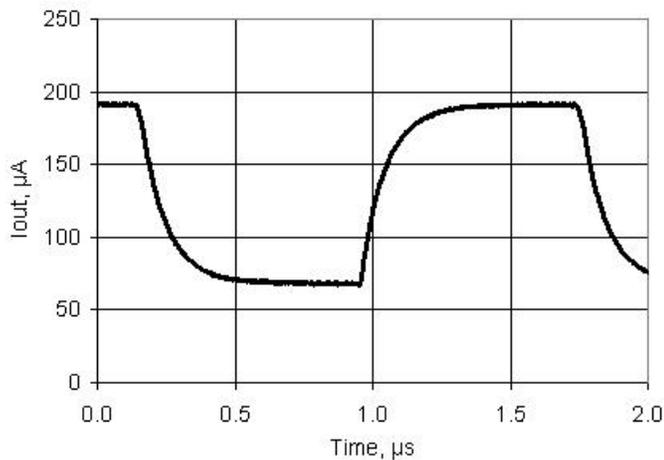
**Figure 11-37. IDAC Glitch Response, Codes 0x7F - 0x80, 255  $\mu$ A Mode, Source Mode, High speed mode, V<sub>D<sub>DA</sub></sub> = 5 V**
