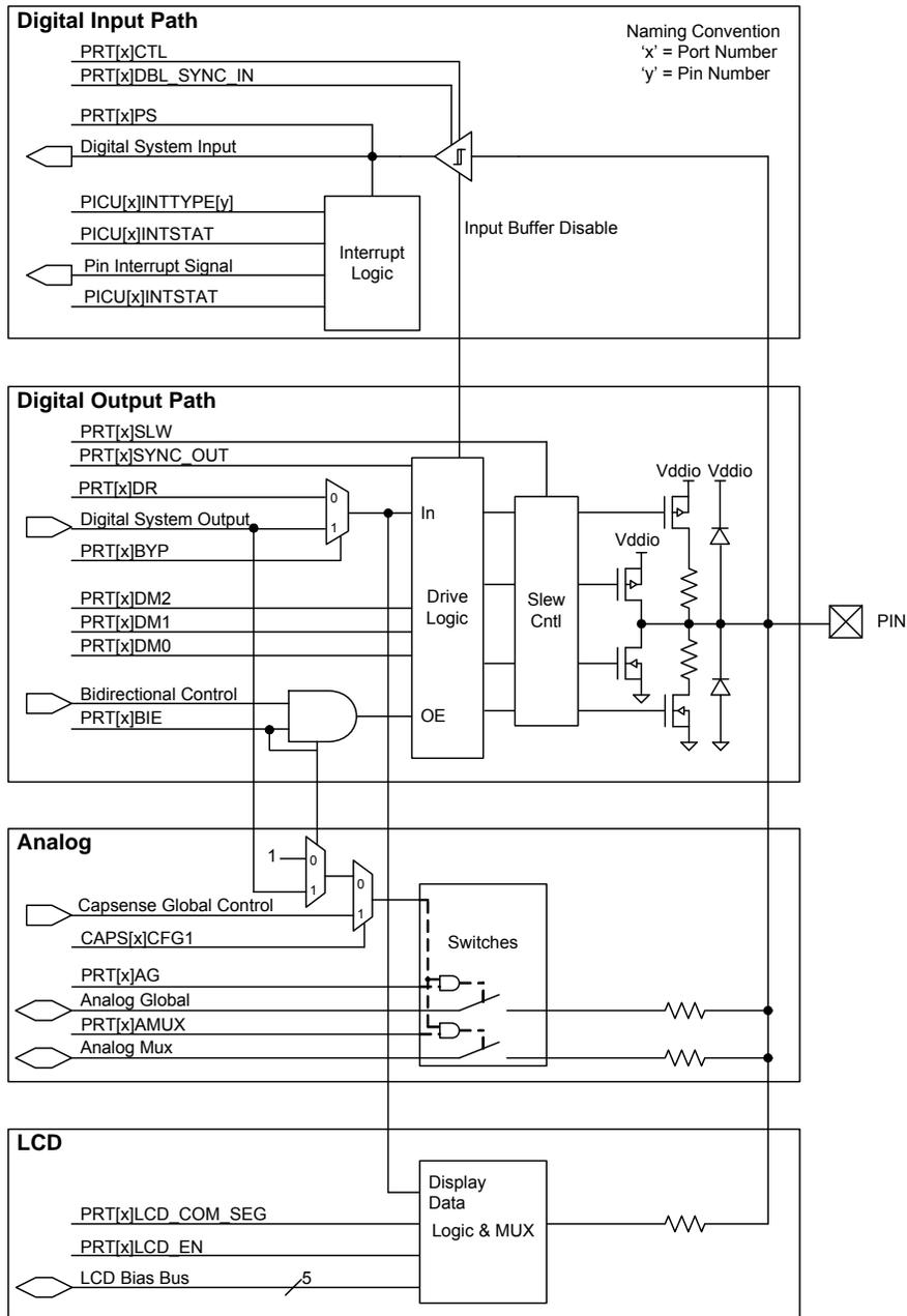
Figure 6-10. SIO Input/Output Block Diagram
