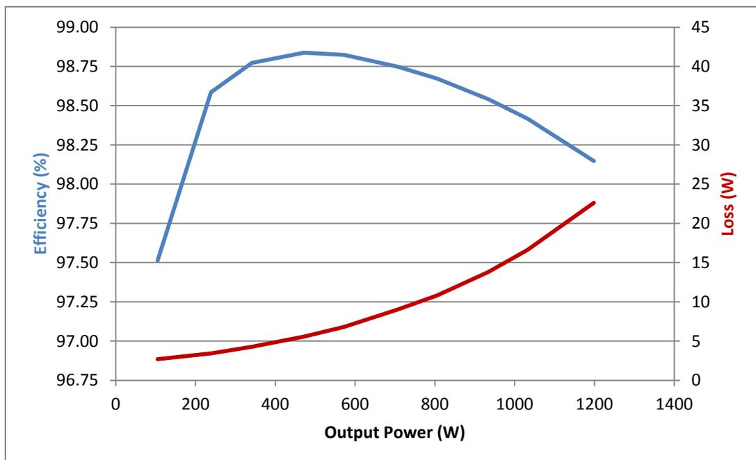
Figure 7. Typical Efficiency 350Vdc input, 240Vac output
