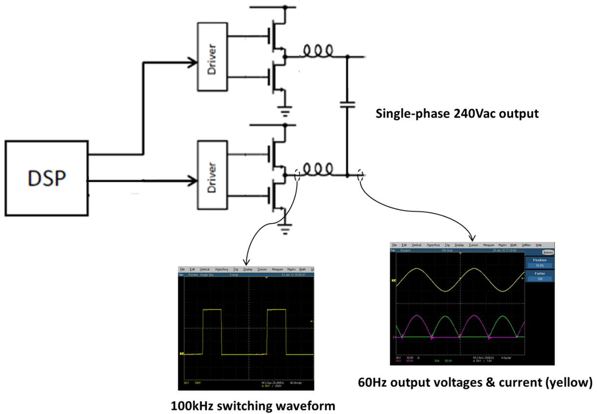
Figure 6. Typical Waveforms
