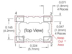
\* Do not route any traces in the keep out area. It is recommended the next layer under the keep out area is to be ground plane.
