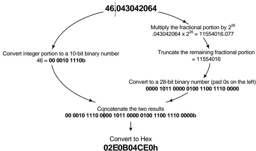
**Figure 4. Example of RFREQ Decimal to Hexadecimal Conversion**
