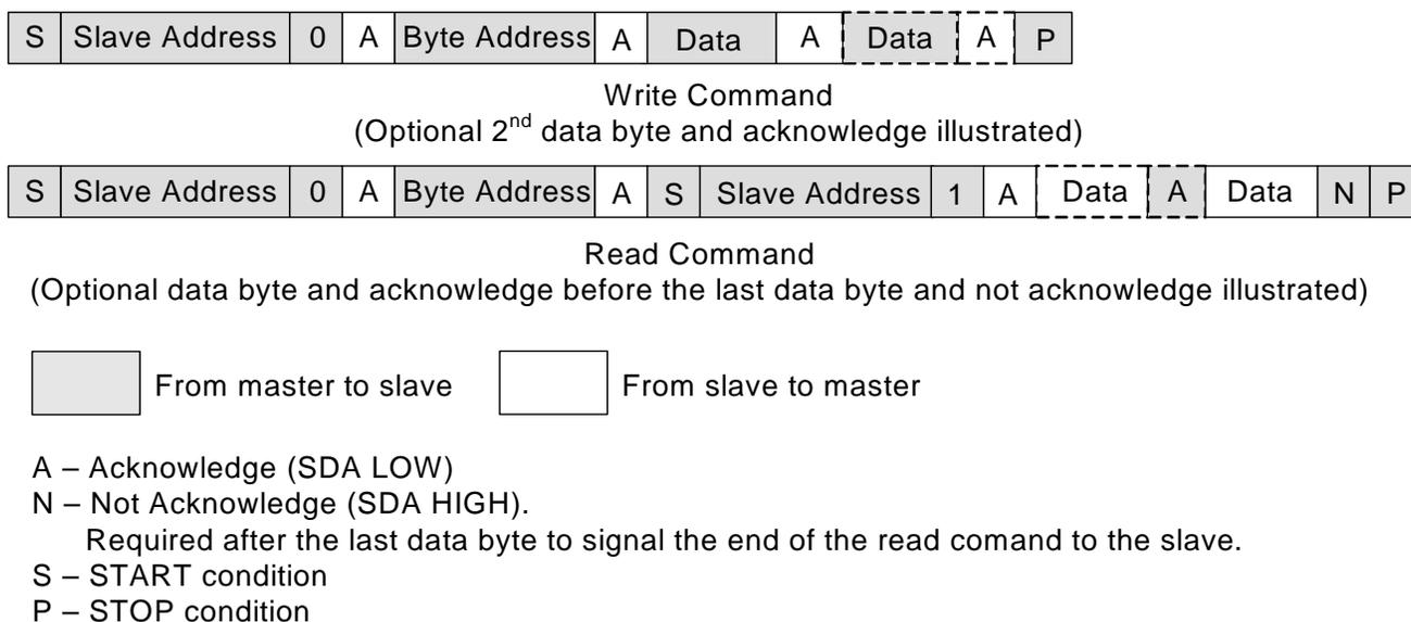
**Figure 5. I<sup>2</sup>C Command Format**
