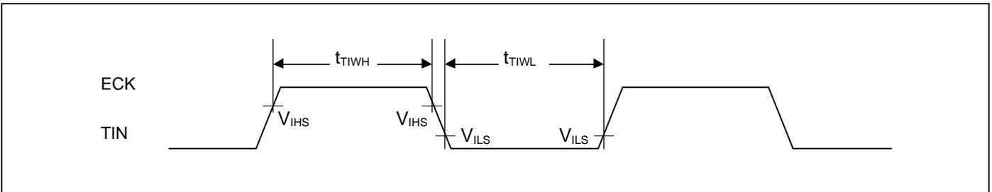
**Trigger input timing**
