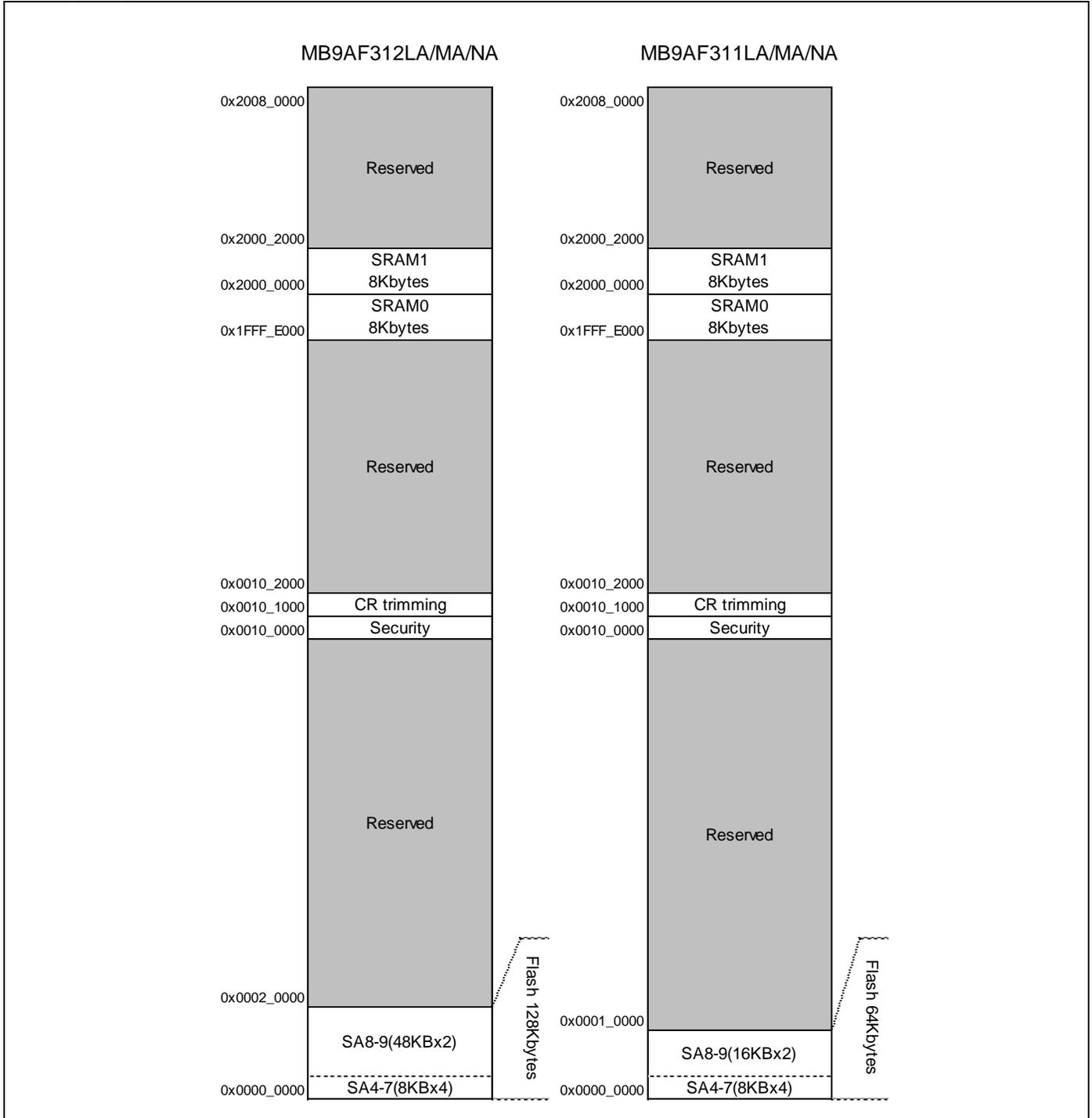
\*: See "MB9A310A/110A Series Flash programming Manual" for sector structure of Flash.
