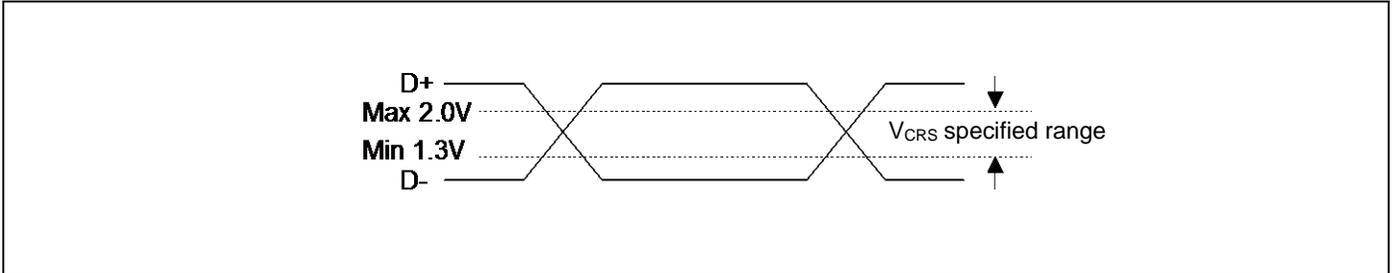
\*5: They indicate rising time ( $T_{rise}$ ) and falling time ( $T_{fall}$ ) of the full-speed differential data signal. They are defined by the time between 10% and 90% of the output signal voltage. For full-speed buffer,  $T_r/T_f$  ratio is regulated as within  $\pm 10\%$  to minimize RFI emission.
