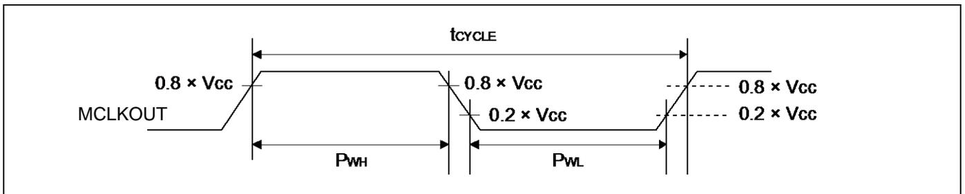
**External bus signal input/output characteristics**
