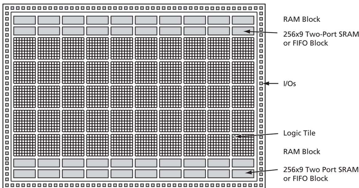
Figure 1-1 • The ProASIC<sup>PLUS</sup> Device Architecture
