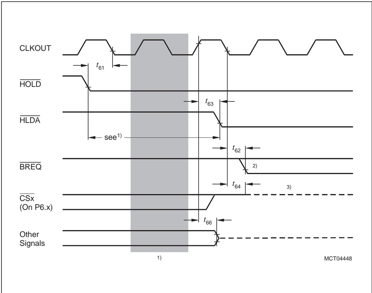
**Figure 22 External Bus Arbitration, Releasing the Bus**
