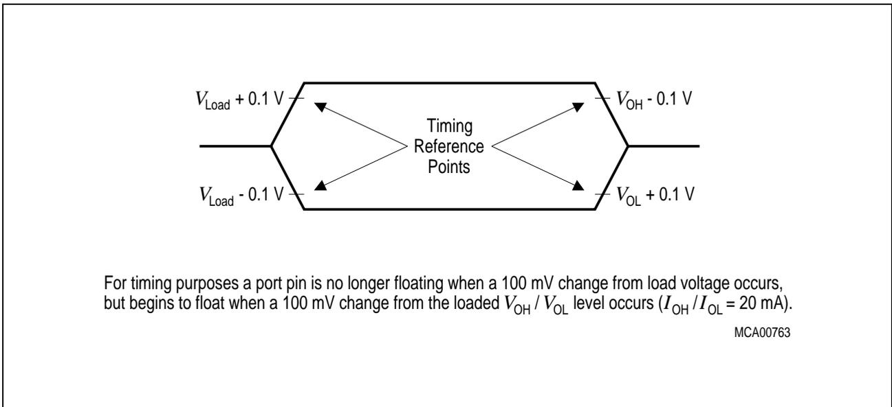
**Figure 12 Float Waveforms**
