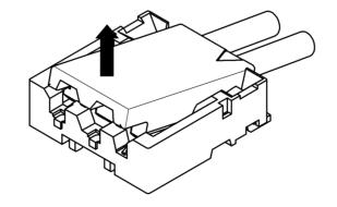
Slift up to the upper direction and positive lock is released. Removal completes.
