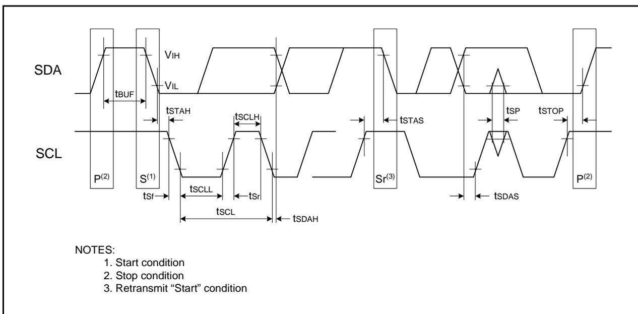
**Figure 5.7 I/O Timing of I<sup>2</sup>C Bus Interface**
