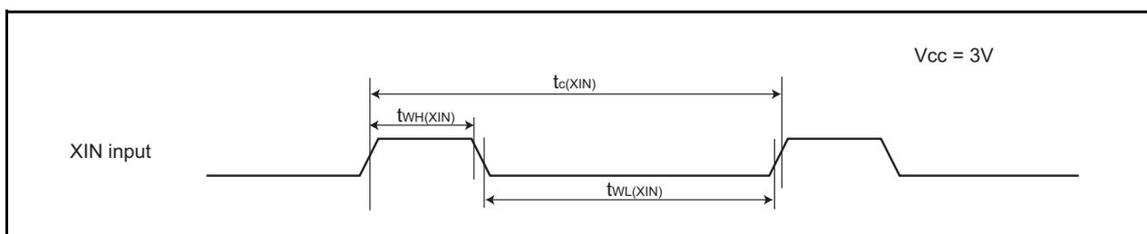
**Figure 5.12 XIN Input Timing Diagram when  $V_{CC} = 3\text{ V}$** **Table 5.23 TRAIO Input**
