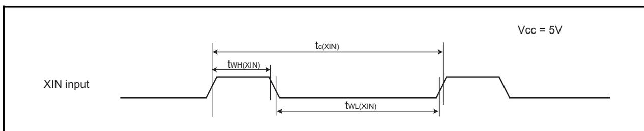
**Figure 5.8 XIN Input Timing Diagram when  $V_{CC} = 5\text{ V}$** **Table 5.17 TRAIO Input**
