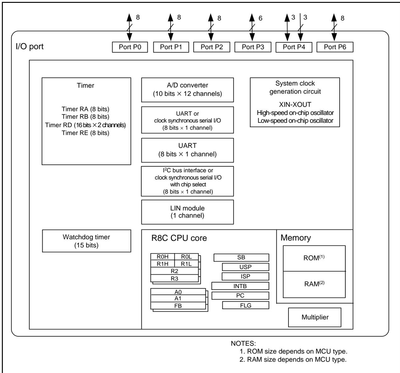
Figure 1.1 Block Diagram
