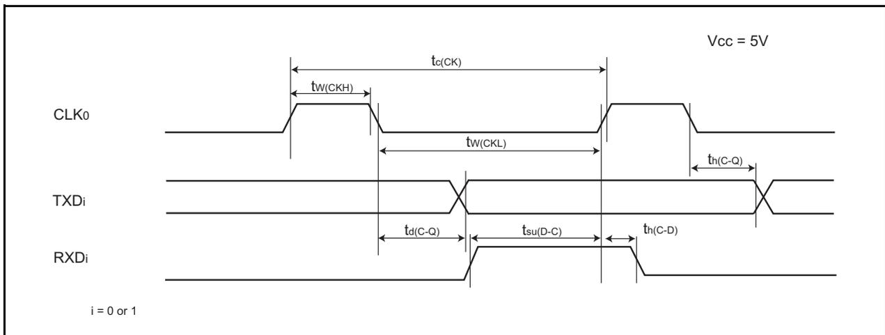
**Figure 5.10 Serial Interface Timing Diagram when Vcc = 5 V****Table 5.19 External Interrupt  $\overline{INTi}$  (i = 0 to 3) Input**
