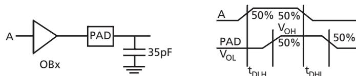
Figure 1-27 • Output Buffer Delays
