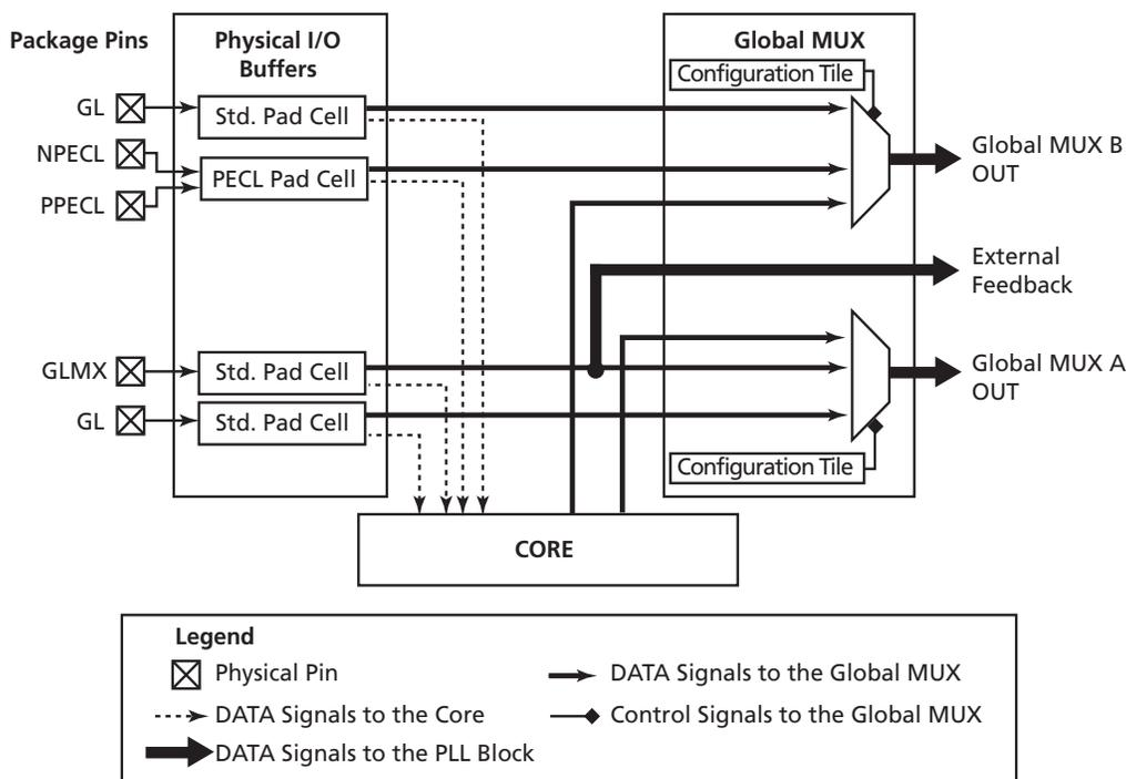
**Note:** When a signal from an I/O tile is connected to the core, it cannot be connected to the Global MUX at the same time.
