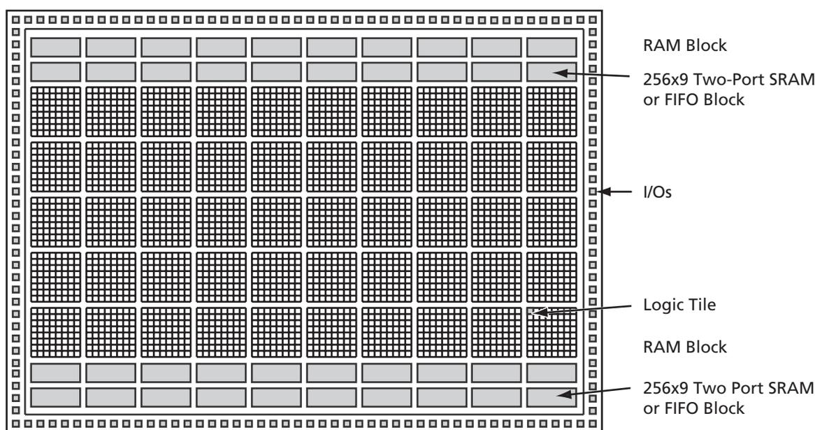
Figure 1-1 • The ProASIC<sup>PLUS</sup> Device Architecture
