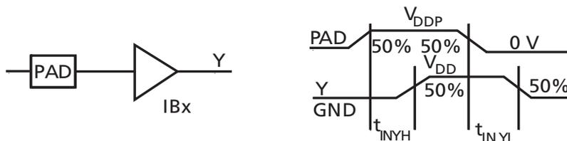
Figure 1-28 • Input Buffer Delays
