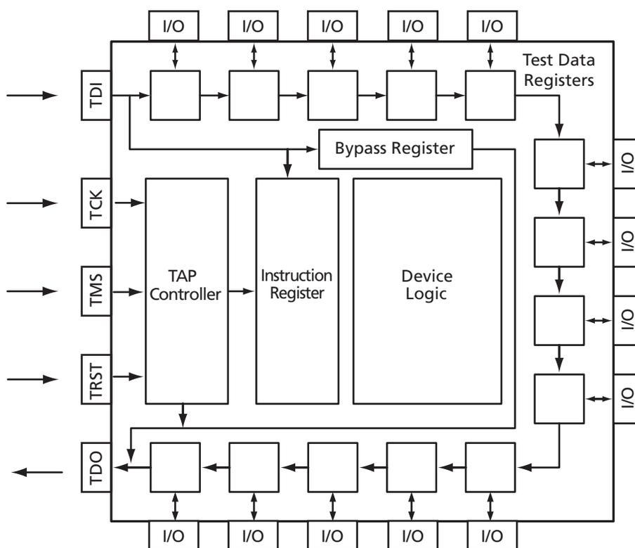
Figure 1-12 • ProASIC<sup>PLUS</sup> JTAG Boundary Scan Test Logic Circuit
