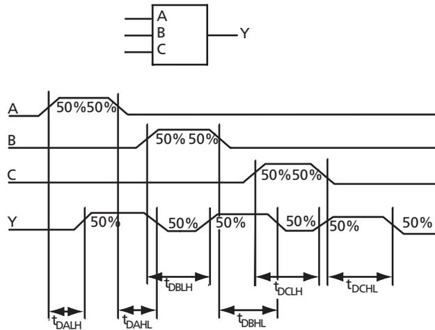
Figure 1-29 • Module Delays
