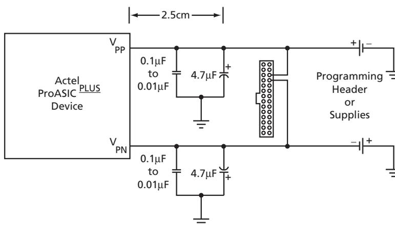
Figure 1-49 • ProASIC<sup>PLUS</sup> V<sub>PP</sub> and V<sub>PN</sub> Capacitor Requirements
