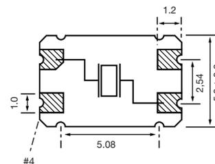
Figure 3) CSM-8B – Pad Configuration Bottom view
