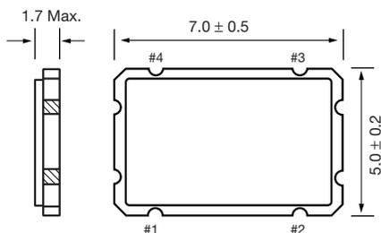
Figure 1) CSM-8 – Side and Top view
