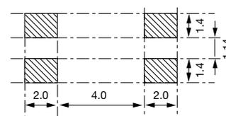
Figure 6) CSM-8B – Recommended Solder Pad Layout Top view
