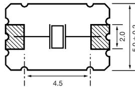
Figure 2) CSM-8A – Pad Configuration Bottom view
