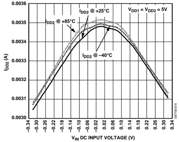
Figure 15.  $I_{DD2}$  vs.  $V_{IN}$  at Various Temperatures
