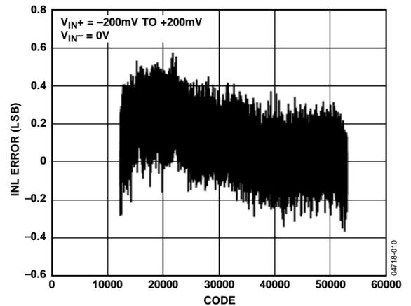
Figure 11. Typical INL, ±200 mV Range (Using Sinc<sup>3</sup> Filter, 256 Decimation Rate)
