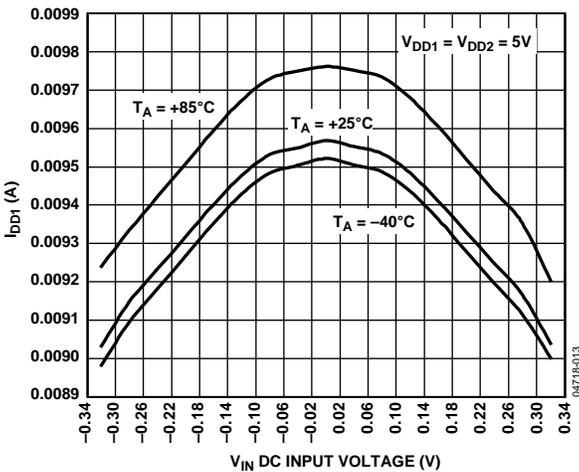
Figure 14.  $I_{DD1}$  vs.  $V_{IN}$  at Various Temperatures
