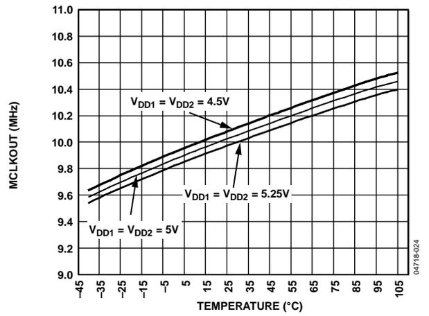
Figure 19. MCLKOUT vs. Temperature for Various Supplies
