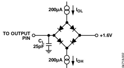
Figure 2. Load Circuit for Digital Output Timing Specifications
