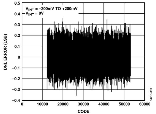
Figure 10. Typical DNL, ±200 mV Range (Using Sinc<sup>3</sup> Filter, 256 Decimation Rate)
