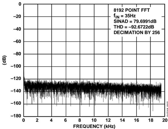
Figure 8. Typical FFT, ±200 mV Range (Using Sinc<sup>3</sup> Filter, 256 Decimation Rate)
