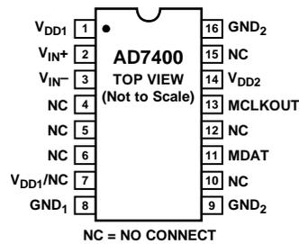
Figure 5. Pin Configuration
