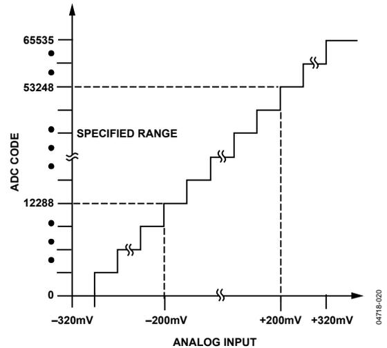
Figure 21. Filtered and Decimated 16-Bit Transfer Characteristic
