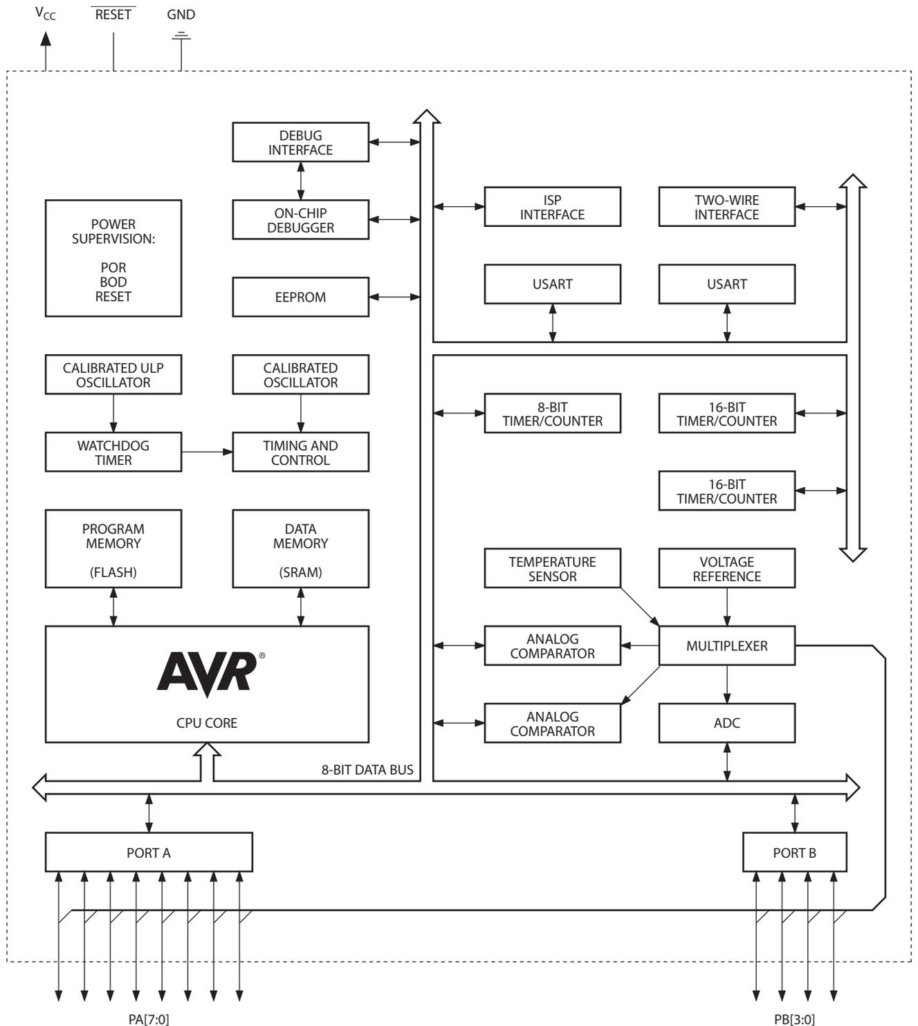
The AVR core combines a rich instruction set with 32 general purpose working registers. All 32 registers are directly connected to the Arithmetic Logic Unit (ALU), allowing two independent registers to be accessed in a single instruction, executed in one clock cycle. The resulting architecture is compact and code efficient while achieving throughputs up to ten times faster than conventional CISC microcontrollers.
