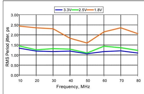
**Figure 9. RMS Period Jitter vs Frequency**
