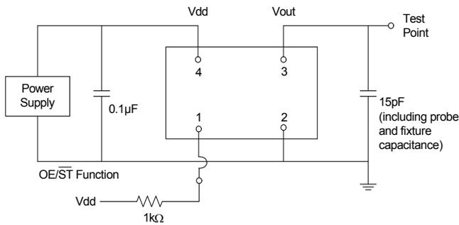
**Figure 2. Test Circuit**
