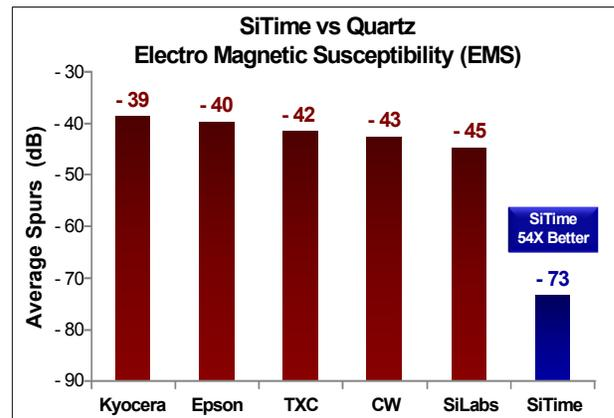
Figure 3. Electro Magnetic Susceptibility (EMS)<sup>[3]</sup>
