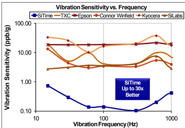
Figure 5. Vibration Robustness<sup>[5]</sup>
