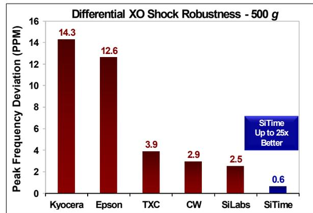
Figure 6. Shock Robustness<sup>[6]</sup>
