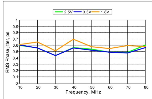
**Figure 11. RMS Phase Jitter vs Frequency**
