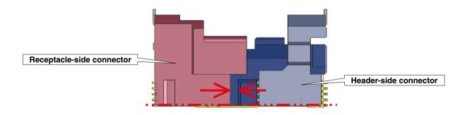
•Using excessive force when mating these connectors may result in damage and alter their performance. Although they are designed with a prevention mechanism to resist incorrect insertion, do not forcibly mate them. Before mating the connector confirm the connector polarity as shown below.
