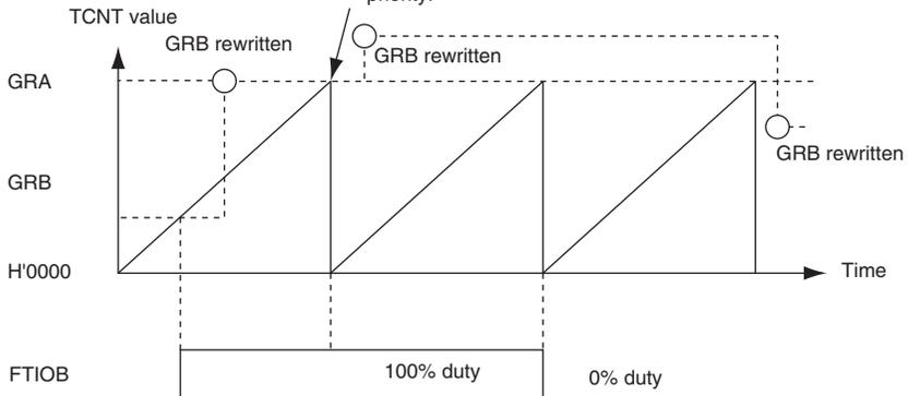
**Figure 13.25 Example of PWM Mode Operation (4)**
