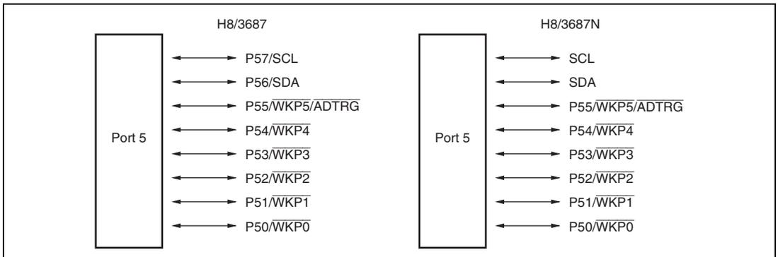
**Figure 9.4 Port 5 Pin Configuration**
