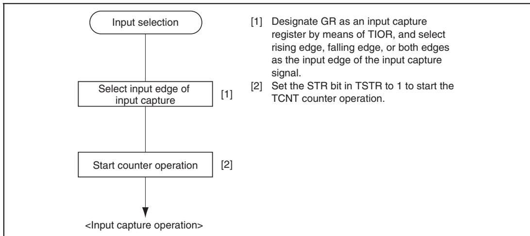
**Figure 13.16 Example of Input Capture Operation Setting Procedure**
