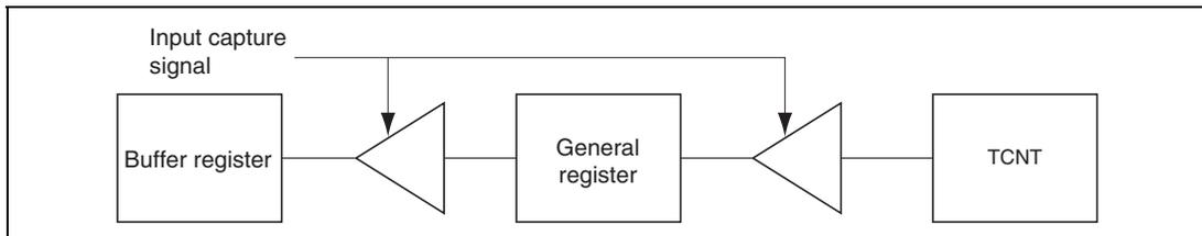
**Figure 13.36 Input Capture Buffer Operation**
