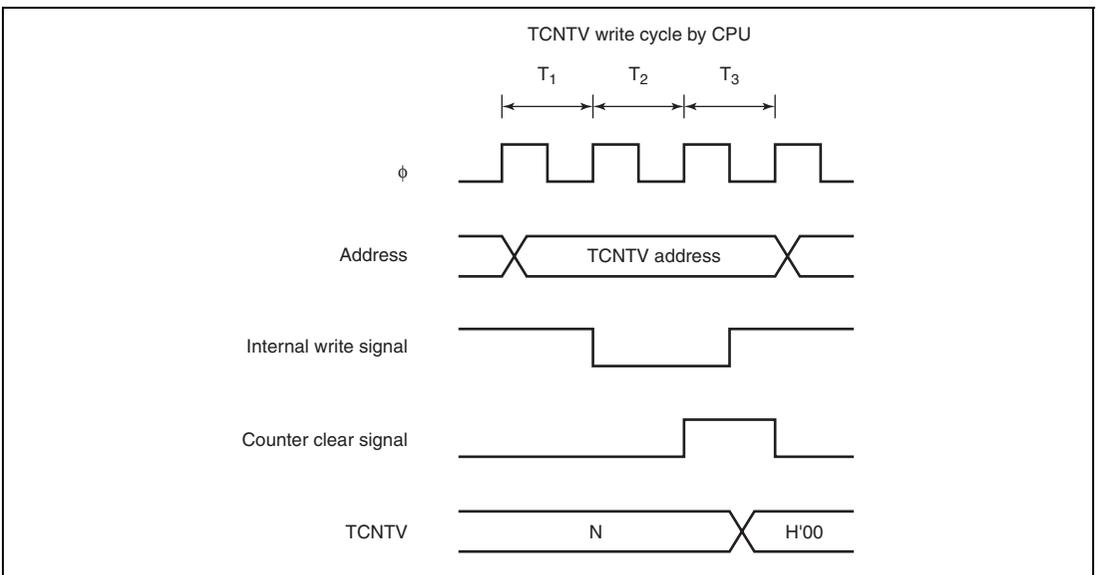
**Figure 12.11 Contention between TCNTV Write and Clear**
