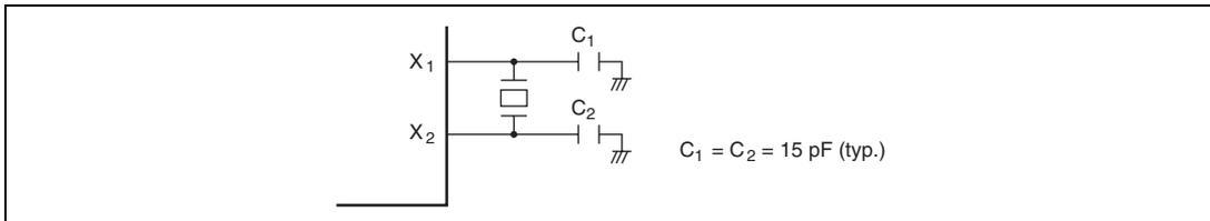
**Figure 5.8 Typical Connection to 32.768-kHz Crystal Resonator**
