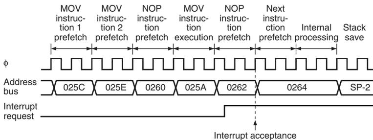
**Figure 4.2 Address Break Interrupt Operation Example (2)**
