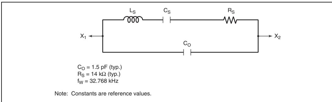
**Figure 5.9 Equivalent Circuit of 32.768-kHz Crystal Resonator**
