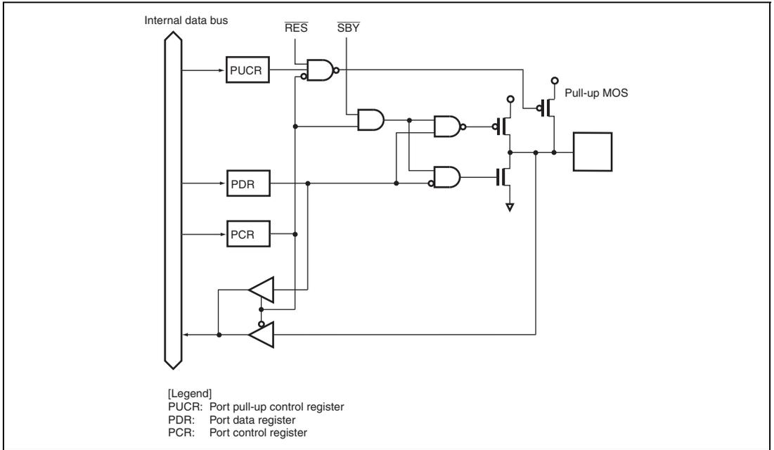
**Figure B.4 Port 1 Block Diagram (P12)**
