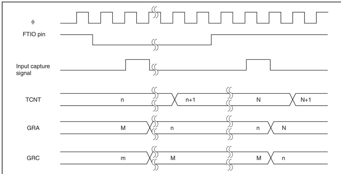
**Figure 13.41 Input Capture Timing of Buffer Operation**
