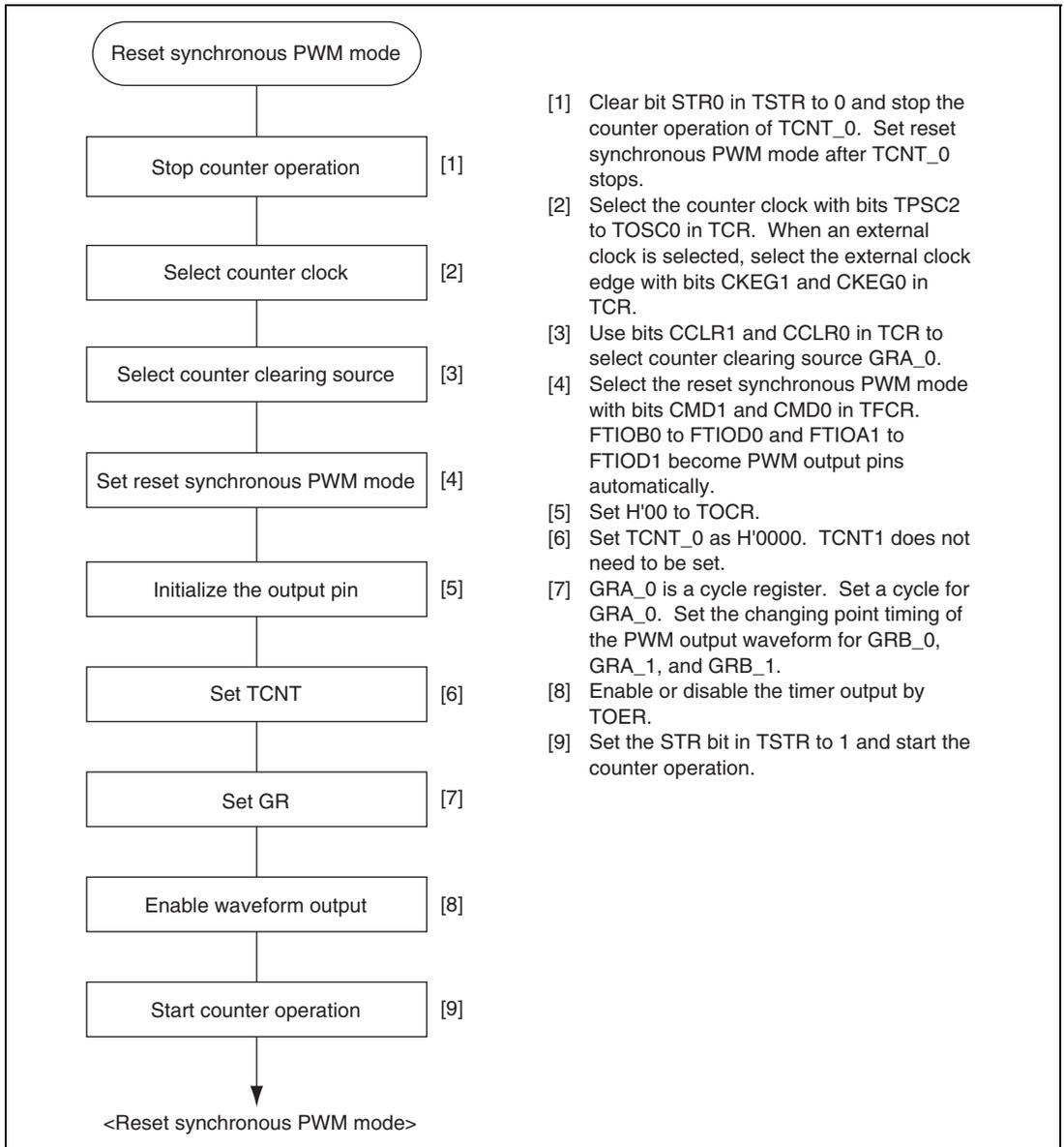
**Figure 13.26 Example of Reset Synchronous PWM Mode Setting Procedure**
