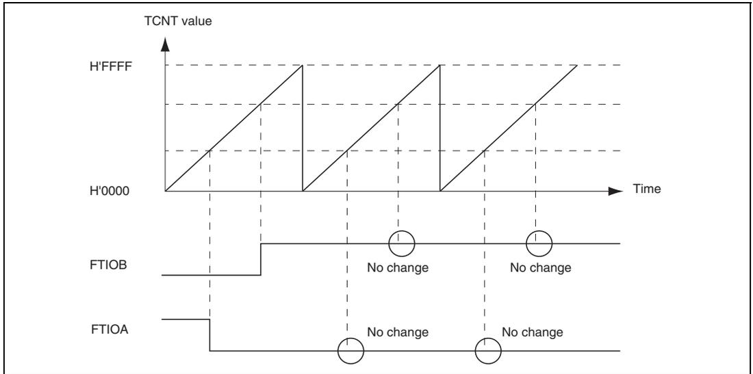
**Figure 13.13 Example of 0 Output/1 Output Operation**
