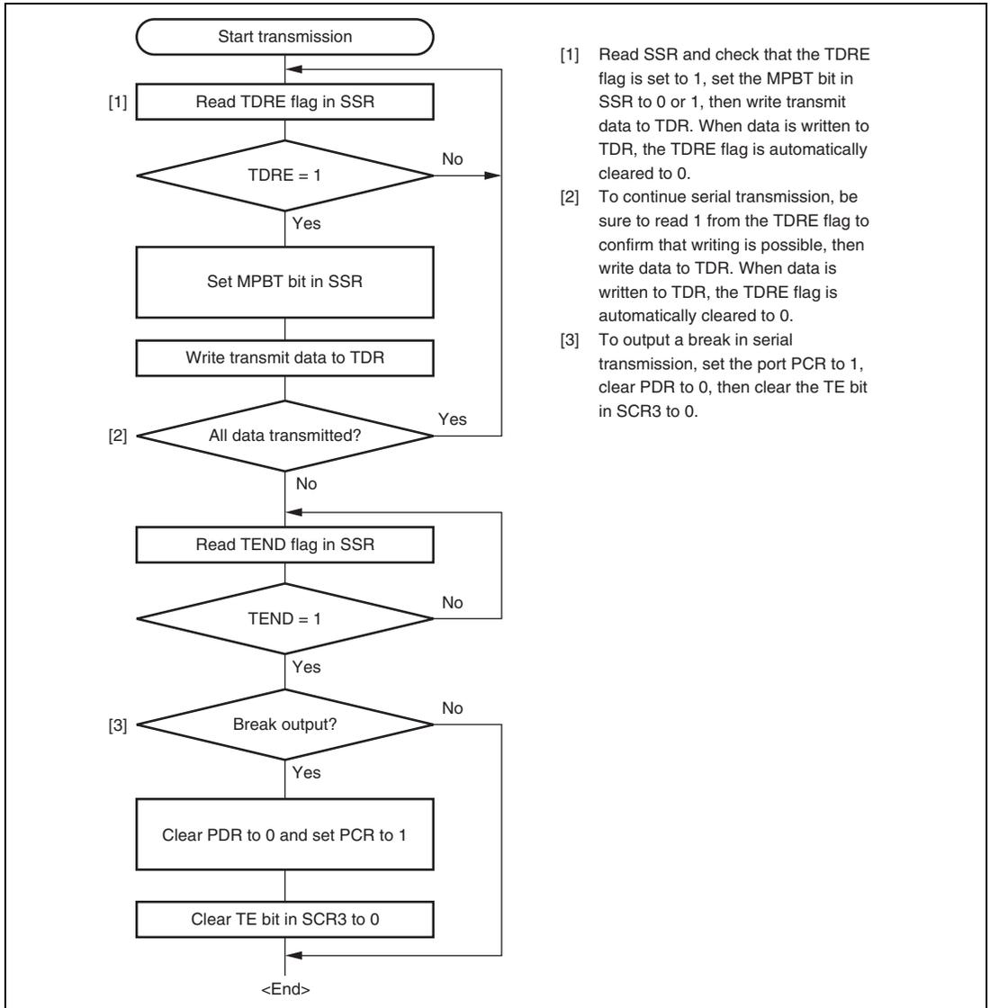
**Figure 16.16 Sample Multiprocessor Serial Transmission Flowchart**
