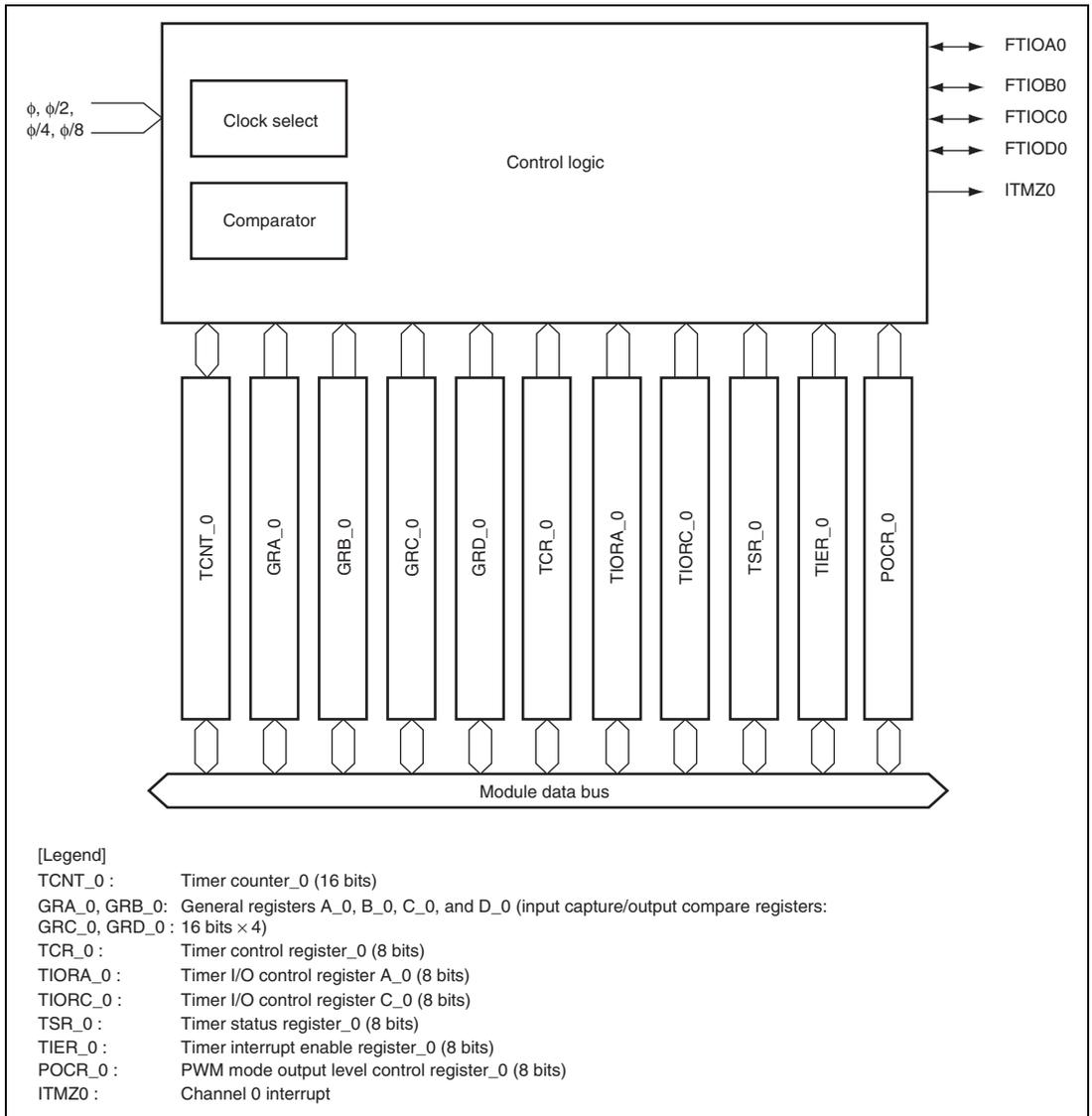
**Figure 13.2 Timer Z (Channel 0) Block Diagram**
