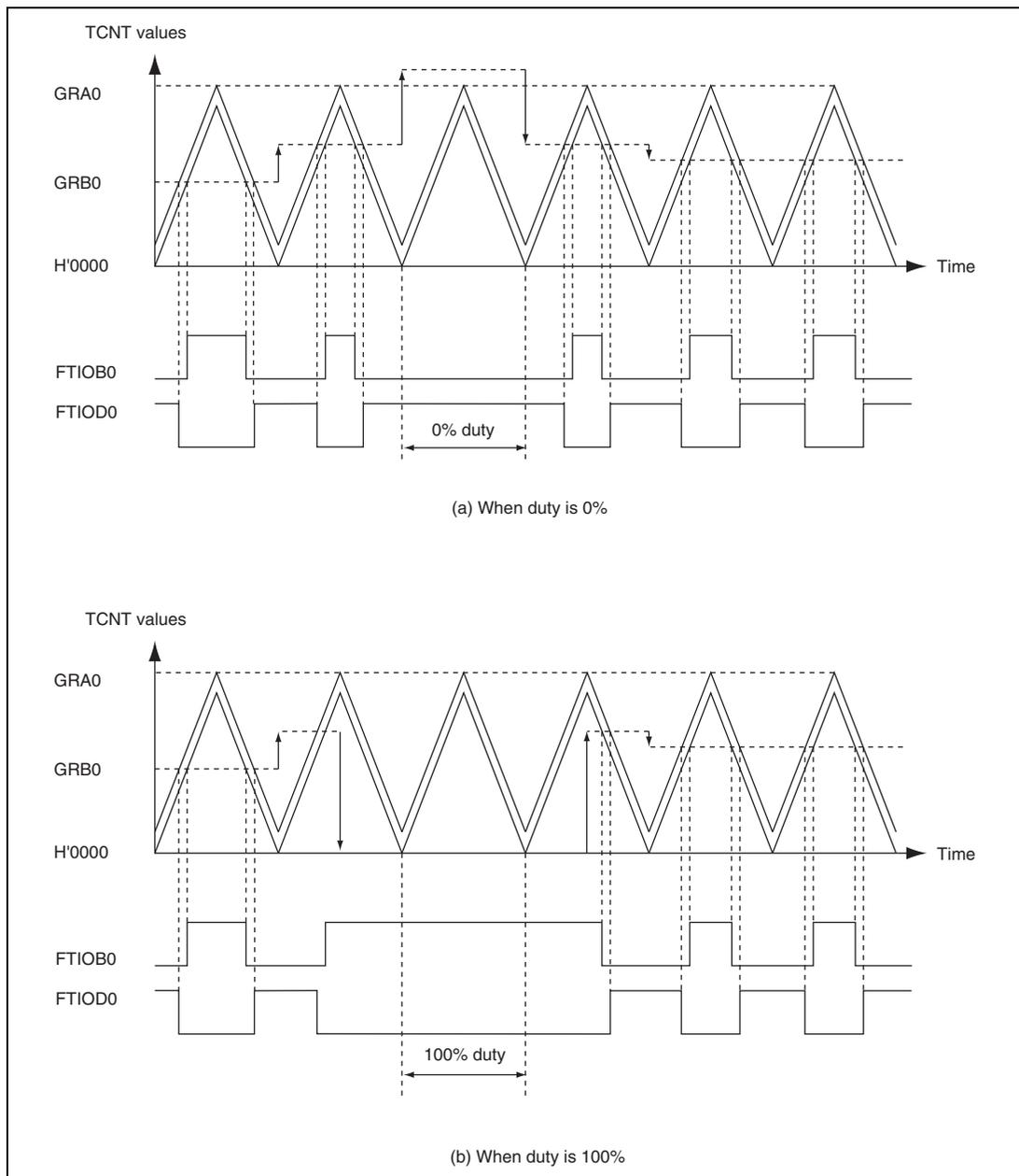
**Figure 13.32 (1) Example of Complementary PWM Mode Operation
