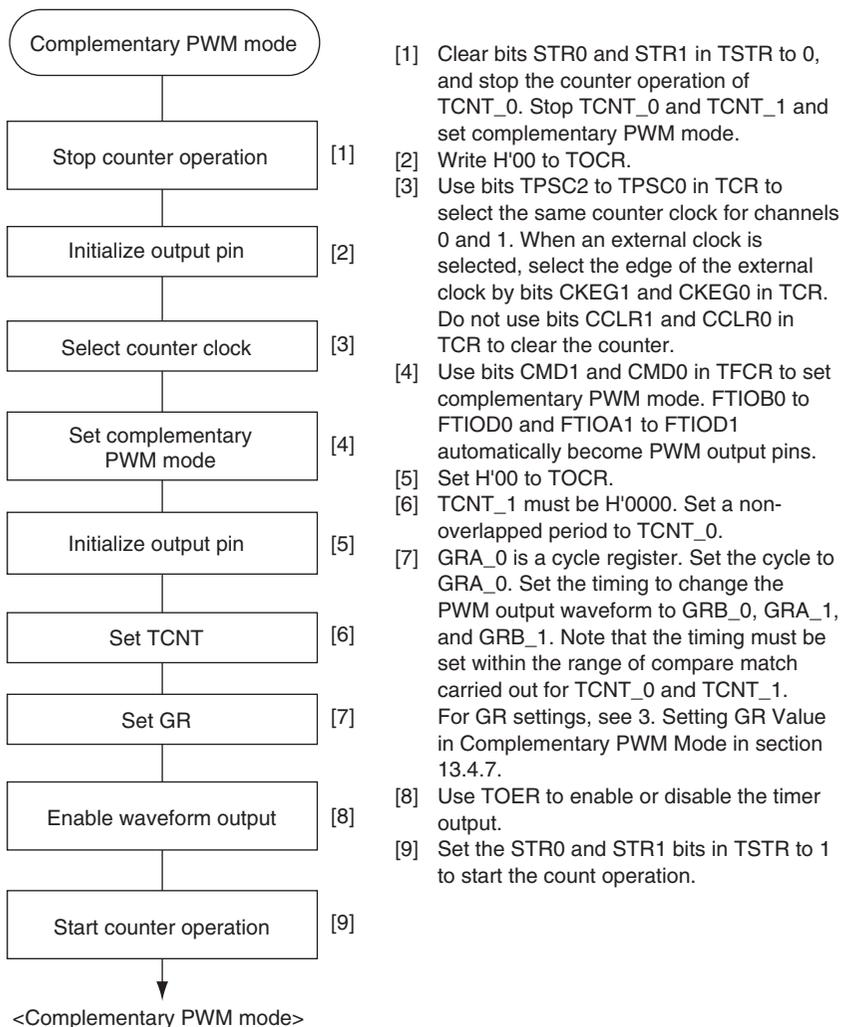
Note: To re-enter complementary PWM mode, first, enter a mode other than the complementary PWM mode. After that, repeat the setting procedures from step [1].
