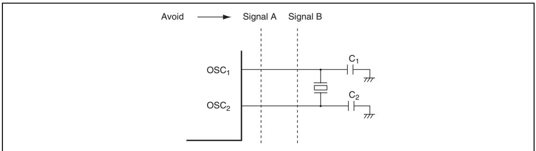
**Figure 5.11 Example of Incorrect Board Design**
