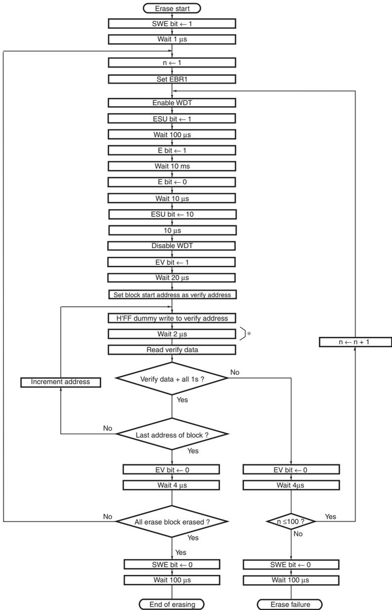
Note: \*The RTS instruction must not be used during a period between dummy writing of H'FF to a verify address and verify data reading.
