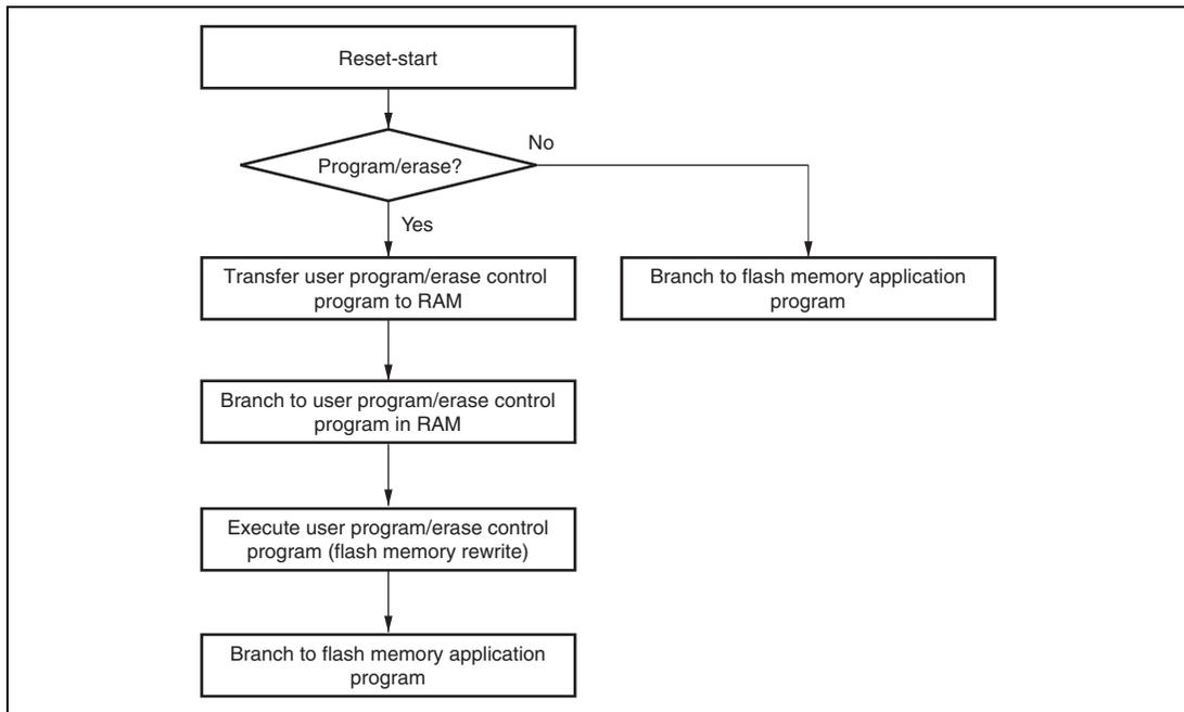
**Figure 7.2 Programming/Erasing Flowchart Example in User Program Mode**
