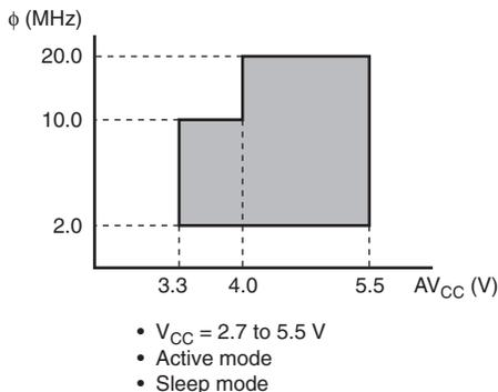
**Range of Power Supply Voltage and Oscillation Frequency when Low-Voltage Detection Circuit is Used**
