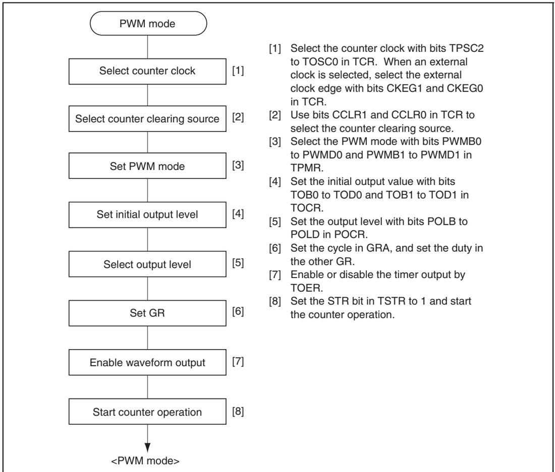
**Figure 13.21 Example of PWM Mode Setting Procedure**
