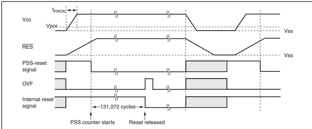
**Figure 20.2 Operational Timing of Power-On Reset Circuit**
