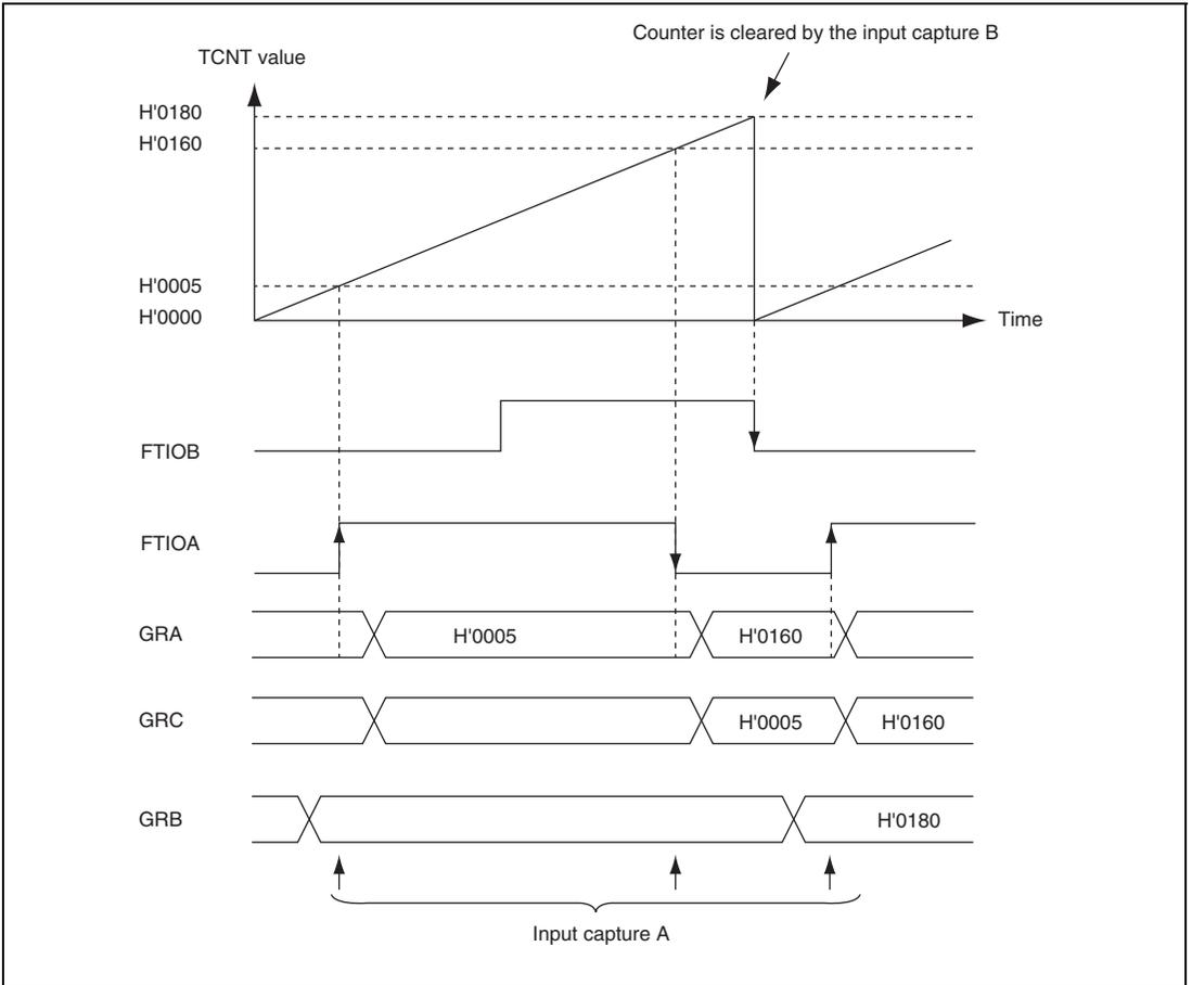
**Figure 13.40 Example of Buffer Operation (2)
