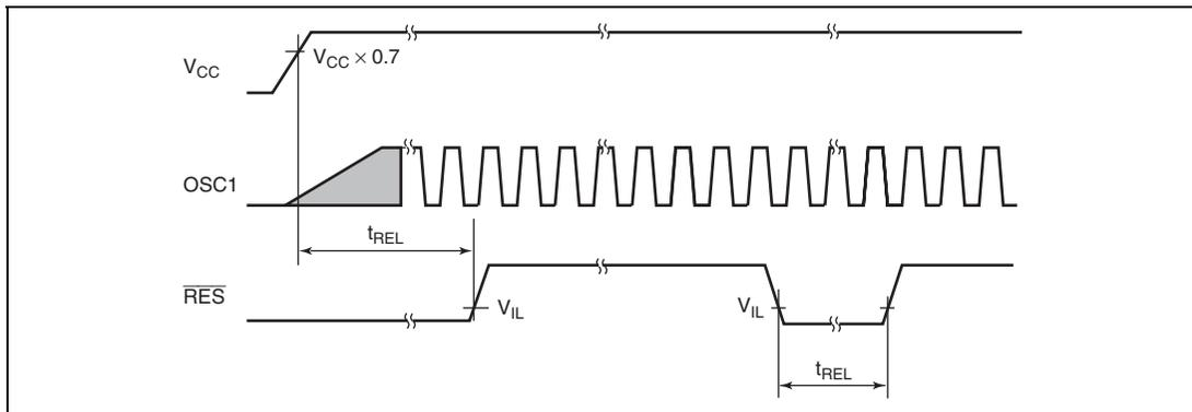
**Figure 23.2**  $\overline{\text{RES}}$  Low Width Timing
