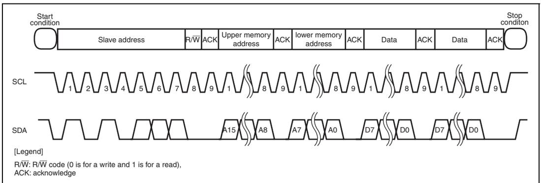
**Figure 19.2 EEPROM Bus Format and Bus Timing**
