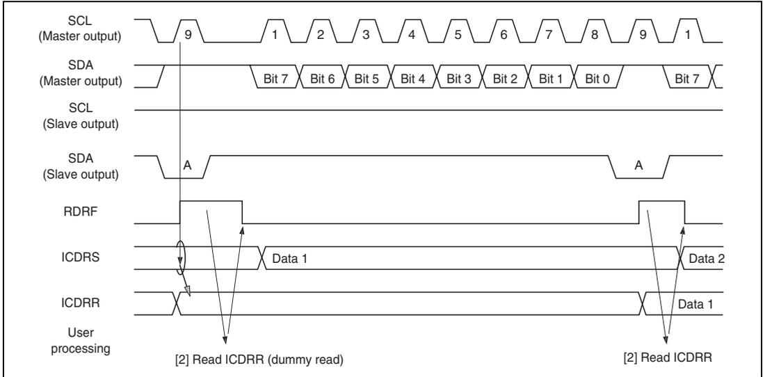
**Figure 17.11 Slave Receive Mode Operation Timing (1)**
