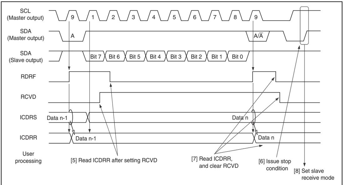
**Figure 17.8 Master Receive Mode Operation Timing (2)**
