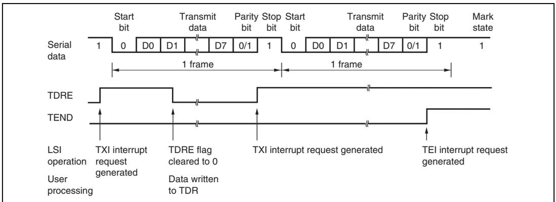
**Figure 16.5 Example of SCI3 Transmission in Asynchronous Mode
