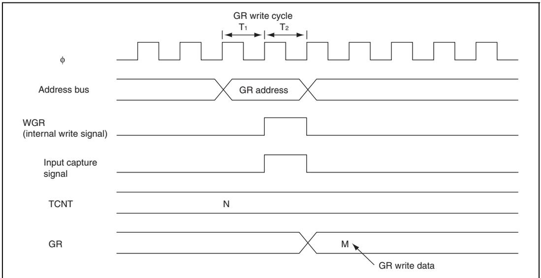
**Figure 13.58 Contention between GR Write and Input Capture**
