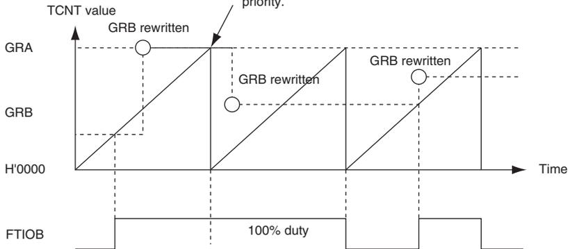
When cycle register and duty register compare matches occur simultaneously, duty register compare match has priority.
