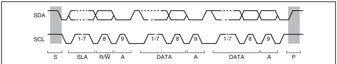
Figure 17.4 I<sup>2</sup>C Bus Timing
