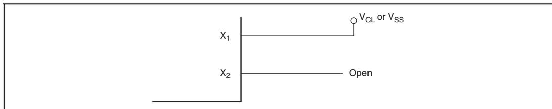
**Figure 5.10 Pin Connection when not Using Subclock**
