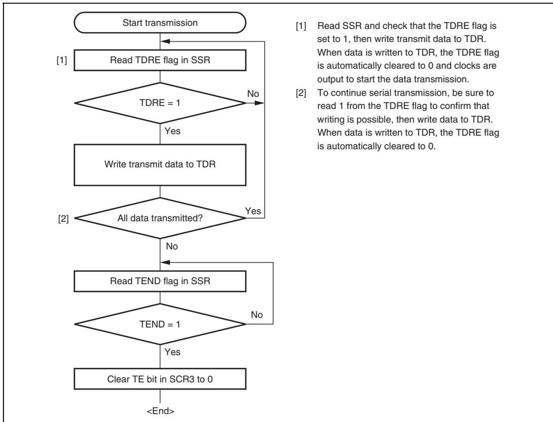
**Figure 16.11 Sample Serial Transmission Flowchart (Clocked Synchronous Mode)**
