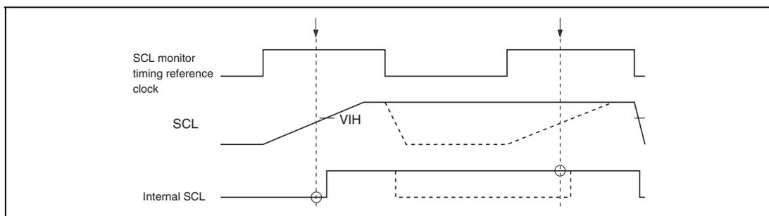
**Figure 17.21 The Timing of the Bit Synchronous Circuit**
