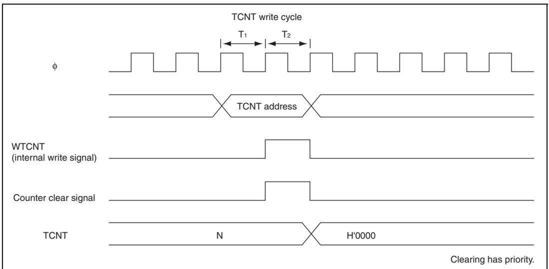
**Figure 13.52 Contention between TCNT Write and Clear Operations**
