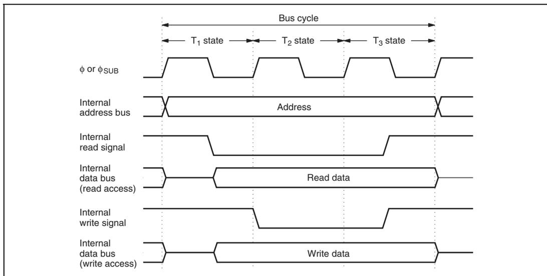
**Figure 2.10 On-Chip Peripheral Module Access Cycle (3-State Access)**
