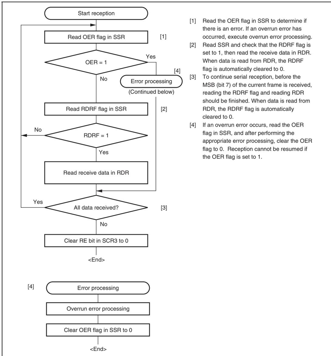
**Figure 16.13 Sample Serial Reception Flowchart (Clocked Synchronous Mode)**
