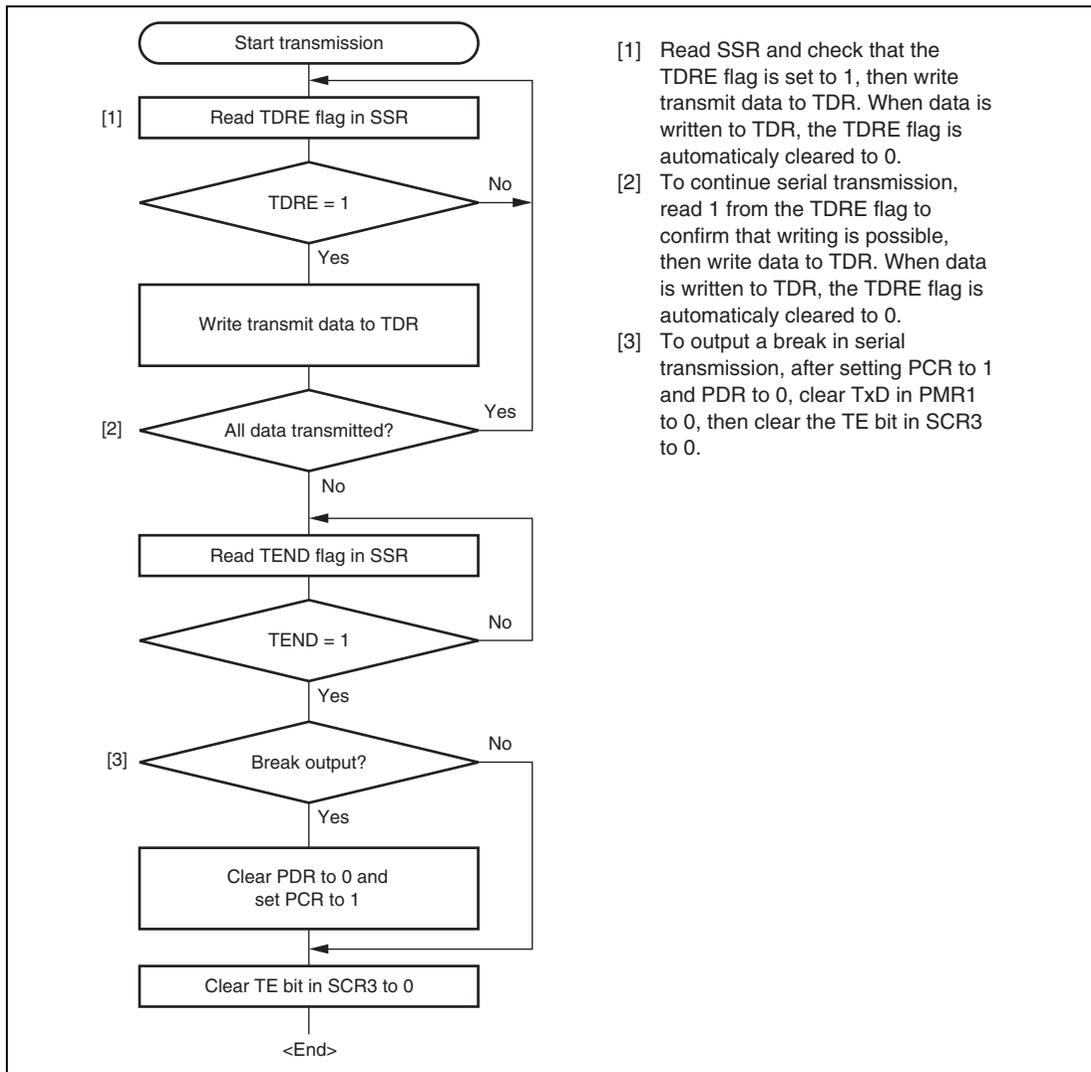
**Figure 16.6 Sample Serial Transmission Data Flowchart (Asynchronous Mode)**
