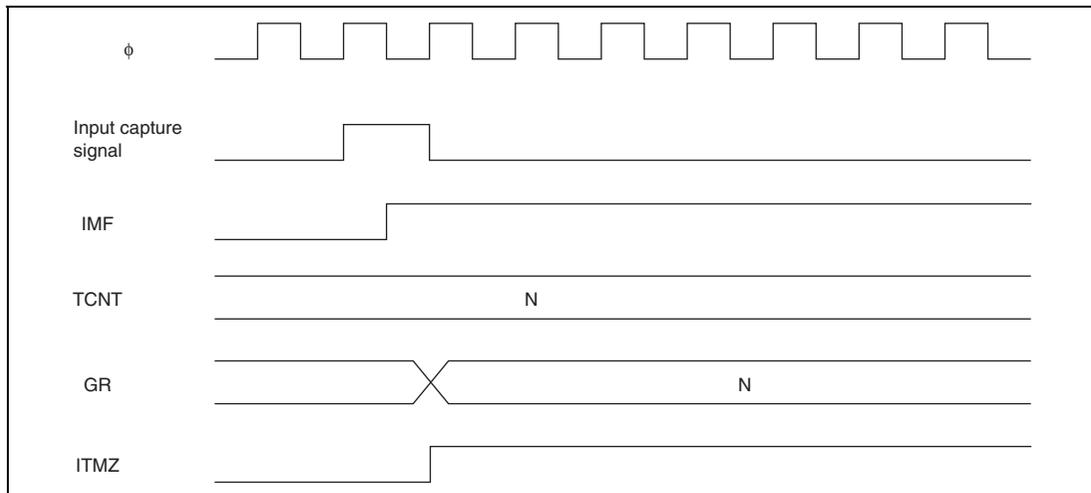
**Figure 13.49 IMF Flag Set Timing at Input Capture**
