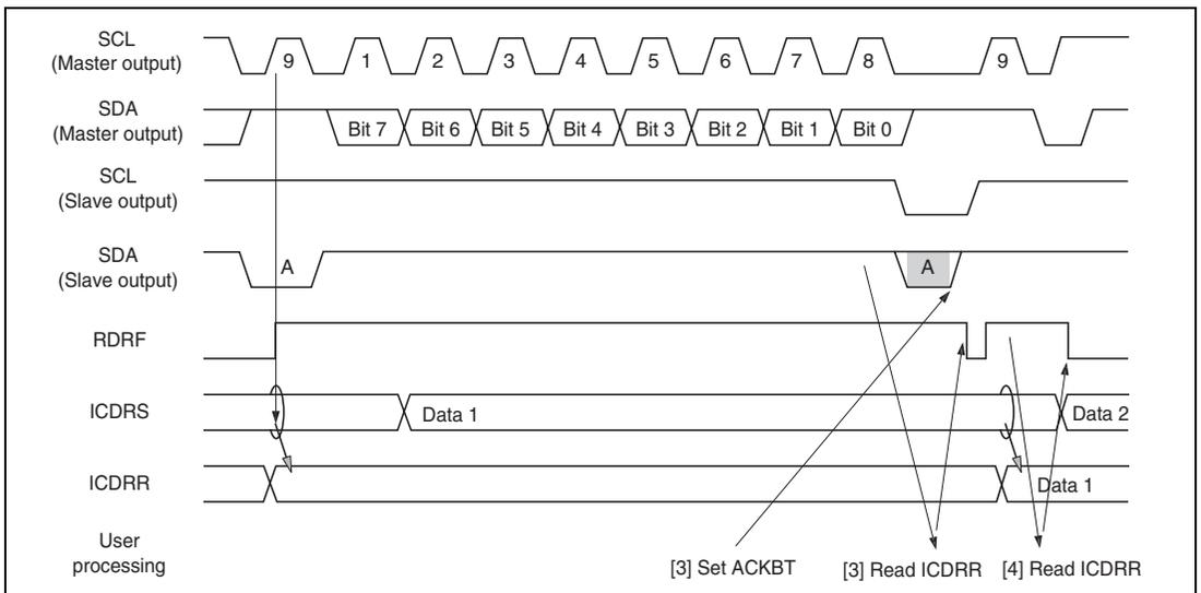
**Figure 17.12 Slave Receive Mode Operation Timing (2)**
