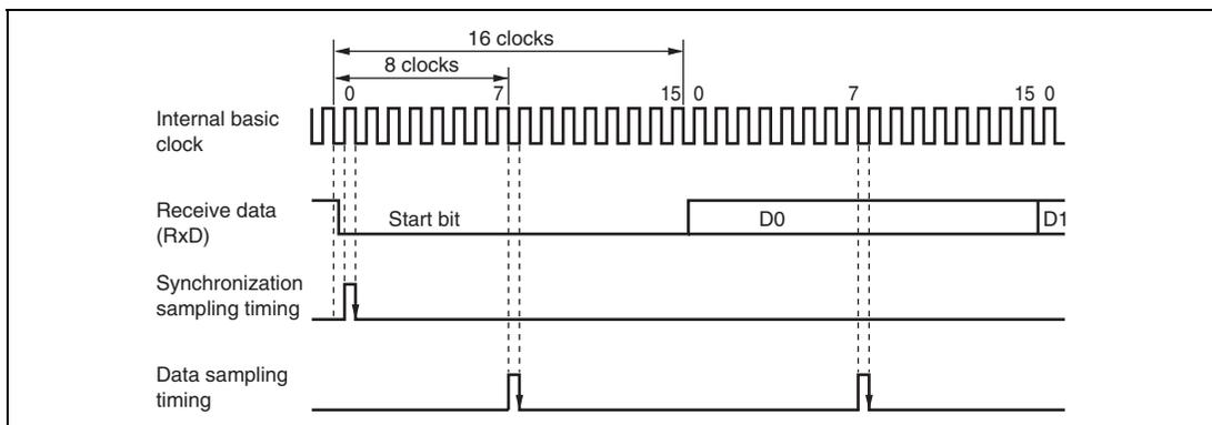
**Figure 16.19 Receive Data Sampling Timing in Asynchronous Mode**
