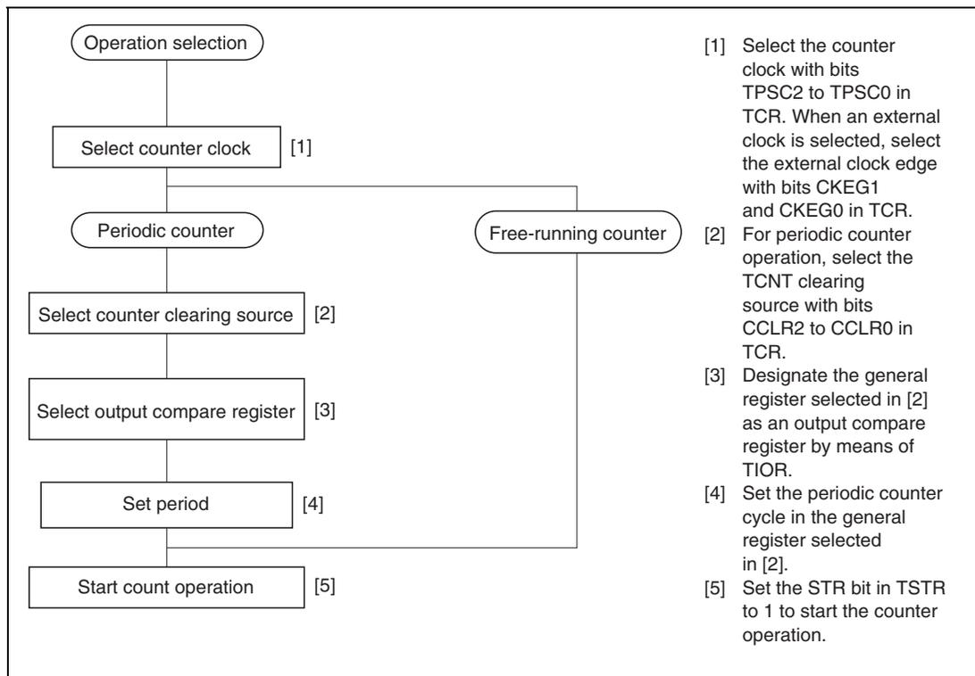
**Figure 13.7 Example of Counter Operation Setting Procedure**
