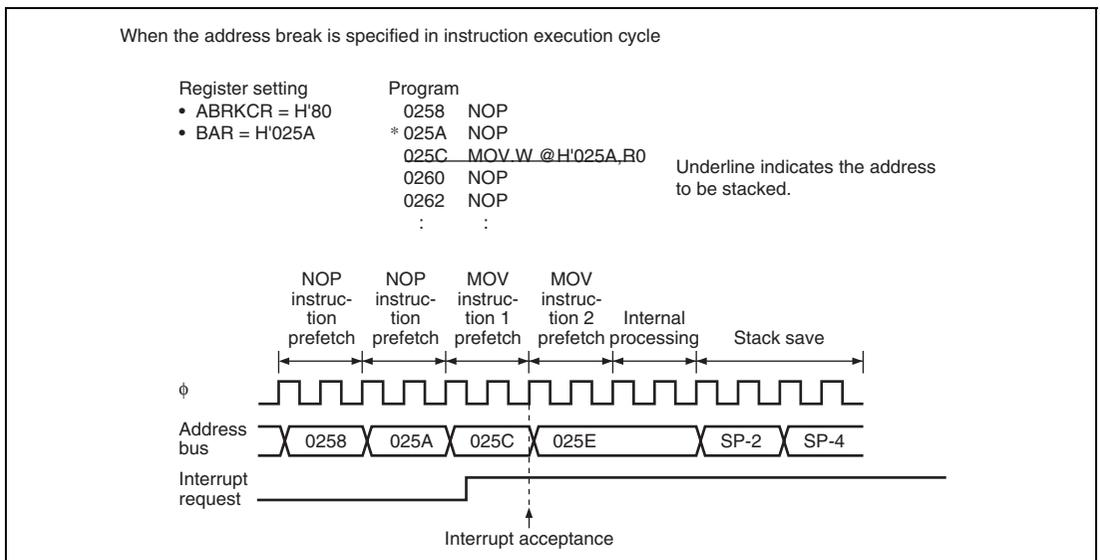
**Figure 4.2 Address Break Interrupt Operation Example (1)**
