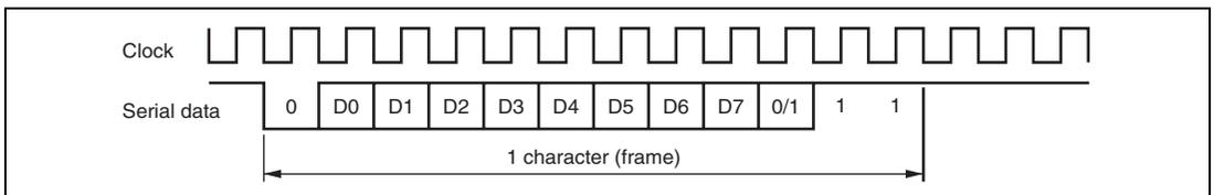
**Figure 16.3 Relationship between Output Clock and Transfer Data Phase (Asynchronous Mode) (Example with 8-Bit Data, Parity, Two Stop Bits)**
