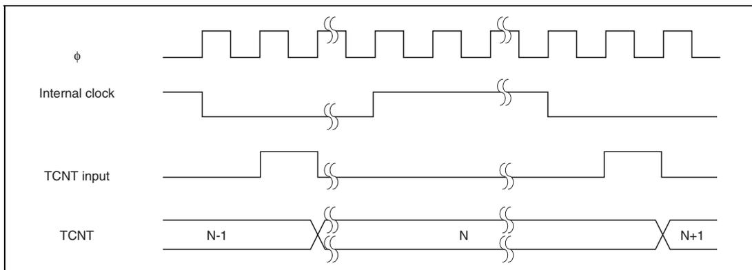
**Figure 13.10 Count Timing at Internal Clock Operation**
