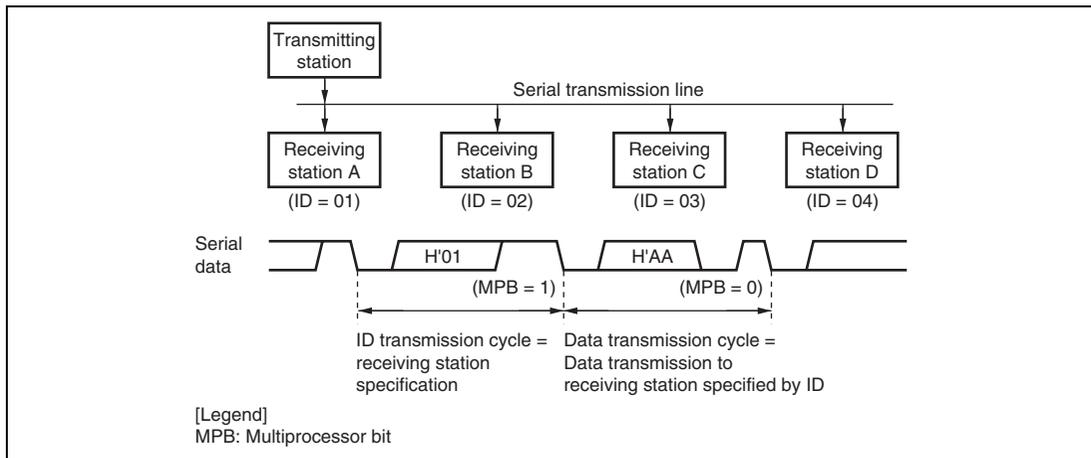
**Figure 16.15 Example of Inter-Processor Communication Using Multiprocessor Format
