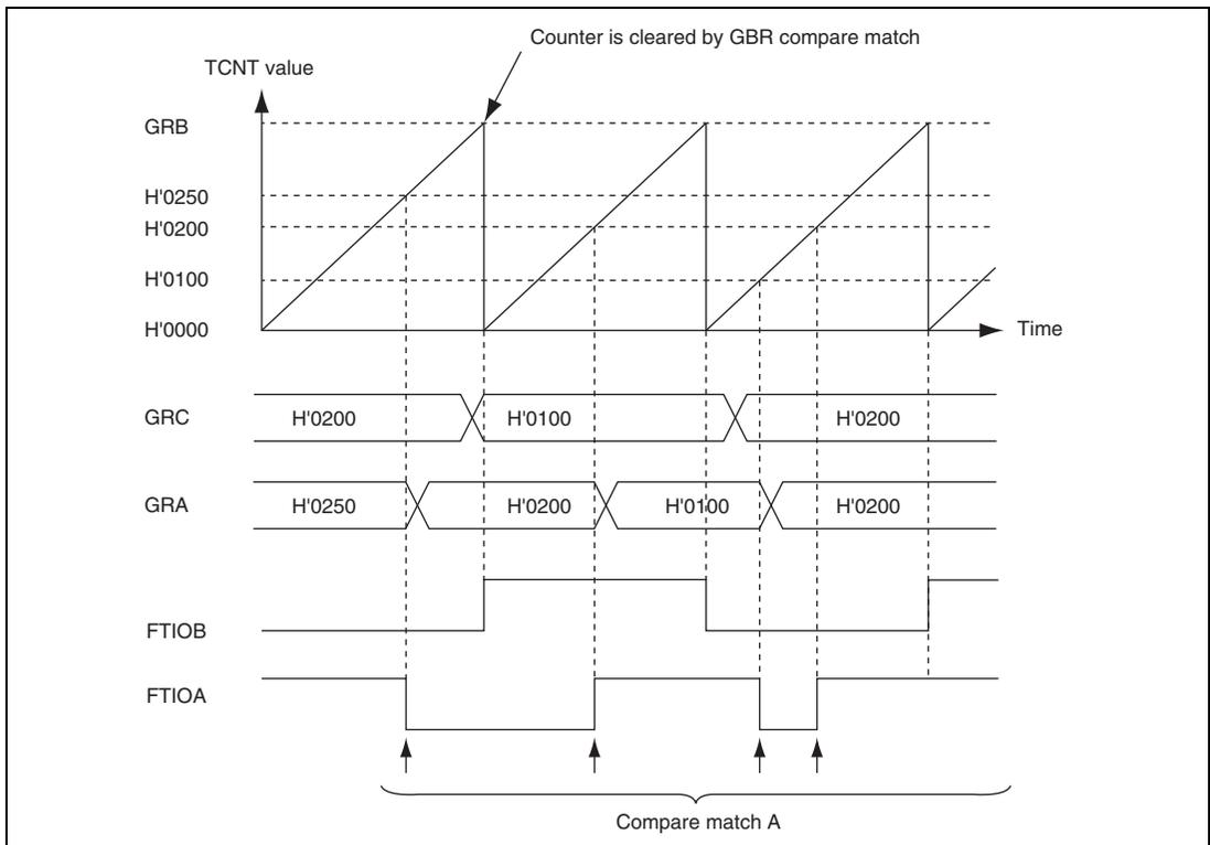
**Figure 13.38 Example of Buffer Operation (1)
