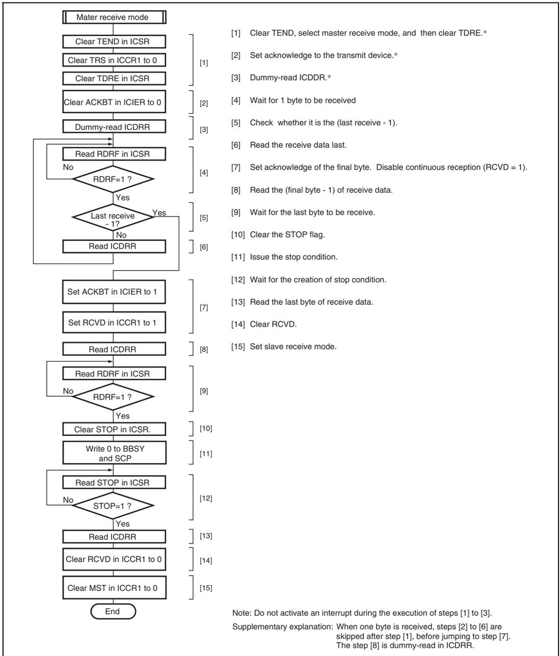
Figure 17.18 Sample Flowchart for Master Receive Mode
