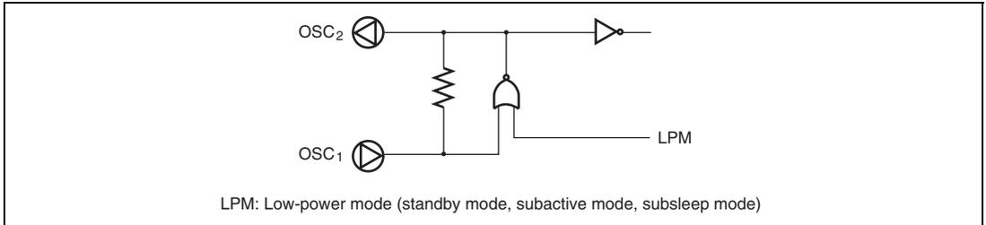
**Figure 5.2 Block Diagram of System Clock Generator**
