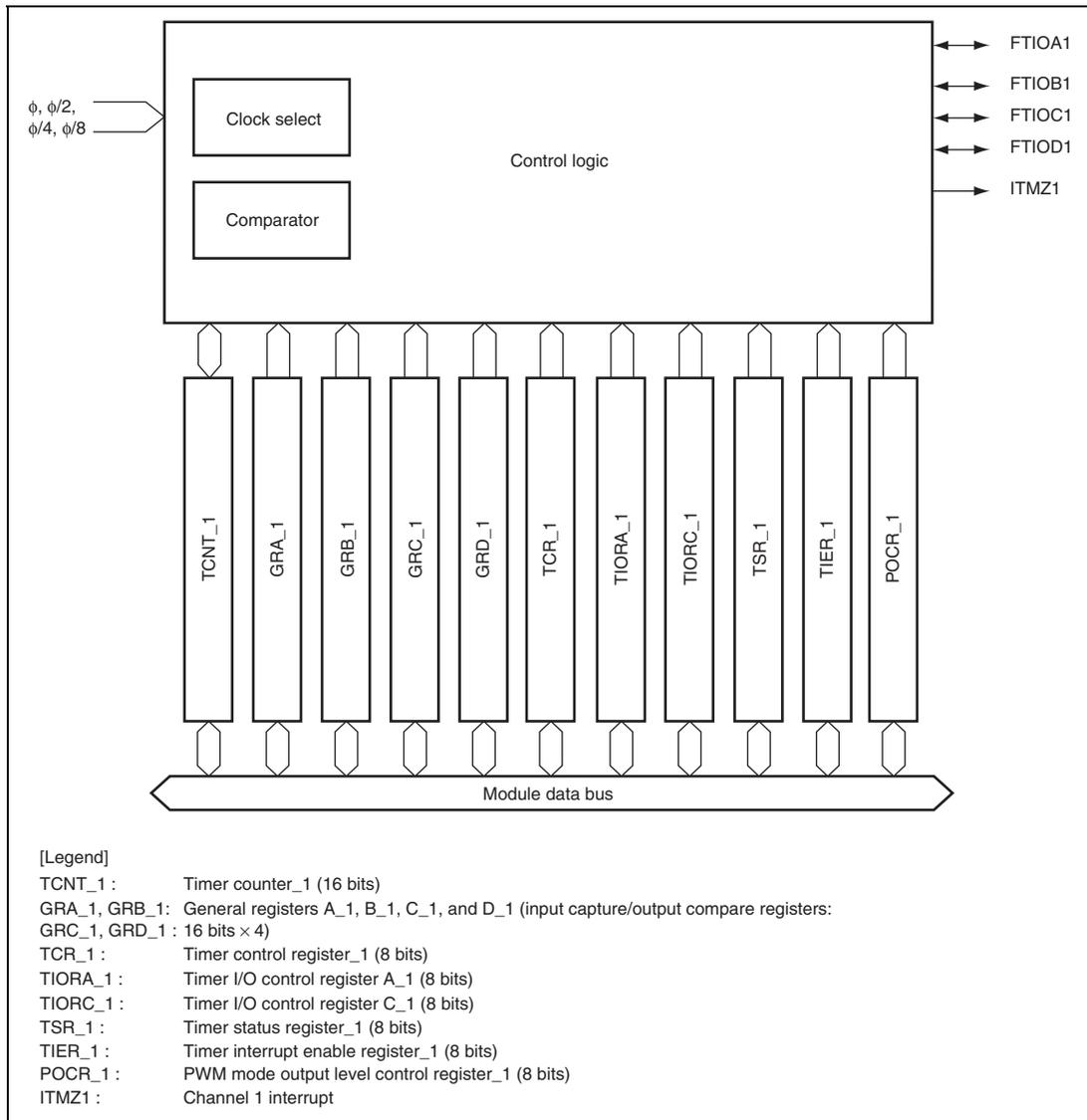
**Figure 13.3 Timer Z (Channel 1) Block Diagram**
