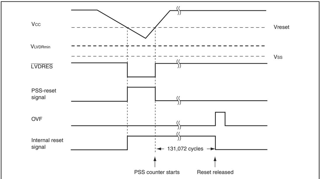
**Figure 20.3 Operational Timing of LVDR Circuit**
