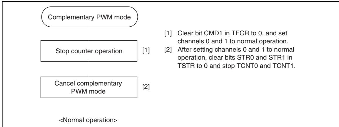
**Figure 13.30 Canceling Procedure of Complementary PWM Mode**
