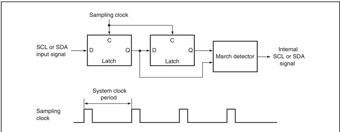
**Figure 17.16 Block Diagram of Noise Canceler**
