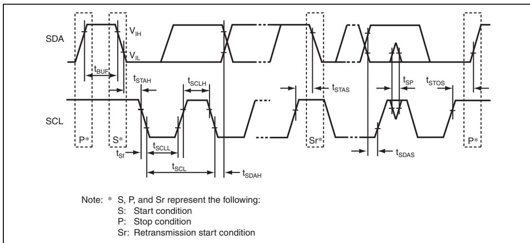
**Figure 23.4** I<sup>2</sup>C Bus Interface Input/Output Timing
