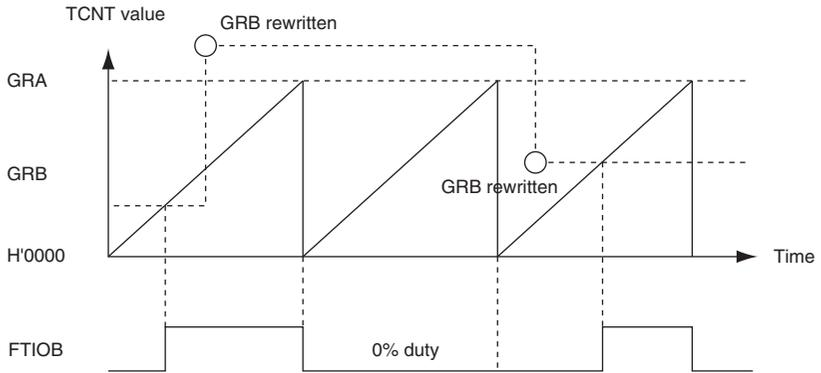
When cycle register and duty register compare matches occur simultaneously, duty register compare match has priority.
