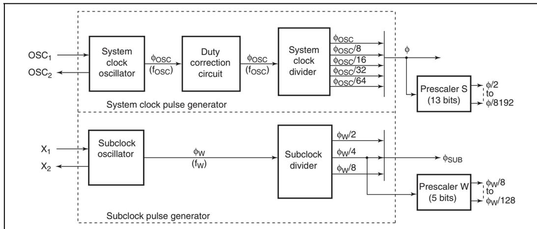
**Figure 5.1 Block Diagram of Clock Pulse Generators**
