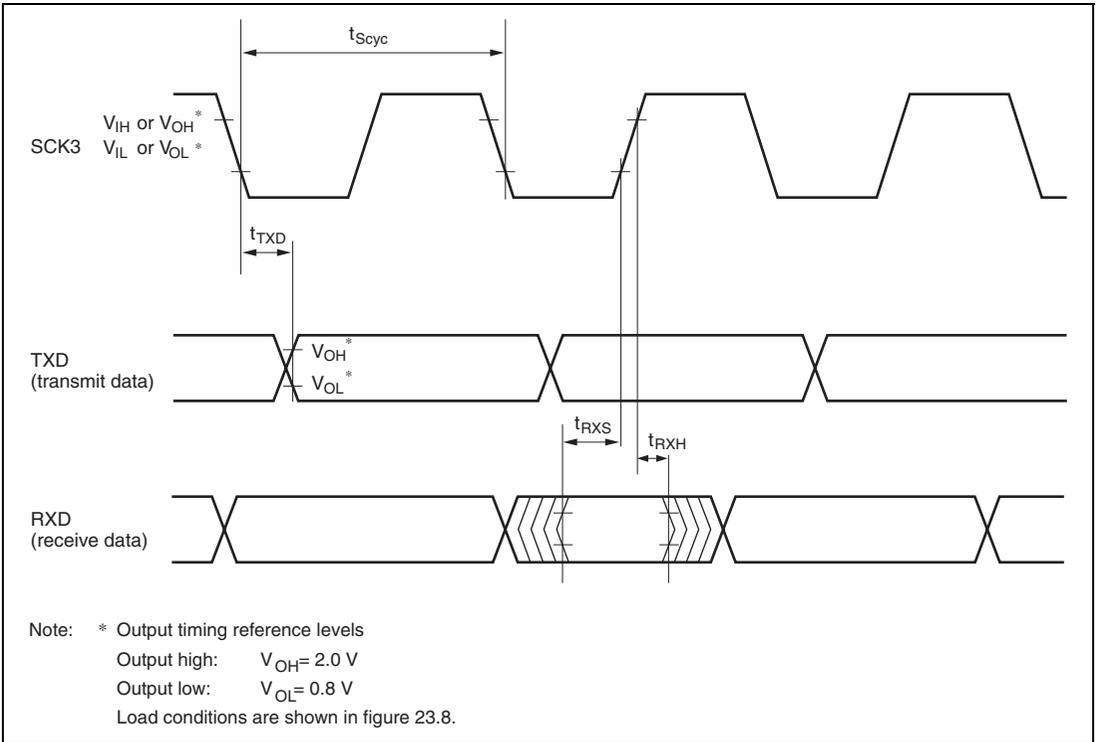
**Figure 23.6 SCI Input/Output Timing in Clocked Synchronous Mode**
