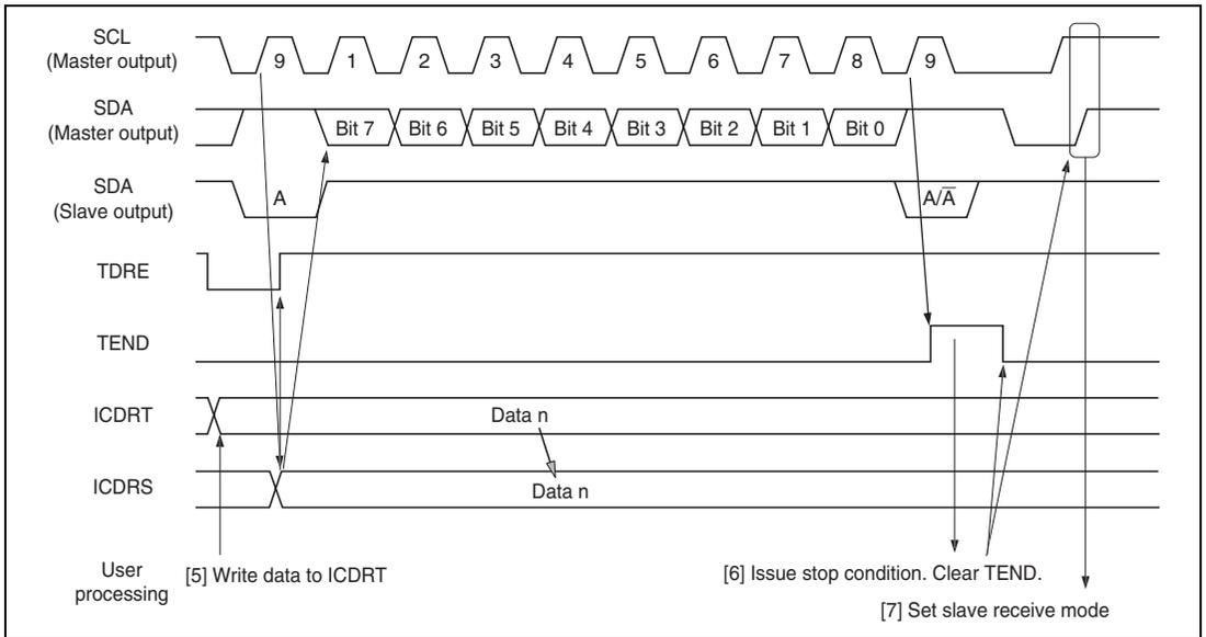
**Figure 17.6 Master Transmit Mode Operation Timing (2)**
