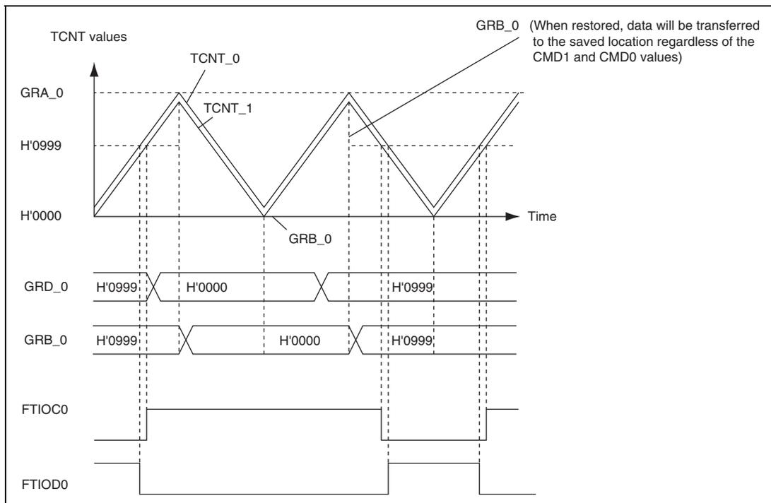
**Figure 13.43 Buffer Operation (4)**
