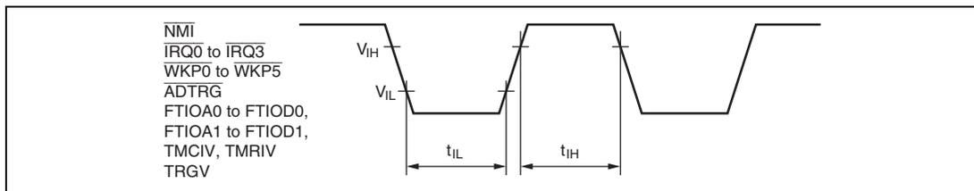
**Figure 23.3** Input Timing
