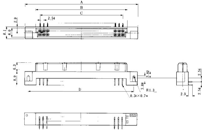
\*Type Q differs in the external size and PCB mounting pattern.
