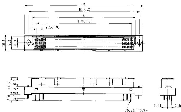
Note: The PCB mounting pattern is equivalent to PCN10-\*S-2.54DSA(72).
