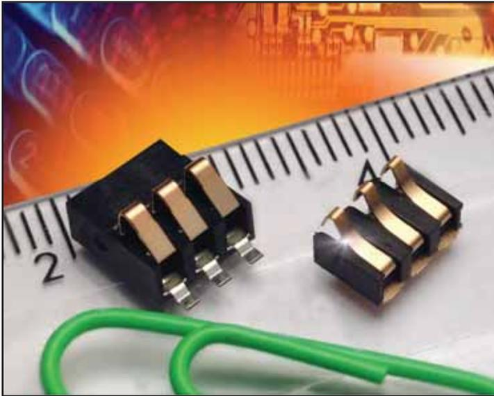
The newest product in AVX's Interconnect family of battery connectors saves 50% in volume over the initial 9155 series compression connectors as illustrated in the photograph. These connectors are rated at a full 3 amps per contact on 2.5mm centers. Sizes range from 2 positions through 5 positions and are end to end stackable.
