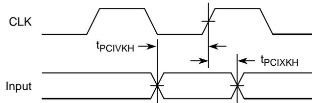
**Figure 37. PCI Input AC Timing Measurement Conditions**
