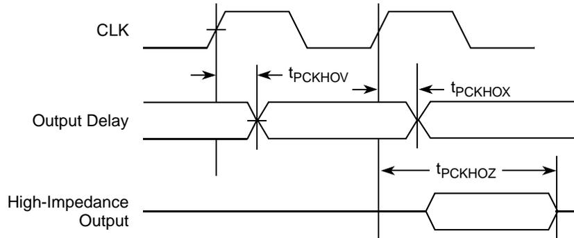
**Figure 38. PCI Output AC Timing Measurement Condition**
