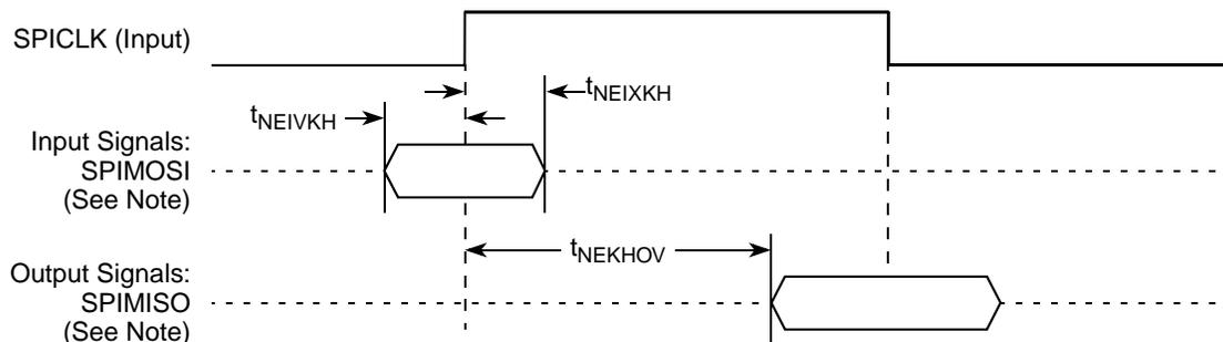
**Note:** The clock edge is selectable on SPI.
