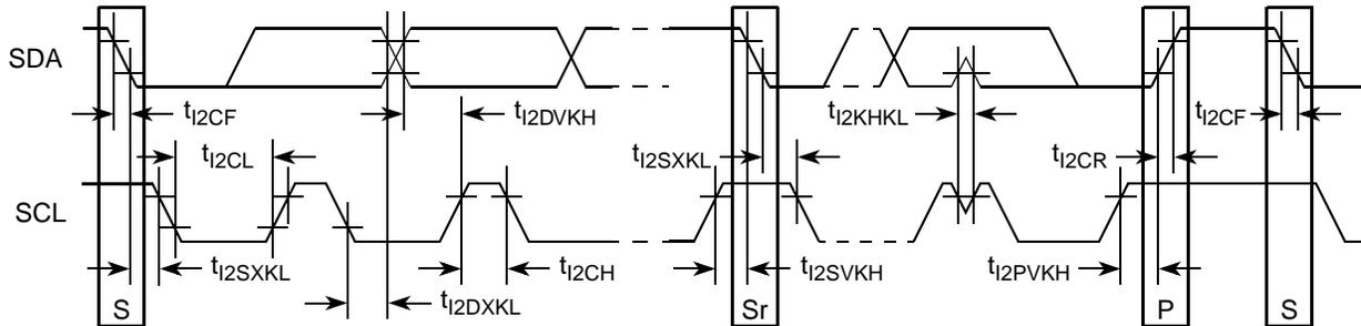
Figure 35. I<sup>2</sup>C Bus AC Timing Diagram
