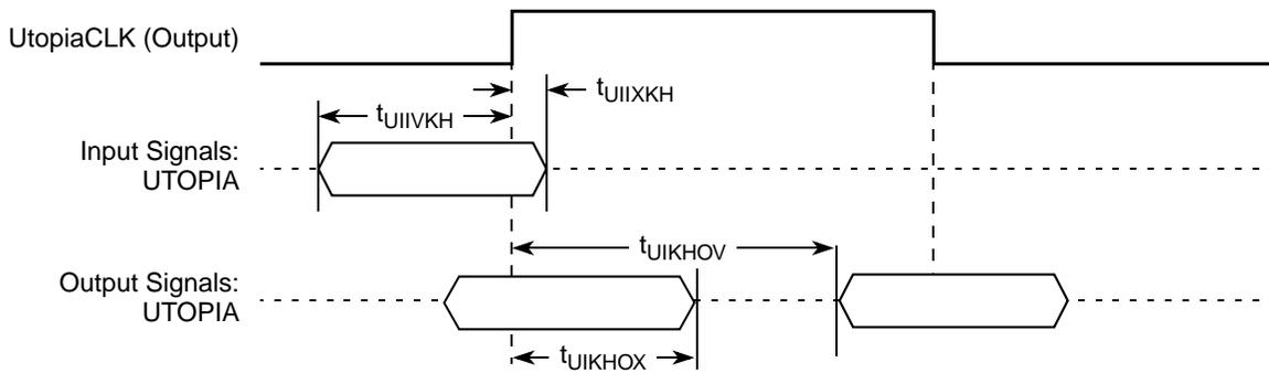
Figure 48. UTOPIA AC Timing (Internal Clock) Diagram
