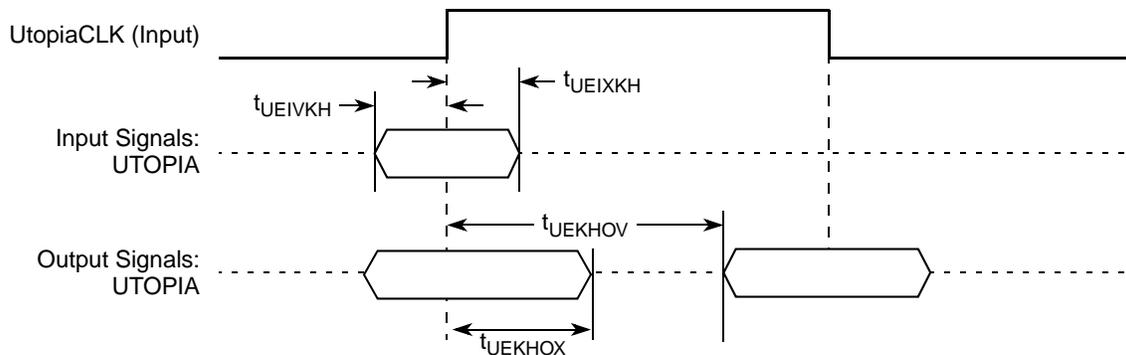
**Figure 47. UTOPIA AC Timing (External Clock) Diagram**
