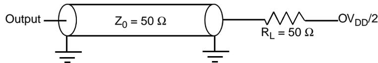
Figure 34. I<sup>2</sup>C AC Test Load
