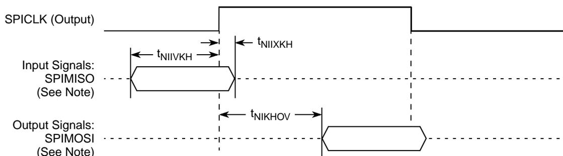
**Note:** The clock edge is selectable on SPI.
