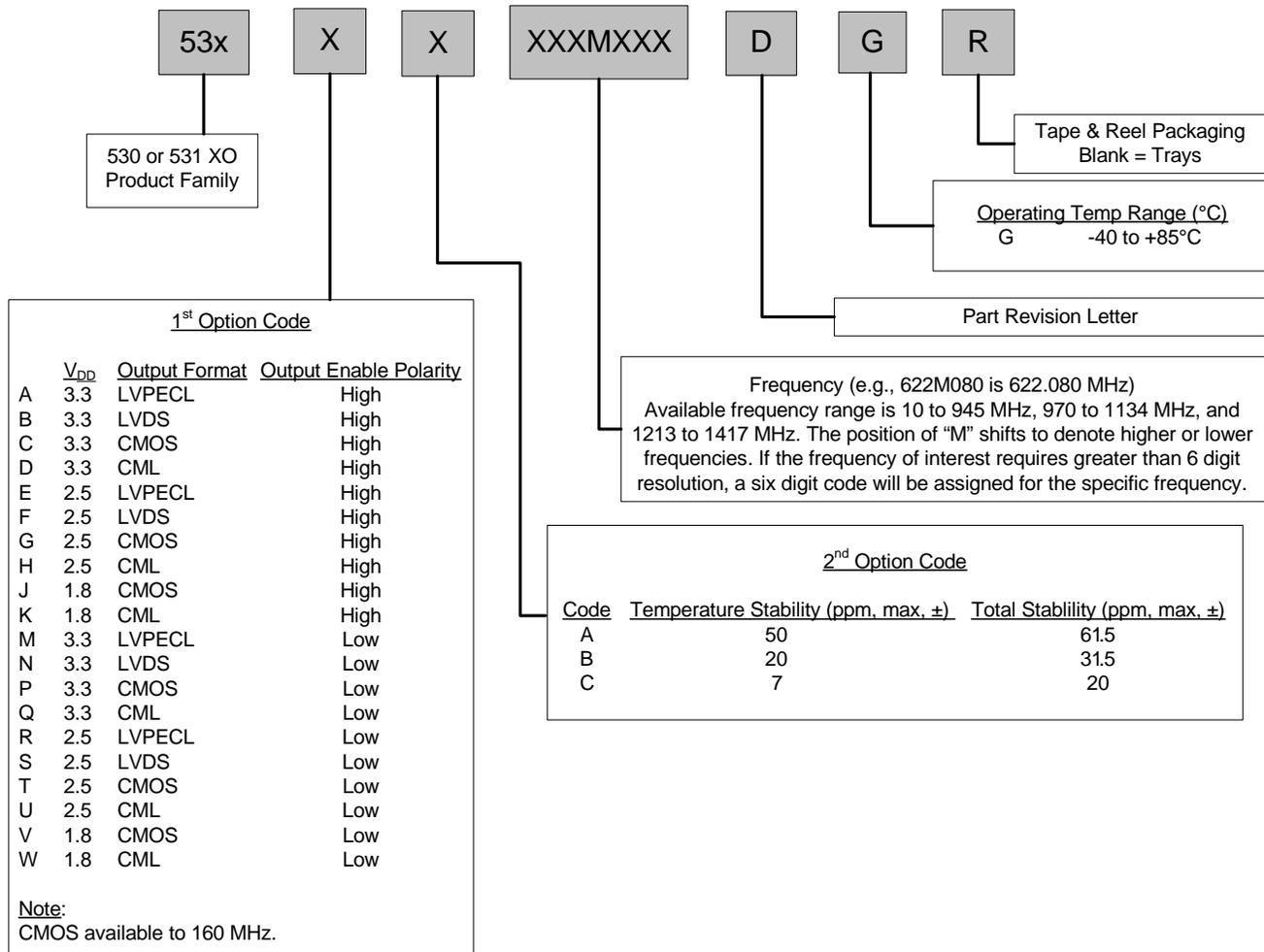
Example P/N: 530AB622M080DGR is a 5 x 7 XO in a 6 pad package. The frequency is 622.080 MHz, with a 3.3 V supply, LVPECL output, and Output Enable active high polarity. Temperature stability is specified as  $\pm 20$  ppm. The part is specified for  $-40$  to  $+85$  °C ambient temperature range operation and is shipped in tape and reel format.
