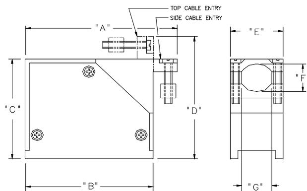
NEW COVER DESIGN (AVAILABLE SOON) WILL ELIMINATE 3 SCREWS FOR SIDE TO SIMPLIFY ASSEMBLY. DISASSEMBLY AND CLAMP ORIENTATION CHANGES.
