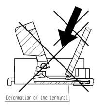
3. Do not rotate the actuator when FFC TAB is on right and left guides for positioning FFC. Make sure the position of FFC TAB and guides before rotate the actuator.
