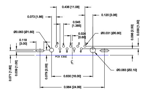
$\frac{P.C.B. LAY \square UT}{\text{TOLERANCE} = \pm 0.002 [\pm 0.05]}$  SCALE = 2:1
