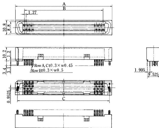
◆ PCB mounting pattern Applicable board thickness t=1.6mm
