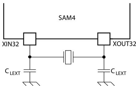
$$C_{LEXT} = 2X(C_{CRYSTAL} - C_{para} - C_{PCB}).$$
