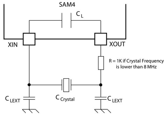
$$C_{LEXT} = 2 \times (C_{CRYSTAL} - C_L - C_{PCB}).$$
