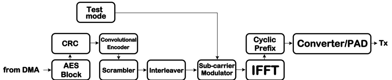
The output is differentially modulated using a BPSK/DQPSK/D8PSK scheme. After modulation, IFFT (Inverse Fourier Transform) block and cyclic prefix block allows to implement an OFDM scheme.
