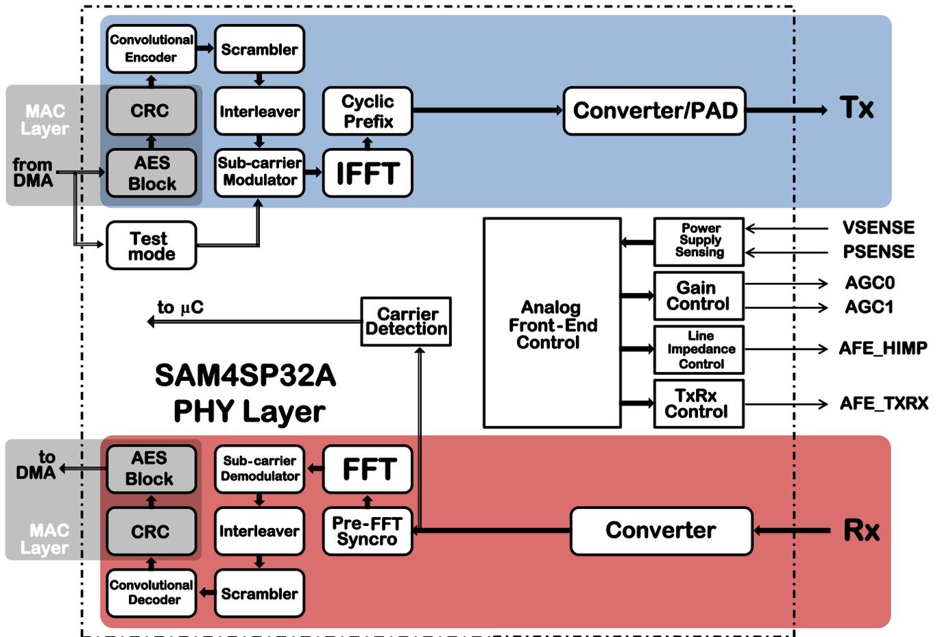
The diagram can be divided in four sub-blocks: Transmission branch, Emission branch, Analog Front End control and Carrier Detection.
