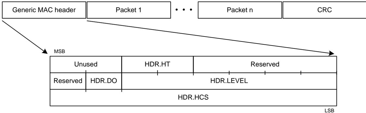
In transmission all CRC bytes are real-time calculated and the last bytes of the MAC PDU are overwritten with these values, (provided that the field HT in the first byte of the MAC header in transmission data is equal to the corresponding MAC PDU type).
