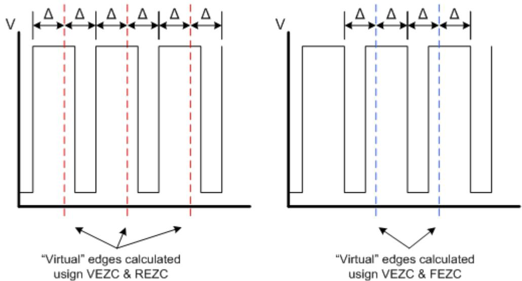
VEZC can be used simultaneously with REZC or FEZC.
