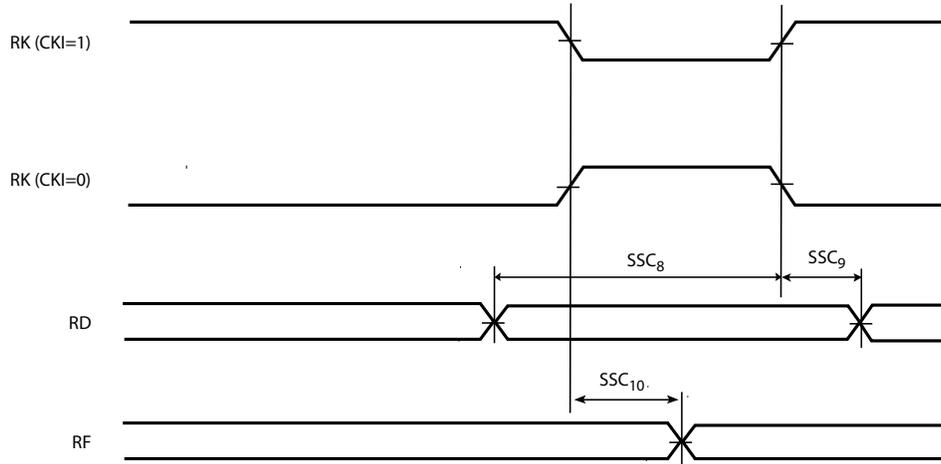
**Figure 13-16. SSC Receiver, RK and RF as output**
