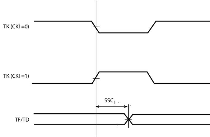
**Figure 13-12. SSC Transmitter, TK as output and TF as input**
