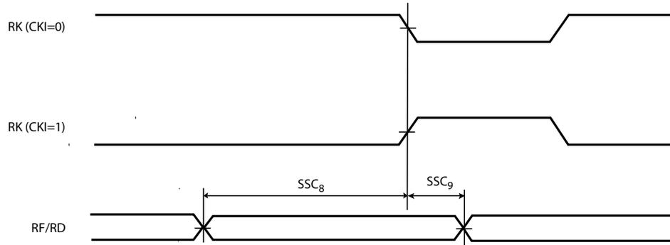
**Figure 13-15. SSC Receiver, RK as input and RF as output**
