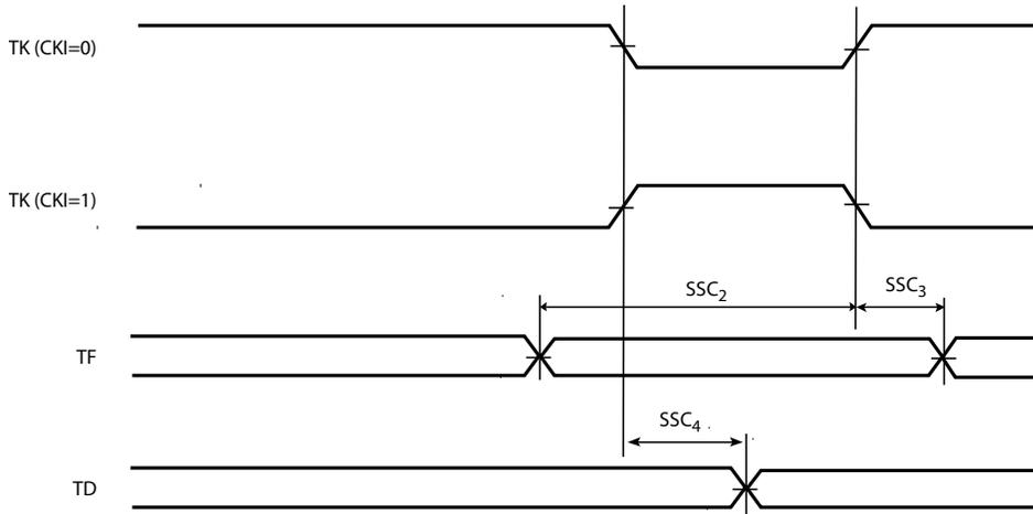
**Figure 13-13. SSC Transmitter, TK and TF as input**
