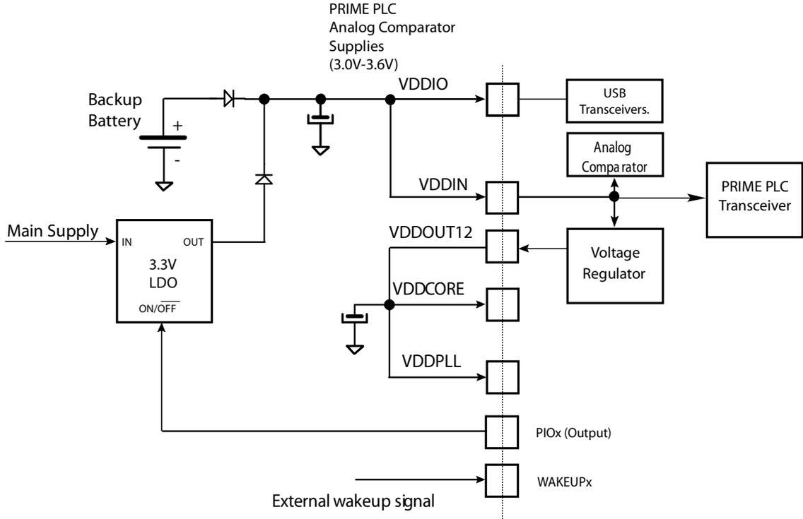
Note: The two diodes provide a "switchover circuit" (for illustration purpose) between the backup battery and the main supply when the system is put in backup mode.
