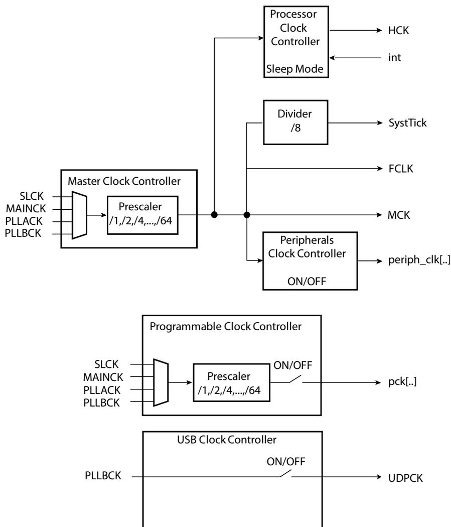
The SysTick calibration value is fixed at 12500, which allows the generation of a time base of 1 ms with SysTick clock at 12.5 MHz (max HCLK/8 = 100 MHz/8 = 12500, so STCALIB = 0x30D4).
