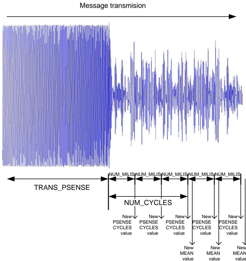
Psense and Vsense configurations parameters are automatically set by the Phy layer.
