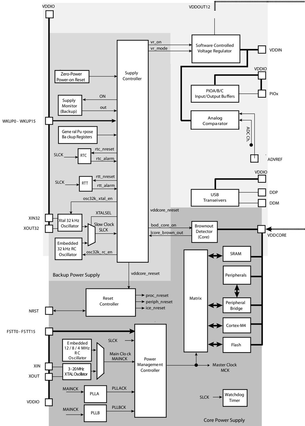
FSTT0 - FSTT15 are possible Fast Startup sources, generated by WKUP0 - WKUP15 pins, but are not physical pins.
