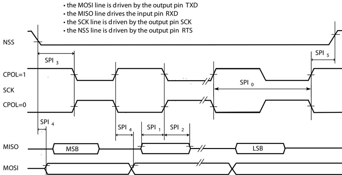
**Figure 13-22. USART SPI Slave Mode: (Mode 1 or 2)**
