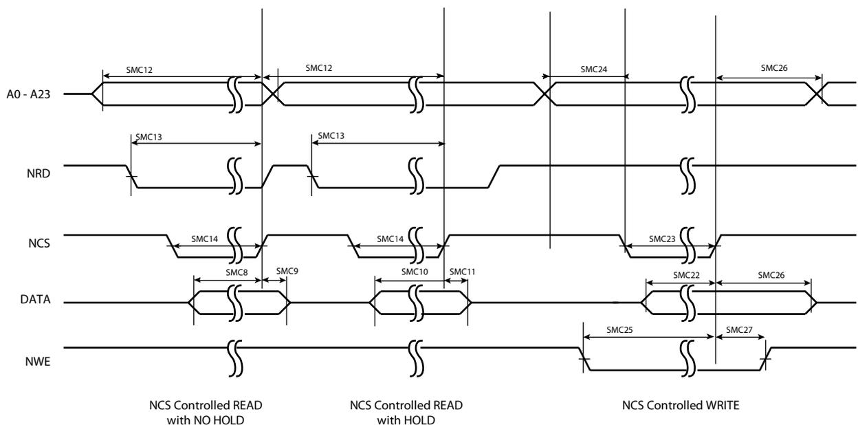
**Figure 13-20. SMC Timings - NRD Controlled Read and NWE Controlled Write**
