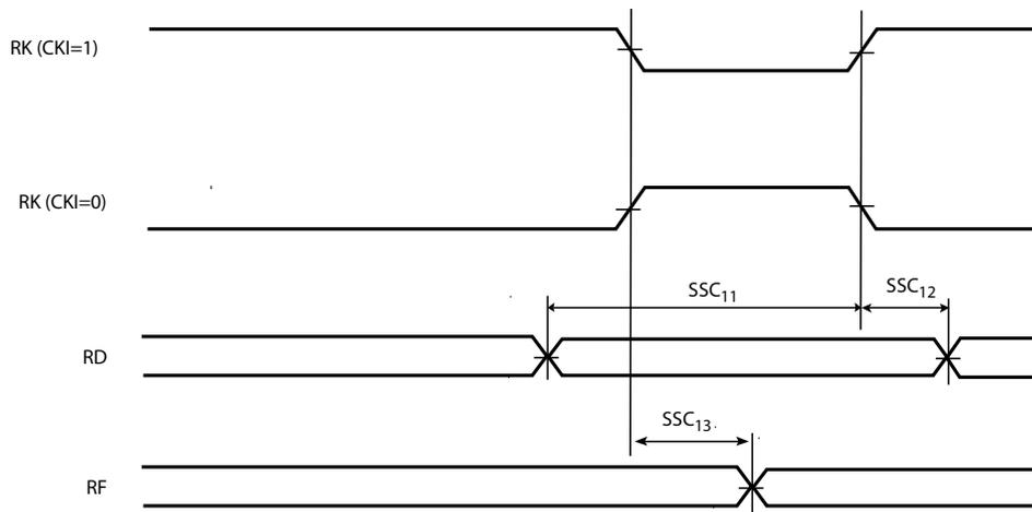
Figure 13-17. SSC Receiver, RK as output and RF as input
