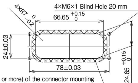
Finish the edge (3.5 mm or more) of the connector mounting hole where waterproof sealant will make contact (▨ area) with the surface roughness of  $\sqrt{Rz3.2}$
