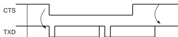
Figure 44-28: Transmitter Behavior when Operating with Hardware Handshaking
