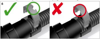
Orientate the oval retaining clip as illustrated and locate it in the slot as shown.
