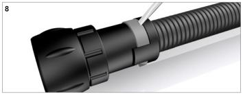
To release the locking mechanism, use a screwdriver.
