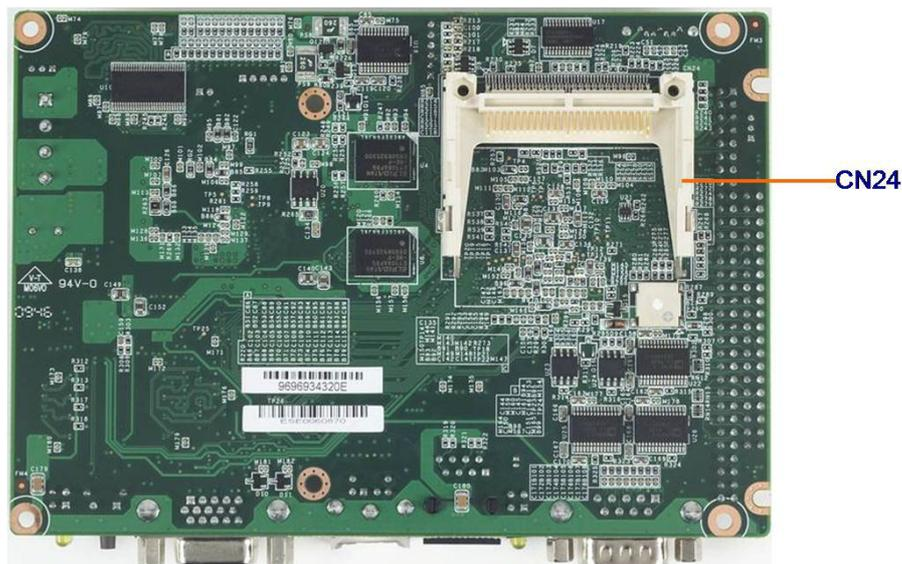
Figure 2.2 Jumper and Connector layout (Solder side)
