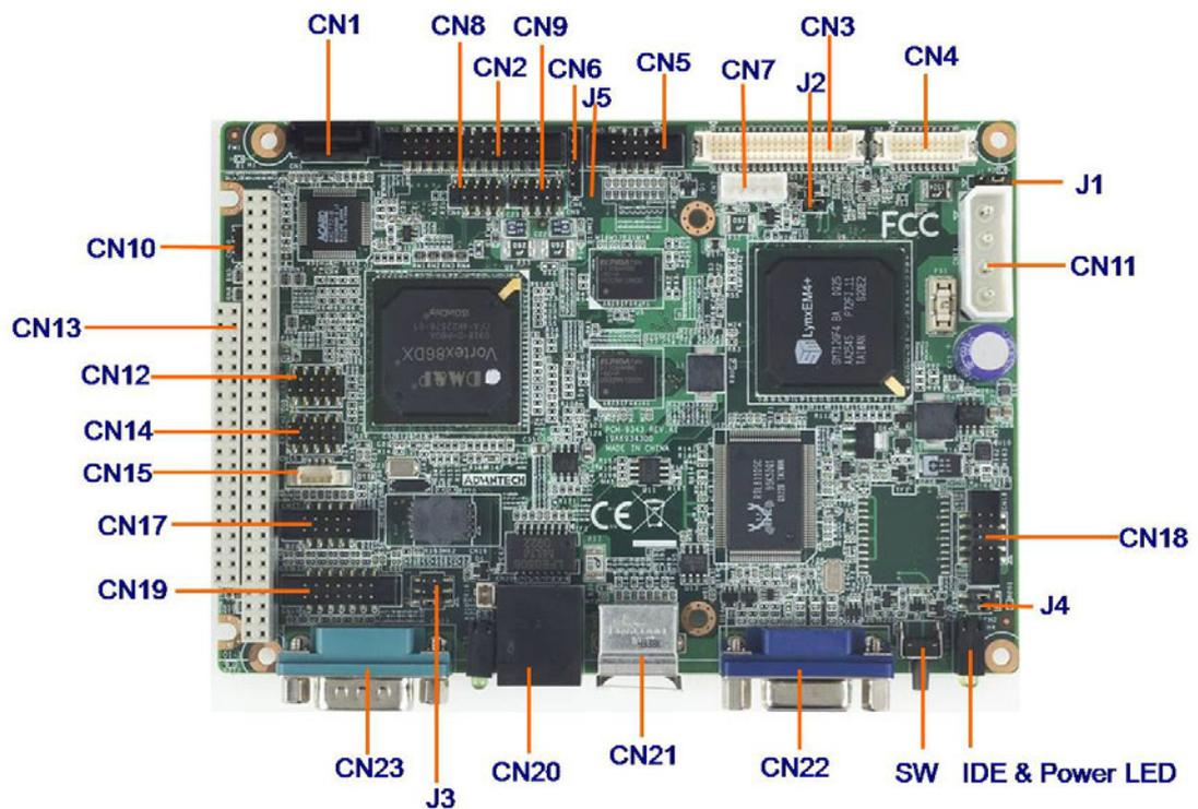
Figure 2.1 Jumper and Connector layout (Component side)
