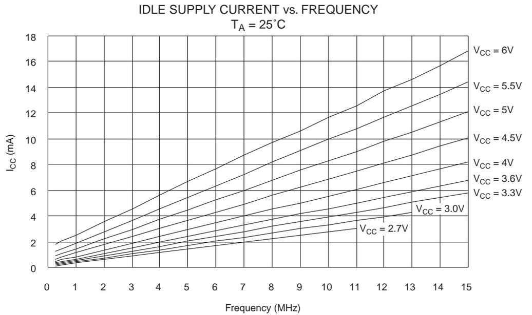
Figure 73. Idle Supply Current vs.  $V_{CC}$
