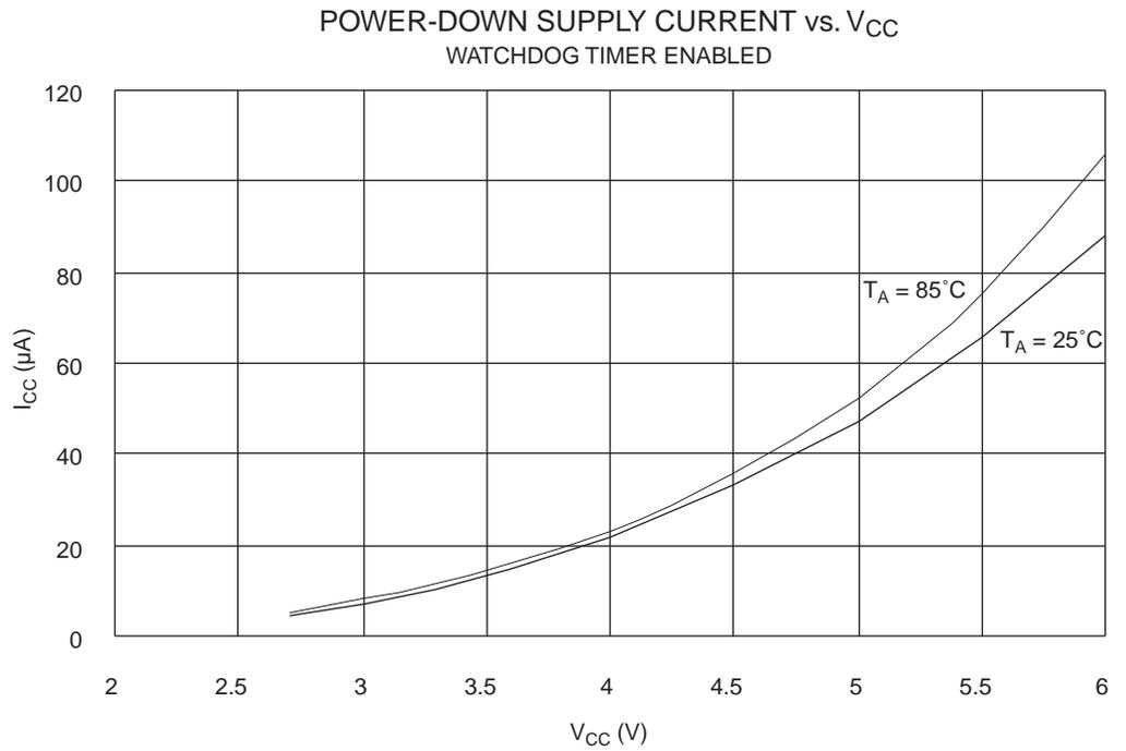
**Figure 76.** Power-down Supply Current vs.  $V_{CC}$
