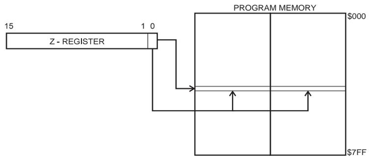
Constant byte address is specified by the Z-register contents. The 15 MSBs select word address (0 - 2K), the LSB selects Low Byte if cleared (LSB = 0) or High Byte if set (LSB = 1).
