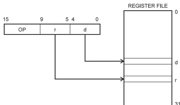
Operands are contained in registers r (Rr) and d (Rd). The result is stored in register d (Rd).
