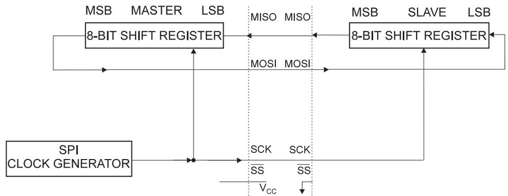
The system is single buffered in the transmit direction and double buffered in the receive direction. This means that bytes to be transmitted cannot be written to the SPI Data Register before the entire shift cycle is completed. When receiving data, however, a received byte must be read from the SPI Data Register before the next byte has been completely shifted in. Otherwise, the first byte is lost.
