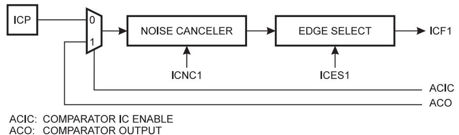
If the Noise Canceler function is enabled, the actual trigger condition for the capture event is monitored over four samples, and all four must be equal to activate the Capture Flag. The input pin signal is sampled at XTAL clock frequency.
