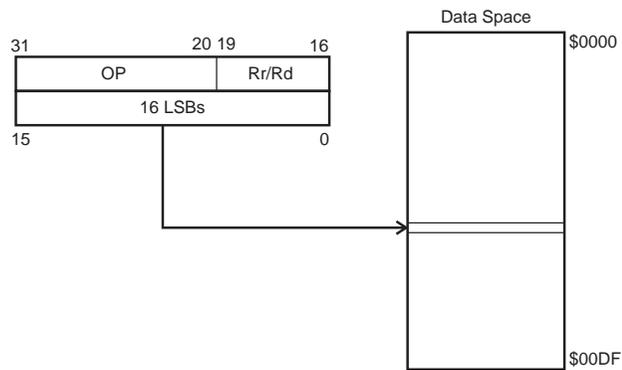
A 16-bit data address is contained in the 16 LSBs of a two-word instruction. Rd/Rr specify the destination or source register.
