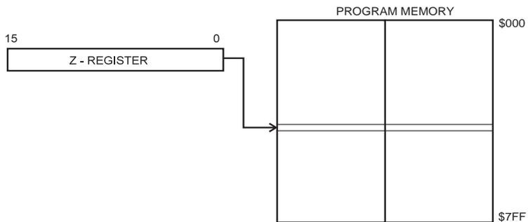
Program execution continues at address contained by the Z-register (i.e., the PC is loaded with the contents of the Z-register).
