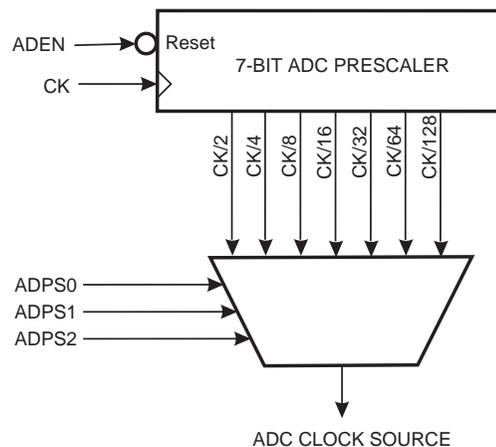
The ADC contains a prescaler, which divides the system clock to an acceptable ADC clock frequency. The ADC accepts input clock frequencies in the range 50 - 200 kHz. Applying a higher input frequency will result in a poorer accuracy (see “ADC Characteristics” on page 71).
