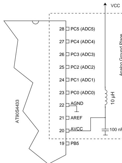
Note that since AVCC feeds the Port C output drivers, the RC network shown should not be employed if any Port C serve as outputs.
