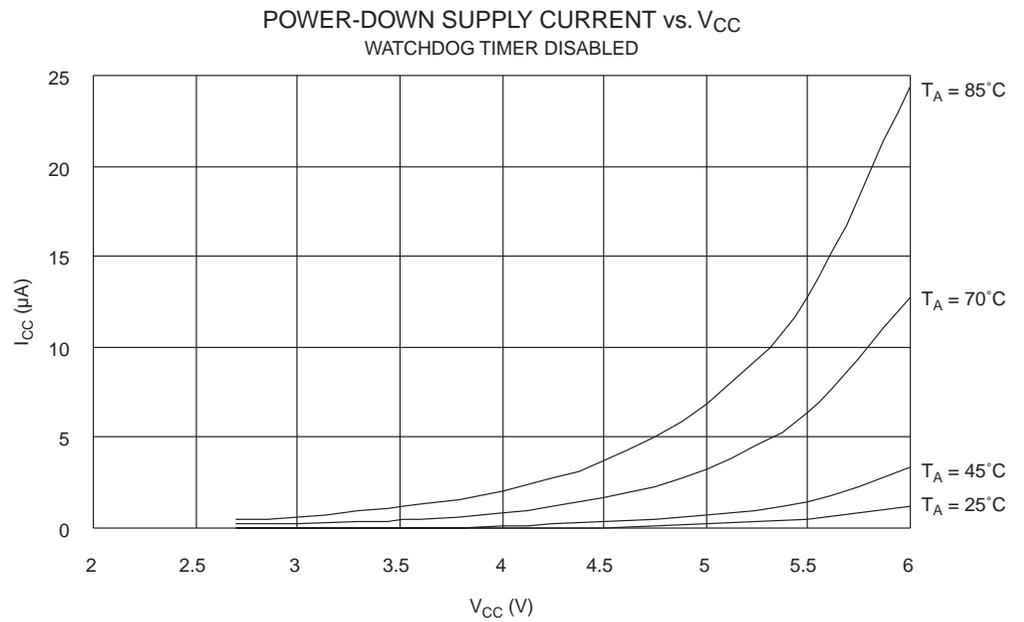
**Figure 75.** Power-down Supply Current vs.  $V_{CC}$
