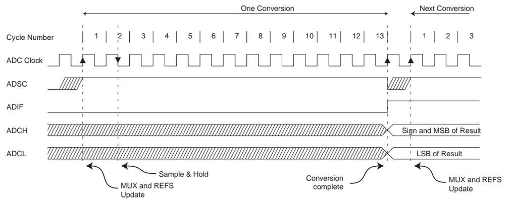
**Figure 48.** ADC Timing Diagram, Free Run Conversion
