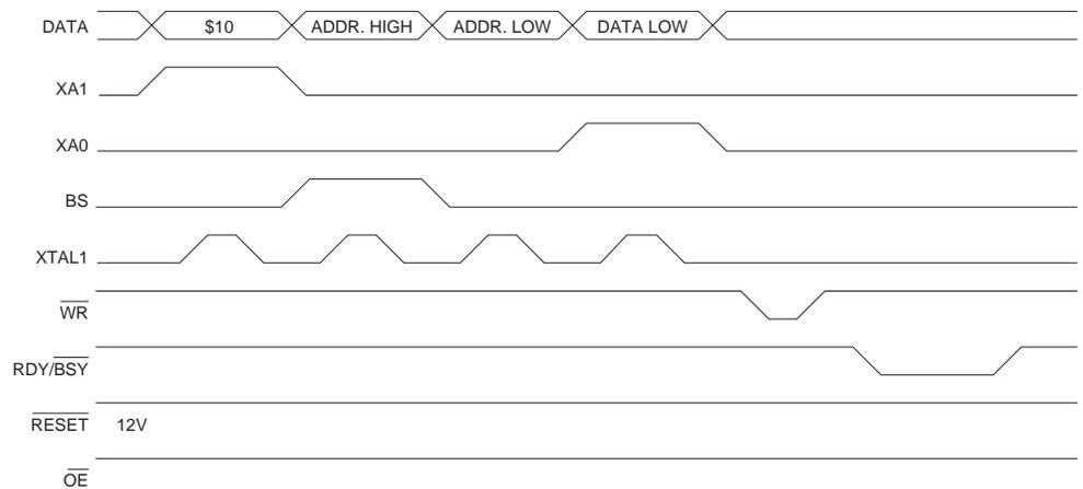
**Figure 64.** Programming the Flash Waveforms (Continued)
