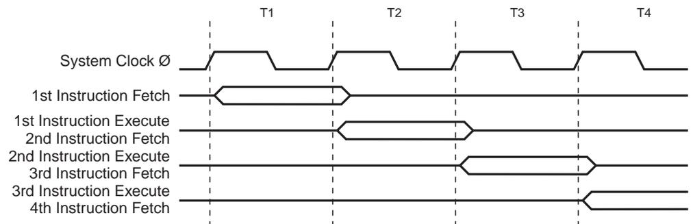
Figure 22 shows the internal timing concept for the Register File. In a single clock cycle an ALU operation using two register operands is executed and the result is stored back to the destination register.
