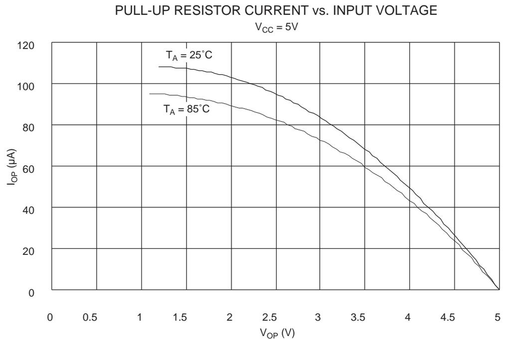
**Figure 83.** Pull-up Resistor Current vs. Input Voltage
