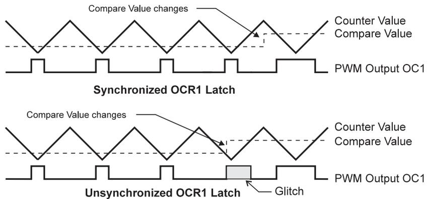
During the time between the write and the latch operation, a read from OCR1 will read the contents of the temporary location. This means that the most recently written value always will read out of OCR1.
