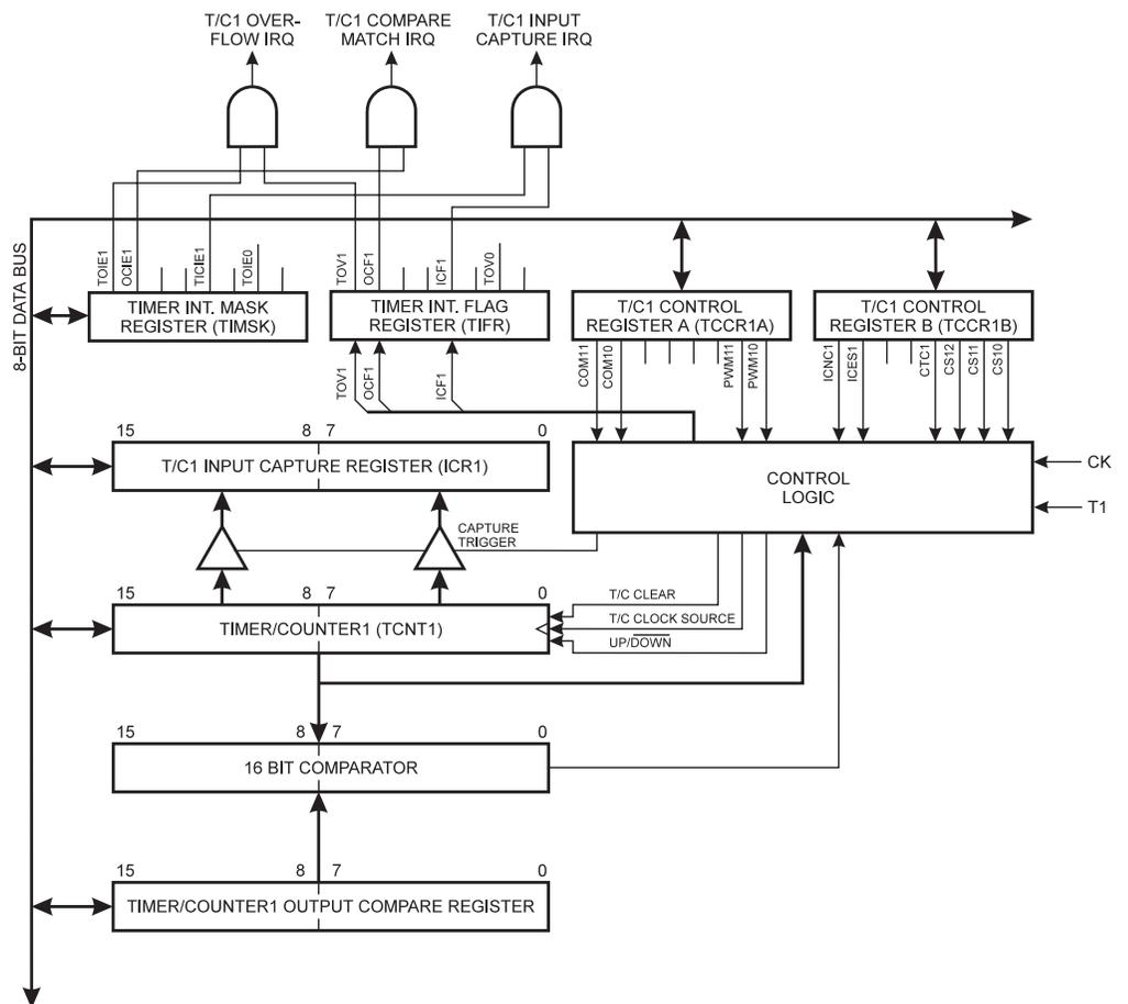
The 16-bit Timer/Counter1 can select clock source from CK, prescaled CK or an external pin. In addition, it can be stopped as described in the specification for the Timer/Counter1 Control Register (TCCR1A). The different Status Flags (Overflow, Compare Match and Capture Event) and control signals are found in the Timer/Counter
