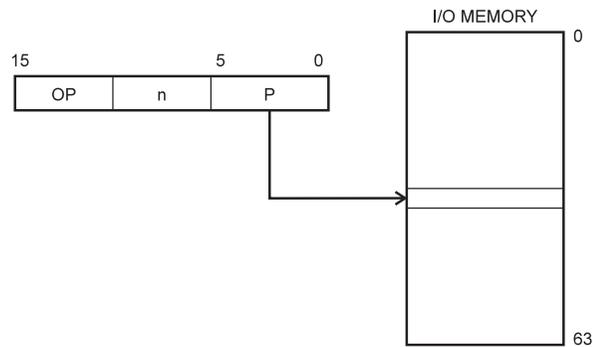
Operand address is contained in six bits of the instruction word. n is the destination or source register address.
