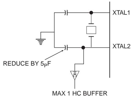
**Figure 4.** External Clock Drive Configuration
