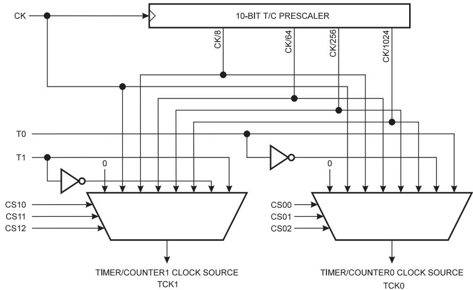
For Timer/Counters0 and 1, the four different prescaled selections are CK/8, CK/64, CK/256, and CK/1024, where CK is the Oscillator clock. For the two Timer/Counters0 and 1, external source and stop can also be selected as clock sources.
