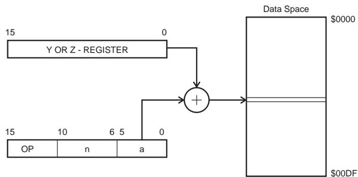
Operand address is the result of the Y- or Z-register contents added to the address contained in six bits of the instruction word.
