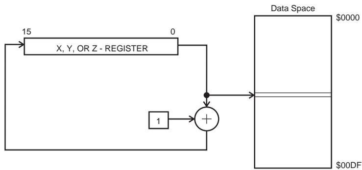
The X-, Y-, or the Z-register is incremented after the operation. Operand address is the content of the X-, Y-, or the Z-register prior to incrementing.
