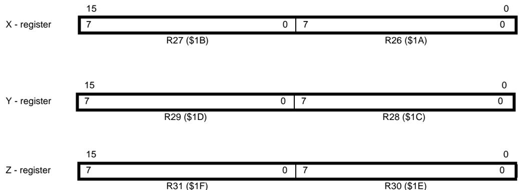
In the different addressing modes, these address registers have functions as fixed displacement, automatic increment and decrement (see the descriptions for the different instructions).
