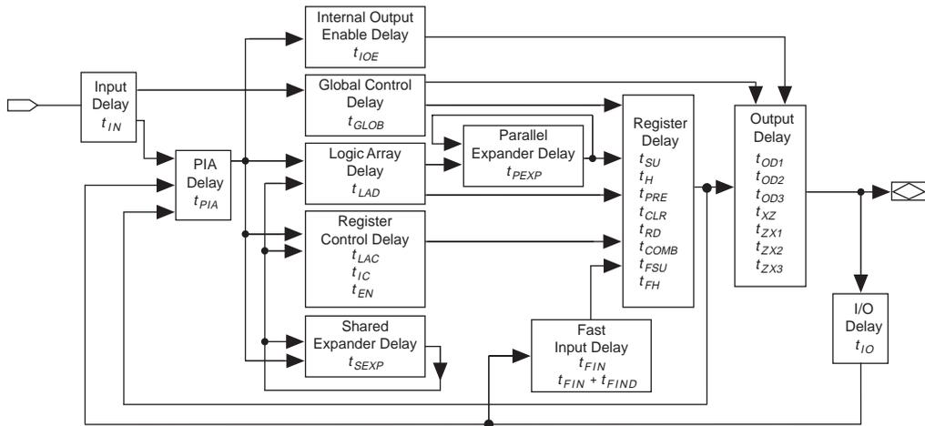
The timing characteristics of any signal path can be derived from the timing model and parameters of a particular device. External timing parameters, which represent pin-to-pin timing delays, can be calculated as the sum of internal parameters. [Figure 14](#) shows the timing relationship between internal and external delay parameters.
