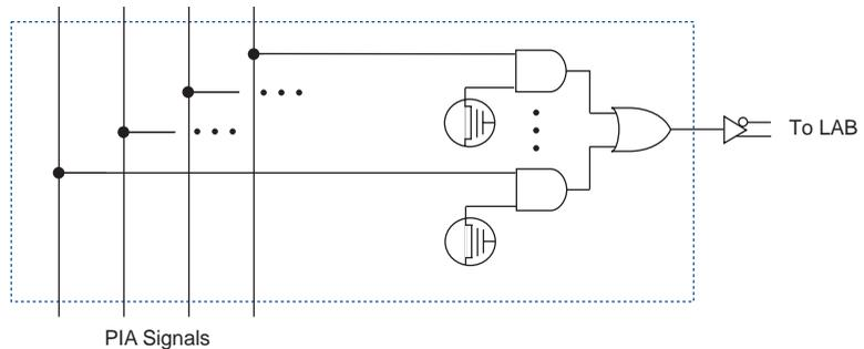
While the routing delays of channel-based routing schemes in masked or field-programmable gate arrays (FPGAs) are cumulative, variable, and path-dependent, the MAX 7000B PIA has a predictable delay. The PIA makes a design's timing performance easy to predict.
