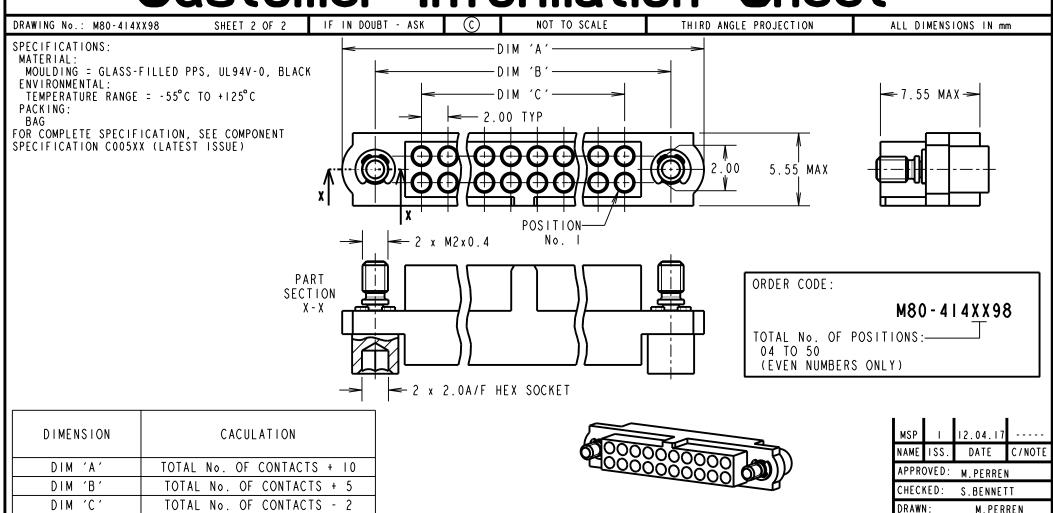
M80-4142098 DIM 'A' = 30.00mm, DIM 'B' = 25.00mm
